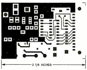
Fig. 4. The component side of the author's double-sided layout is shown here full size. You can fabricate your own board using the artwork provided, or you can purchase a prefabricated board from the source mentioned in the Parts List.
