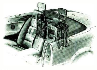
In BMW's Rollover Protection System, if a sensor detects an impending rollover, rollbars located in the seats are released and extend 10 inches above the headrests.
