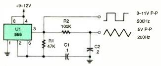
Fig. 1. This triangle waveform generator was designed to give good results with as few parts as possible.
