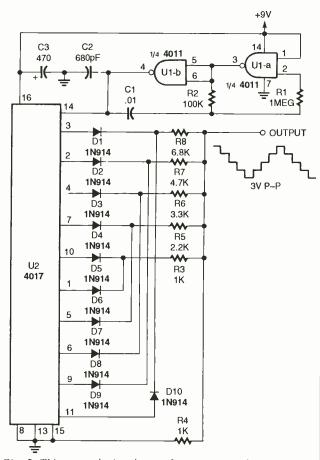
Fig. 5. This stepped triangle waveform generator is an experimenter's delight as different output arrangements can produce a variety of waveforms.
