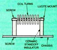
Fig. 3. This is an example mounting for Barker and Williamson Pi-Dux coils used in VFO circuits. Note how stable it looks.
