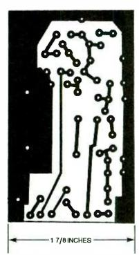
Fig. 3. The author's prototype of the Gate-Dip Meter was assembled on a small printed-circuit board, measuring about 17/8 × 34/6 inches.
