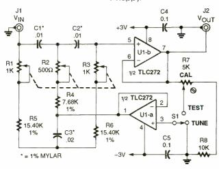
Fig. 1. Need a nice THD analyzer but haven't got thousands of dollars to spend? Try adding this to your multimeter and pocket the difference.
