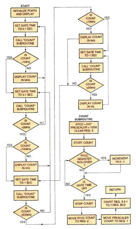
Fig. 2. This flowchart shows the operating program stored in the microcontroller (U1). Note the conditions that change the gate time and/or the suffix (Hz. kHz. or MHz).
