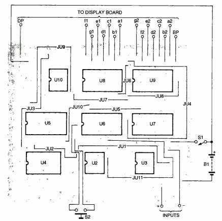
Fig. 5. The locations of the numerous jumpers and the connections to the off-board components are shown here. The outlines of the DIP IC's are also shown as reference points to aid the builder.
