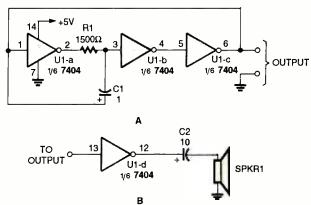
Fig. 3. Thought TTL-based audio oscillators would be impossible to build? Try the one shown in A, and if you need an annunciator. connect the circuit in B to its output.
