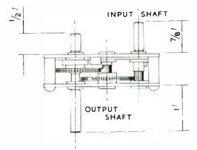
The Jackson Brothers G-10 gear box/drive mechanism is available in three models with different turns ratios.
