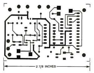
Fig. 3. The author's prototype was assembled on a double-sided printed circuit board, measuring about 21/8 by 115/16 inches. Shown here is a full-size template of the foil side of the board.
