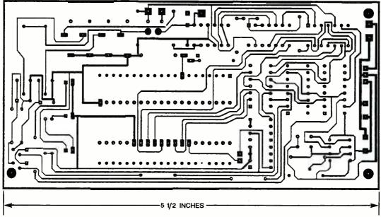
Fig. 2. The Auto-Ranging Digital Capacitance Meter was assembled on a double-sided, printed-circuit board measuring about 5½ by 2½/6 inches. A full-size template of the foil side of the board is shown here.
