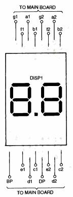
Fig. 7. Here is the parts-placement pattern for the LCD-display board.
