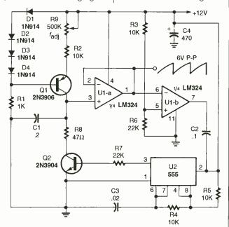
Fig. 4. Offering a different approach to improved linearity, this sawtooth generator is reset at the end of each cycle, resulting in a constant peak-to-peak output throughout its frequency range.
