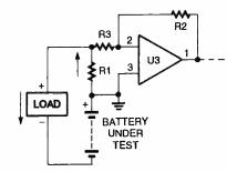
Fig. 9. This diagram shows how a load and a power source (the battery under test) are connected to the meter.
