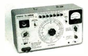
The Sprague TO-4 as received. Its physical condition was good, except for the pushed-in glass window on the meter at the upper right.
