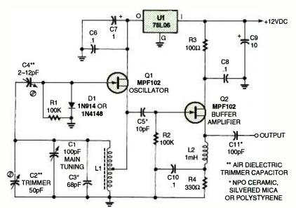
Fig. 4. This typical HF VFO circuit has several stability-enhancing features, including well-chosen capacitor types.
