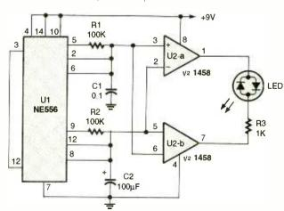
Fig. 3. If you want a really unusual display, check out this LED circuit which slowly shifts between three colors automatically.
