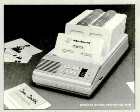
card is pulled from the card file and inserted in the reader slot. Then the DIAL button is pressed. The Phonedex automatically dials the correct number.
