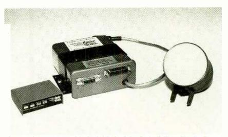
These are the components of the Rashid Radar Safety Brake Collision Warning System. Shown are the dashboard monitor (left), electronic signal processor (center), and microwave radar antenna (right).
