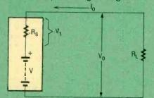
Fig. 1. The main cause of voltage changes with variations in load current is the internal resistance of the DC power supply. The voltage drop across it  $(V_1)$ varies with load current.
