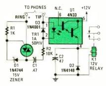
Fig. 1. The Phone-Flasher is a rather simple circuit (built around a triac, an optoisolator/coupler, and a relay) designed to give a visual indication of an incoming call.
