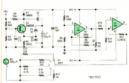
Fig. 2. This Metal-Detector circuit, with Ql serving as the heart of a Colpitts oscillator, is easy to build and contains no exotic parts.
