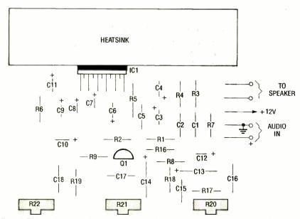
Fig. 4. This is the parts-placement diagram for the 30-watt amplifier. Solder the parts in the order that they're described in the instructions.
