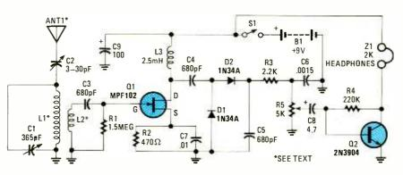
Fig. 1. The Tunable/Amplified Receiver goes two steps beyond the conventional crystal radio by adding a tuned RF amplifier and an audio-amplifier stage.
