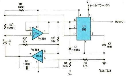
Fig. 4. This circuit multiplies the timing capacitance rather that the timing resistance. Note that in the circuit, the timing capacitance (C3) is not tied to ground, but instead to the output of the second op-amp (Ul-b), which functions as a capacitance multiplier.
