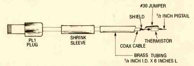
Fig. 4. A negative temperature coefficient thermistor is used as a temperature sensor. It is mounted in a temperature probe using the technique illustrated above.
