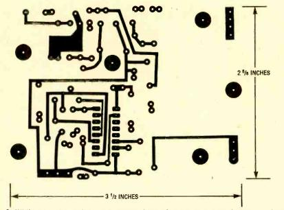
Fig. 2. While any construction technique can be used, the author elected to use a printedcircuit board. If you choose to do the same, here's a PC pattern that you can use.
