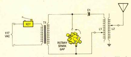
Fig. 3. Still another form of spark-gap transmitter was the rotary spark gap. Although conceptually similar to the fixed spark gap, an electrical motor was used to spin a rotor/ electrode half of the spark gap.
