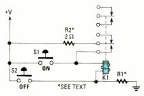
Fig. 8. The Missile-Controller, to put it quite simply, is a double-pole, doublethrow relay wired for latching operation.
