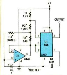
Fig. 3. In this circuit, the op-amp is used as a buffer stage for the timing network, while additional circuitry effectively multiplies the values of the timing components.
