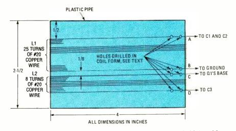
Fig. 2. Inductors L1 and L2 in the Tunable/Amplified Receiver are easily fabricated from a 21/2 length of 4-inch diameter plastic pipe (which is used as the coil form) and 22-gauge enamel-coated wire (25 turns for L1 and 8 turns for L2).
