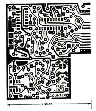
Fig. 2. The Budget Frequency/Events Counter was built on a printed- circuit board; shown here is a template for that board.
