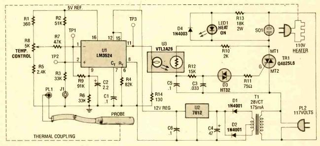
Fig. 1. The heart of the Precision Temperature Controller is UI, an LM3524 pulse-width modulator. That IC is normally used in switching power supplies, but is versatile enough that it can be used in many other applications, including this one.
