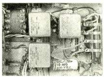
Here's a look beneath the power-supply chassis. The large tubular capacitor and the three big square units are bypasses. A wire-wound bleeder/voltage-divider resistor is at the right.
