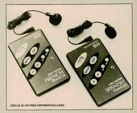
in conjunction with a small LCD display that shows a number between 1 and 301 corresponding to a phrase in the little softcover phrasebook. Finally, two other membrane switches provide single-step, and fast-forward and -reverse, functions to get you quickly to the number of the phrase you need.
