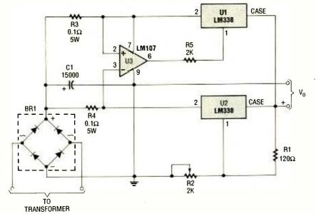
Fig. 8. This is a variable-voltage, 10-ampere DC power supply. The operation of the two LM338's is controled by the op-amp to ensure that they each work equally as hard.
