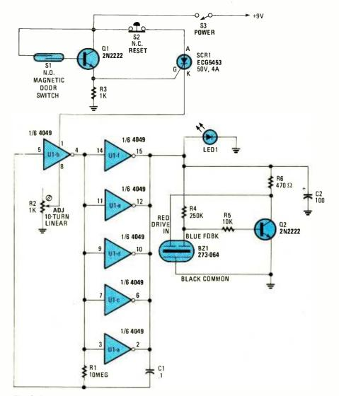
Fig. 9. In the Door Monitor circuit, one gate from a 4049 hex inverter is configured as an astable multivibrator, while the other gates in that package are paralleled to provide additional drive current to the output stages.
