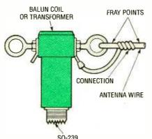
Fig. 1. Dipole antennas often use either a molded, center insulator or balun coil at their feedpoints.
