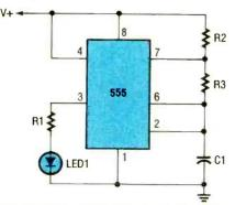
Fig. 1. When operated in the astable mode, the voltage on Cl oscillates between  $\frac{1}{3}V_{CC}$ (the internally set upper threshold level) and  $\frac{2}{3}V_{CC}$  (the internally set lower threshold level) as long as power is applied to the circuit. combination—its upper frequency limit for reliable operation is about 100 kHz.
