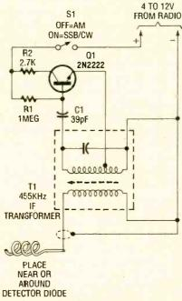
Fig. 1. The CW/SSB Adapter is made up of very few components, and none of them are critical.
