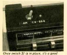
idea to label the switch positions on the outside of the receiver's enclosure. Removing power from the circuit, by flipping SI to the AM position, effectively disconnects the Adapter from the receiver's detector diode.
