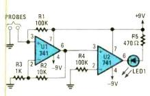
Fig. 5. The Smart Continuity Tester, as its name implies, will not only tell you when you have continuity, but will also tell you if you're reading even a low resistance through a component as well.
