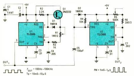
Fig. 4. The CMOS Square-wave/Pulse Generator is essentially two 555 oscillator/timer IC's (one gating the other). The output frequency of the first 555 and the output pulse rate of the second 555 are variable via R1 and R5, respectively.
