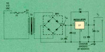
Fig. 2. This is a standard circuit for using a three-terminal voltage regulator. Note that DI will dissipate the charge on C4 when the supply is shut down.
