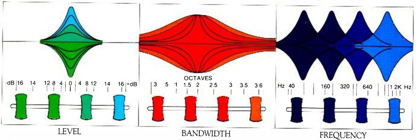
With the graphic equalizer, you have a limited number of chances to correct an infinite number of potential problems in a recording or listening environment. You're dealing with fixed bandwidths and fixed frequencies. You can only increase or decrease the level. When boosting or cutting frequencies,
