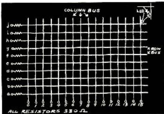
Fig. A. 10 x 16 160-element LED display.
