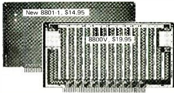
**S100 CARDS—100 PLUG CONTACTS**—Convenient universal tinned pads and bus lines. For interface, memory expansion, breadboarding. Mount almost anything anywhere on card.
