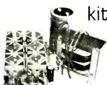
12A @ 50% duty cycle, foldback current limiting, over-voltage protection, many more features. Does not include case.
