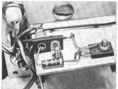
Fig. 4. Electronic components are wired together on L bracket secured to front plate of the box.
