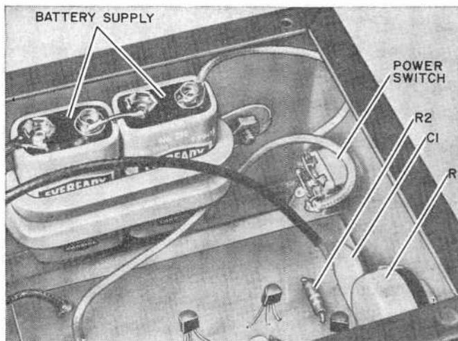
Fig. 3. Two 9-volt transistor batteries, connected in series, can be mounted to box with U brackets or small drawer pull.
