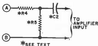
Fig. 4. Optional add-on allows Bug-Shoo to be used with amplifier for larger area coverage. Points A and B connect to respective points in main schematic diagram.
