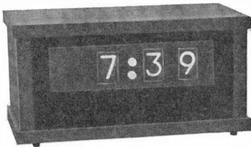
counter chain which uses the 60-Hz line as a reference with decimal and divide-by-six counters feeding BCD-to-decimal decoders. If I were to build another one right now, I could do it for a little under \$90.
