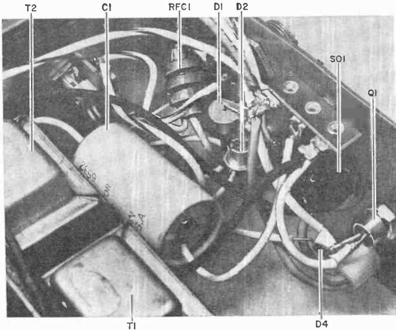
Fig. 2. Component mounting is best accomplished if ends of chassis are bent slightly outward during machining and chassis wiring.
