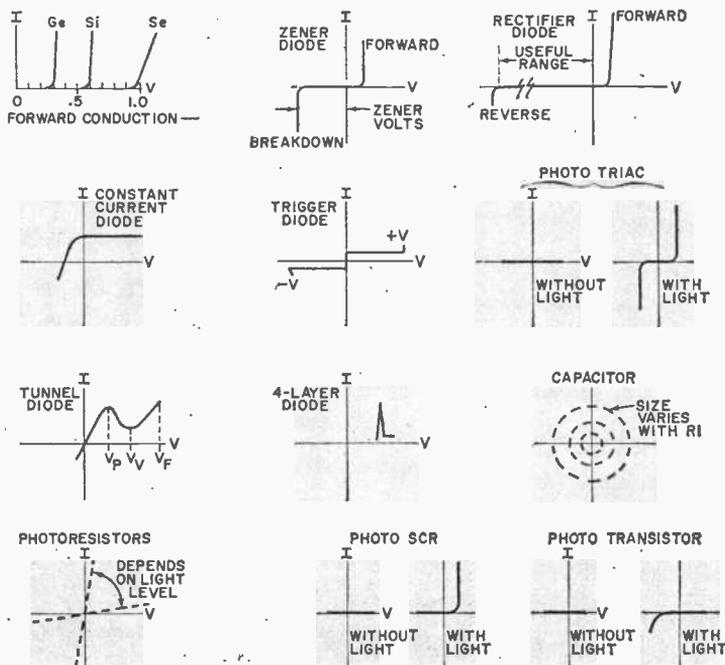
Fig. 2. Typical curves as seen on the scope. For other semiconductors, consult the applicable manual. For exact values, you must use a calibrated d.c. scope.
