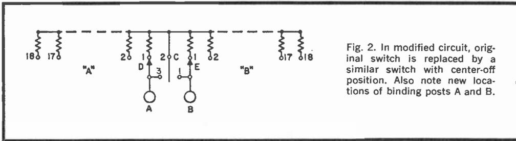
Fig. 2. In modified circuit, original switch is replaced by a similar switch with center-off position. Also note new locations of binding posts A and B.
