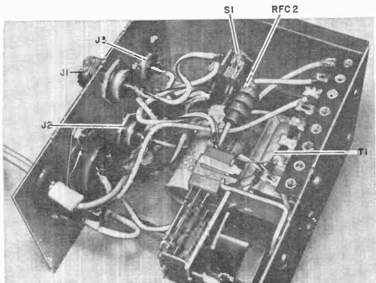
The current threshold detector circuit made up of *D1*, *D2*, and *T1* controls the power delivered to the solenoid of *K1*. The voltage drop across monitoring diodes *D1* and *D2* is on the order of 1.5 volts peak-to-peak and is independent of the power required by the transceiver. The square-wave voltage drop across the diode pair is coupled through transformer *T1* to silicon controlled rectifier *SCR1*.
