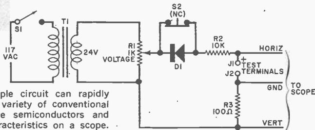
Fig. 1. This simple circuit can rapidly sort out a great variety of conventional and light-sensitive semiconductors and display their characteristics on a scope.
