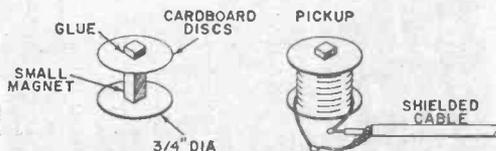
Bond cardboard discs to magnet with epoxy cement. Tape cable to pickup coil winding.
