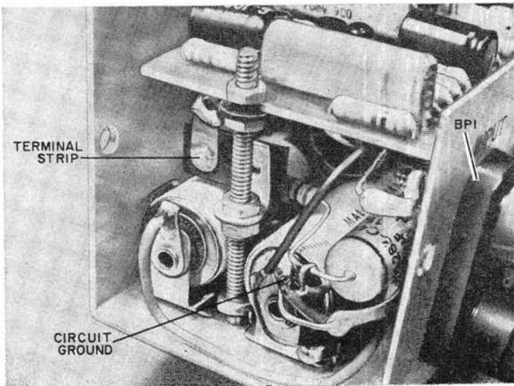
grounds should be made to the same grounded battery clip where the negative end of *C15* is connected.
