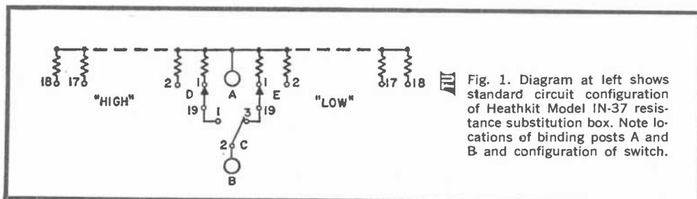
Fig. 1. Diagram at left shows standard circuit configuration of Heathkit Model IN-37 resistance substitution box. Note locations of binding posts A and B and configuration of switch.
