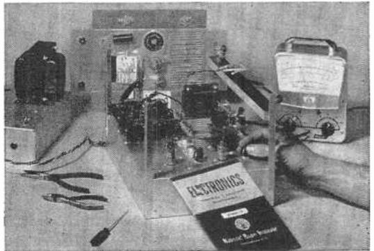
**first** to give you completely specialized training kits engineered for business, industrial and military Electronics. Shown above is your own training center in solid state motor control and analog computer servo-mechanisms. Telemetering circuits, solid-state multi-vibrators, and problem-solving digital computer circuits are also included in your course.
