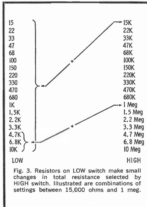
Fig. 3. Resistors on LOW switch make small changes in total resistance selected by HIGH switch. Illustrated are combinations of settings between 15,000 ohms and 1 meg.
