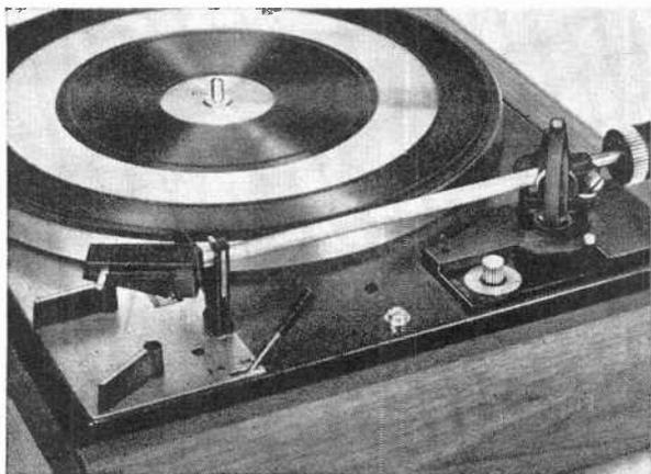
Special features of Dual 1219 include disc diameter selector and damped up/down cueing levers (far left foreground) and anti-skate and tonearm leveler controls (near left foreground). Cast platter is a full 12" in diameter and comes with milled neoprene ribbed disc mat.
