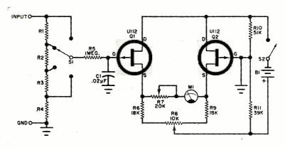
Fig. 11. This FET voltmeter, featuring a matched pair of Siliconix U112 FET's in a differential amplifier arrangement, has a sensitivity of 0.5-1.0 volt full scale.
