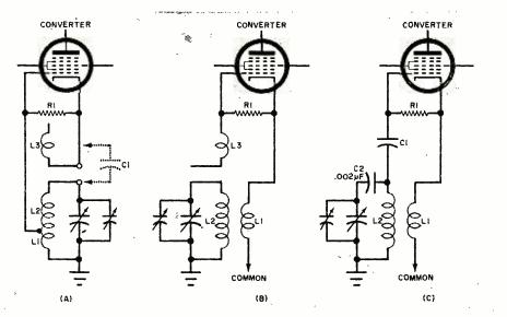
Fig. 1. Broadcast receiver oscillator circuit configurations include (a) tapped coil and (b) standard coil with "gimmick" winding. In converted oscillator (c), L3 is replaced by C1, and padder C2 is added.
