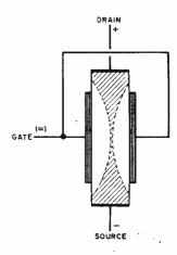
Fig. 4. Diffusion of p-type regions into n-type substrate provides a means of controlling the current flow between source and drain electrodes.
