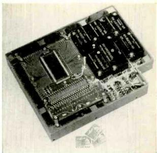
LITTLE GUY WITH A B-I-G JOB—A tiny memory unit built by Electronic Memories is hardly larger than 5 packs of cigarettes, yet it contains all the information needed to put Lunar Orbiter B into orbit around the moon, aim the camera at the moon's surface and start them rolling. During Lunar Orbiter B's shuttle to the moon, the memory unit has the jobs of extending the antennas and solar panels, controlling the propulsion and attitude of the spacecraft, and starting the scientific experiments.
