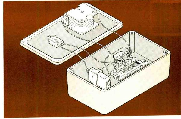
Housed in a plastic instrument case, the AMLIGNER can be assembled and wired in a matter of minutes. When wiring components to the terminal strip, be sure to observe polarity orientation of diode D1.
