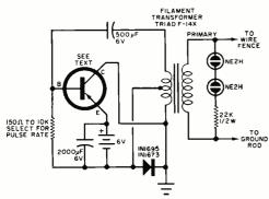
Fig. 1. Simple electric fence shocker.
