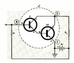
Fig. 3. Packaged in a single case, this Darlington pair can be treated as a single transistor by making the input and output connections as shown.
