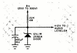
Fig. 6. This simple voltage divider can be used in a tube-type transceiver to obtain a 9-12 volt regulated output for operating the Audio Leveler.
