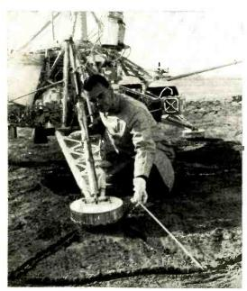
SOFT LANDING VERIFIED—With data taken by electronic strain gauges made by Baldwin-Lima-Hamilton Corp., Surveyor I's soft landing on the moon was verified and radioed back to earth. The strain gauges also provided important data on the bearing strength of the lunar surface.
