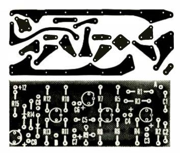
Fig. 3. Actual-size photo shows foil side of printed circuit board (upper left); component side of board is below it. Observe polarity markings when installing diodes and electrolytic capacitors. Also, position the transistors as shown.
