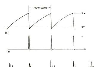
Fig. 2. Voltage and current waveforms include: (a) sawtooth voltage across C1; (b) a current pulse through D1; and (c) a ringing waveform across C2.
