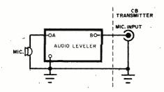
Fig. 5. Terminal A goes to the microphone and terminal B connects to the MIC input on the transmitter. The unit is grounded to the transmitter.
