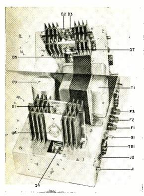
Fig. 5. Mirror standing on top of T1 shows D2 and D3 mounted on the back of the heat sink holding Q6. Other heat sink holds D1 and Q7. Note the cutouts in chassis to allow heat from Q4 and Q5 to escape.
