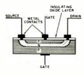
Fig. 8. This junction FET features single-ended construction. Here, an n-type channel is formed on one side only of a p-type substrate by photo-masking, etching, and impurity diffusion processes. The surface is covered with an insulating oxide layer through which holes are cut for electrode connections.
