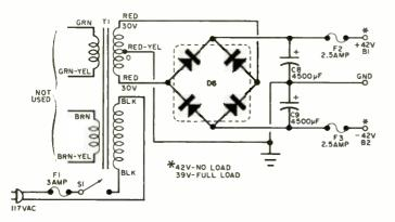
Fig. 2. Positive and negative supply voltages are balanced with respect to ground through a 60-volt center-tapped winding. Try using 2-ampere, fast-blow fuses for F2 and F3. If they don't stand up, use the 2½-ampere size shown here.
