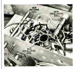
Under-the-chassis view of a converted marine band receiver shows location of the antenna and oscillator coils. The old oscillator coil is made inoperative but is not physically removed from the circuit.
