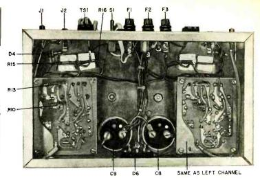
The chassis improves shielding of the input stages and minimizes extraneous hum and noise pickup. Don't forget the rectangular cutouts on top of the chassis to permit air circulation around driver transistors Q4 and Q5.
