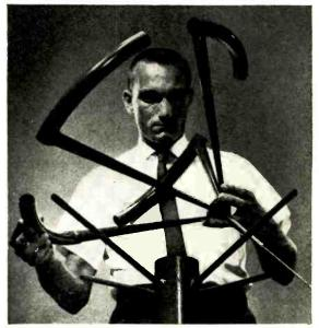
"CIRCULAR POLARIZED LOOP VEE"—A new type of space age antenna (photo above) has been designed and built for the U.S. Air Force by Electronic Communications, Inc. Together with its associated satellite communications terminal equipment, this odd-shaped antenna will be used in airborne applications. It radiates up to 1000 watts of power in an omnidirectional pattern to provide optimum near-horizon communications coverage.
