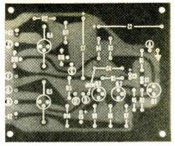
Fig. 4. Component layout on printed circuit board. The jumper lead (JUM) connecting C4 to Q3's collector can be eliminated by extending the foil conductor from C4 around the left end of resistor R5.
