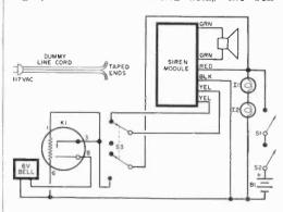
sounds off, causing the "victim" to panic and throw the switch again. This, of course, starts the siren up a second time. The relay, *K1*, is an Amperite 6N05T. A 6-volt lantern bat-
