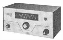
dial, it comes in two models—one covering 152-175 mc., the other 30-50 mc. The "FM Alert" utilizes a quadrature detector and high-gain i.f. to provide clean, quiet reception over a wide range of signal strengths and modulation levels. Sensitivity is 3  $\mu$ v. or less for squelch control and 10 db S/N. A separate matching speaker can be used either at the receiver or at a remote location.
