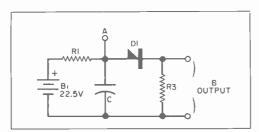
Fig. 1. Four-layer diode conducts when the capacitor charges up to about 12 volts, and stays "on" as long as there is more than 1 ma. of current flow.
