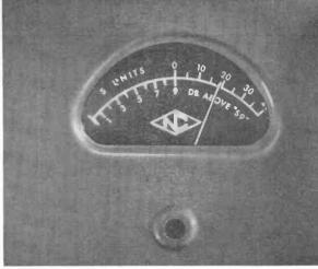
be inconsistent is the fact that receiver manufacturers do not have a common calibration standard. Also, each manufacturer has his own calibration method. Plus, variations in components may cause S-meters in two receivers of the same make and model to perform differently.
