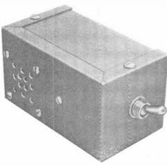
Completed unit should be located within easy reach of the driver. Only two wires connect the alarm to the lights and ignition system. Ground the case,
