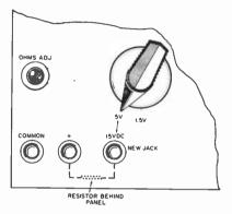
to "5 V," and the d.c. test lead in the new jack, a full-scale deflection will indicate 15 volts. With the d.c. scale essentially linear, a mid-scale reading will indicate 7.5 volts. Inscribe "15 VDC" on the front panel directly over the new jack, using white India ink or
