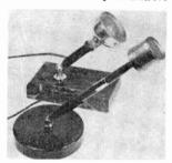
side of the case for the mike cable to pass through. If you decide to mount the mike in the pen holder, locate the hole in any suitable position. One thing you won't be able to do with the pen when you're through is write.
