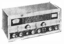
the entire tuning range. A front panel control permits ready selection of either upper or lower sideband for simplified tuning of the SSB signals. In addition to having a circular main tuning dial and a slide rule electrical bandspread dial, the SX-130 features both crystal filtration and crystal-controlled selectivity. The 1650-kc. i.f. system insures excellent image rejection. Other features of the SX-130 include a built-in S-meter and a calibrated BFO.
