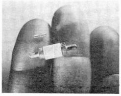
The relative size of two transit time devices being investigated at Bell Labs for use as microwave generators and amplifiers is shown above. The smaller device contains a tiny wafer of gallium arsenide. The larger device is used to house either a Read diode or a silicon pn junction diode.
