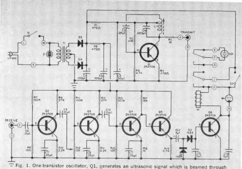
Fig. 1. One-transistor oscillator, Q1, generates an ultrasonic signal which is beamed through the air and back to the receiver, Q2 to Q6. Alarm sounds when beam is interrupted.
