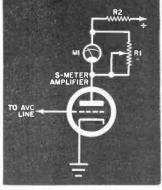
The only difference between these two S-meter circuits is. To make the meter read forward-increase of the position of the meter. In both cases the meter reads in strength means more current—the meter backward-increasing signal strength means less current, circuit must be revised as shown here.
