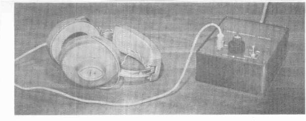
CERTAIN solid-state hi-fi/stereo amplifiers require special consideration when stereo headphones are to be used. If you own one of these amplifiers, here is "how-to-build-it" information on a universal speaker/headphone control unit—which, incidentally, can also be employed with any conventional tube-type stereo amplifier. With this control unit, you can remotely select speaker or headphone operation—and adjust headphone volume level—without leaving your easy chair.
