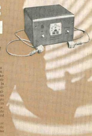
same chassis that detects this "sound." The "sound" is a 25-kc, note which is about 10 kc. above most people's hearing range. In many respects the system is similar to the common light source and photocell alarm system, but with several
