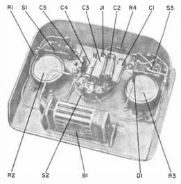
Only electrical connection to the chassis is at J1. The unused side of S2 conveniently serves as a terminal strip for the negative capacitor leads,
