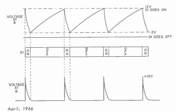
Fig. 2. Typical capacitor chargedischarge waveform is present at point "A" in Fig. 1. At output "B," the rise time is so fast that you'll need a fairly good scope to see it. When the diode is "off," the capacitor has a chance to build up a charge until it is large enough to trigger the diode into conduction. Current flow through the diode is relatively so very large that the capacitor discharges and cannot take on a new charge until the diode stops conducting.
