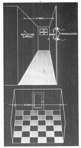
Fig. 6. To cover a narrow passageway, both transducers can be mounted on the same wall; for a wider area, up to 50', the direct-path technique is used.
