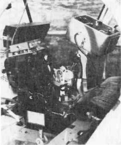
The Hydrodist, the black rectangular box at left, transmits microwaves to ground units. Distance is determined by the time it takes for the signals to make the round trip back.
