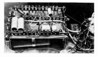
der cars and has two ranges-0-1200 rpm and 0-6000 rpm. Both ranges work from a transistorized Schmidt trigger pulse counter and can be attached to conventional and most transistorized ignition systems.
