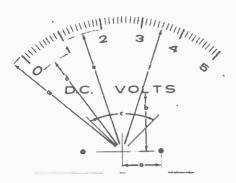
Fig. 1. Carefully measure dimensions "a" through "g" on original meter face and multiply by five. All measurements are in inches except the angle "c," which is measured in degrees with a protractor.
