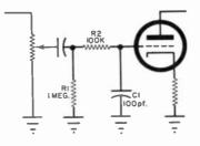
this type of interference is to reduce the value of the grid resistor (R1) in the first audio stage to 1 megohm, and install R2 and C1.
