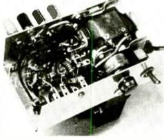
Adjustment. The output voltage of the supply may be set to any value between 150 and 250 volts with  $R_4$ . To avoid exceeding the dissipation rating of the 6JZ8, the current drawn from the supply should be limited to 40 ma. at 150 volts, and 60 ma. at 250 volts. With the transformer specified, about  $1\frac{1}{2}$  amperes may be drawn from the 6.3-volt terminals to operate the filaments of the tubes in another unit.
