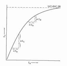
Fig. 6. Beta readings will vary as the slope angle of the response curve. Notice that for the same amount of change in base current, there is a smaller change in collector current as the curve flattens out and approaches saturation.
