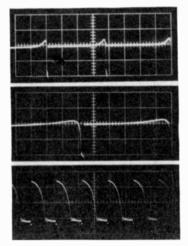
Waveforms (with R2 at 18,000 ohms) across lamp at .1, 1, and 30 cycles.
