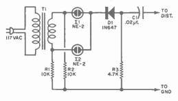
Low cost, easy-to-make tester calibrates tachometers under actual conditions without any other equipment
