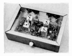
Fig. 7. A printed circuit board or any other standard wiring technique can be used. All components are mounted on one slde. Keep transistors about  $\frac{1}{4}$ " above the board, or install in sockets.
