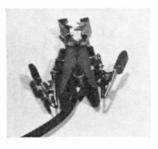
mission line can be connected to the small alligator clips. The extra set of clips can also be used as terminal points for stubs and other test leads even while the connector is clamped to a pair of terminals in the conventional manner.
