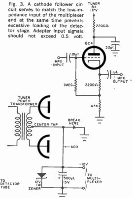
Fig. 4. Zener diode and filter capacitor added to the tuner's power supply eliminate need for an external power source for the multiplexer.
