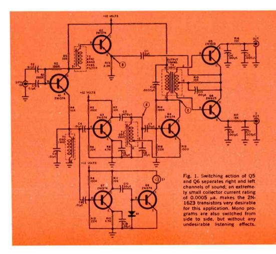
38-kc. rate. If this switching rate is precisely synchronized with the 19-kc. pilot signal of a stereo station, the left and right components of a stereo program are separated and recovered.
