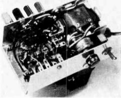
Adjustment. The output voltage of the supply may be set to any value between 150 and 250 volts with  $R_4$ . To avoid exceeding the dissipation rating of the 6JZ8, the current drawn from the supply should be limited to 40 ma. at 150 volts, and 60 ma. at 250 volts. With the transformer specified, about  $1\frac{1}{2}$  amperes may be drawn from the 6.3-volt terminals to operate the filaments of the tubes in another unit.
