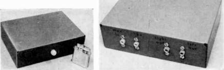
Fig. 5. Indicator lamp on front of cabinet goes on when stereo signals are tuned in. Electronic switching eliminates all external controls.
