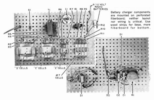
To eliminate shock hazard and make the charger convenient to use, build a base with some wood strips and another piece of fiberboard as a bottom cover. The parts can be held together with screws.
