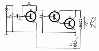
Fig. 3. General-purpose audio amplifier circuit submitted by reader Craig Ransom is good for intercom, signal tracer, etc.
