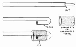
itself for a convenient but small distance. Although about  $\frac{1}{2}$ " is usually enough, different thicknesses or stiffnesses of wire will require different size folds to make a neat finish. (Be careful to ayoid accidental contact with metallic shielding when present.) Then slip a piece of spaghetti over the fold as shown in the drawing-it should fit snugly. *Phillip Baskin, K2RLB*
