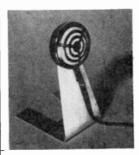
dimensions are not critical. Approximately 4" from the top, bend the metal to form about a 70-80° angle, adjusting the bend for best stability. Remove rough edges, if any, and use polish or paint to improve appearance. A piece of felt cemented to
