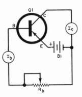
(adjusting Rb) and recording the corresponding values of Ic. A typical curve might look somewhat like the one illustrated in Fig. 6.
