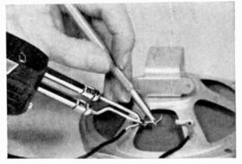
POSITION AND HOLD WIRE Joint must remain perfectly still until solder sets. An easy way to accomplish this is to hold the wire with a soldering aid. Blowing on solder will speed setting.
