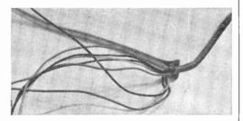
jacket down the side, and remove the color-coded hookup wire. The cable can be obtained at most radio parts suppliers for a few cents a foot.
