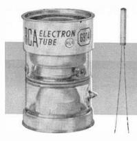
Image tube (far left) converts invisible infrared into visible light; the World War II "snooperscope," which enabled troops to see in the dark, employed such a detector. Modern single-crystal infrared detector (left) is a byproduct of transistor development; unit produces output voltage in proportion to amount of infrared radiation falling upon it. Both devices are products of Radio Corporation of America.
