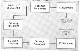
may sound complicated, this entire operation takes only about one-tenth of a microsecond. When the process is complete, the circuit is once again in equilibrium, although the tubes have of course reversed their relative positions.
