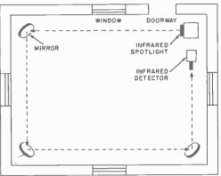
frared beam is focused on photocell PC1; you may have to put a larger lamp in the spotlight for long beam lengths or when mirrors are used.
