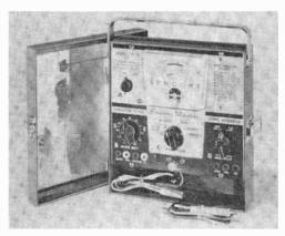
the tester is an r.f.-a.f. signal generator and voltmeter-milliammeter for troubleshooting purposes. The Transi Master is supplied with a test probe that connects to all three leads of a transistor at one time, and a mirrored-top case for ease in checking printed-circuit boards. Price, \$49.50. (Sencore—Service Instruments Corp., Addison, Ill.)
