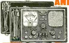
During the past 5 years, millions of transistor radios and other transistar operated devices have been imported and produced in this country with no adequate provision for servicing this ever increasing output. The Model 88 was designed specifically to test all transistors, transistor radios, transistor recorders, and other transistor devices under dynamic conditions.
