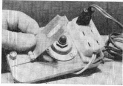
switch will serve as the power outlet. Connect the switch in series with the receptacle and a heavy-duty power cord and plug. To operate the footswitch, plug the power tool into the receptacle and step down on the treadle. The power (Continued on page 107)
