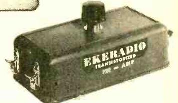
You can build a powerful two-stage amplifier or pre-amp which can be used as a phonograph amplifier or amplifier for a crystal set, and as a pre-amp for crystal or magnetic pick-ups. Kit comes complete with two transistors, volume control with switch, attractive plastic case with a snap bottom, and is powered with a single penlight cell with an output of nearly 1/4 of a watt. Complete with easy-to-follow instructions. \$5.95 postpaid.
