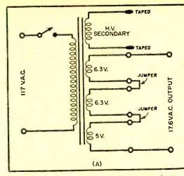
however, it is necessary to determine their phasing. For instance, if a 6.3-volt winding is connected to a 5.0-volt secondary in series-aiding, their output voltages are in phase and add up to yield a total voltage of 11.3 volts. On the other hand, reversing one connection places the secondaries in series-opposing. In this condition, the voltages are 180° out-of-phase and subtractive, giving an available potential of 1.3 volts.
