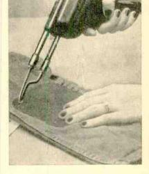
Two ways of using the smoothing tip are shown at right. To seal a patch on a pair of well-worn dungarees, stroke the smoothing tip around the edge of the patch; then crisscross it over the patch to insure a good seal. A plastic bag is being sealed airtight in the operation at the lower right. In the photo above, the regular tip melts the plastic binder which holds 300-ohm twin-lead wires in place.
