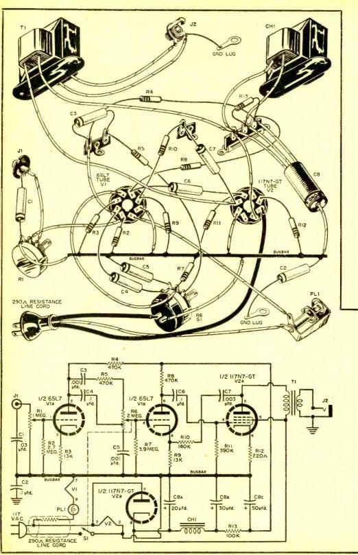
Underside of amplifier chassis, showing terminal board and point-to-point wiring. You will note that the major components are crowded to the back of the chassis. While this keeps hum away from the tone and volume controls, the top of the chassis looks somewhat unbalanced. You may want to experiment with alternate layouts to obtain a more balanced appearance while retaining minimum hum.
