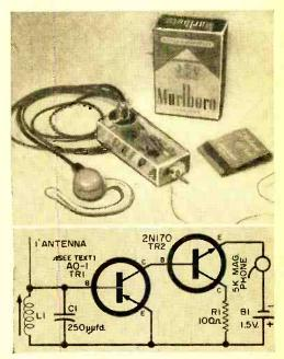
Fig. 3. Hugh Van Horn's two-transistor receiver. It is shown above assembled in a small plastic box.
