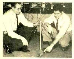
mitter will send a steady radio signal for a distance of 25 miles throughout a whole day. The gunpowder pops up the selfcontained antenna which is shown in the photo in its fully extended position. Although operating above 280 mc., the circuit is printed on a special insulator, uses transistors and is really sealed in a standard sardine can.
