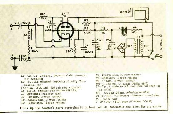
If your antenna lead is too close to loop L2, it will cause a signal to be fed back and create an unstable circuit. This dictates the use of 300-ohm twin-lead (TV type) lead-in. The antenna and ground, or antenna and counterpoise, are connected to the far end. I used two 30' pieces of wire attached to the end of a 40' lead-in. These can be strung out-of-doors or in the attic as long as the antenna ends do not come close to the booster.
