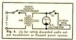
basic Ohm's law equation:  $I = E_{\text{sec}}/R_{\text{load.}}$ The result will tell you the current rating of the tube for which the transformer may be used.
