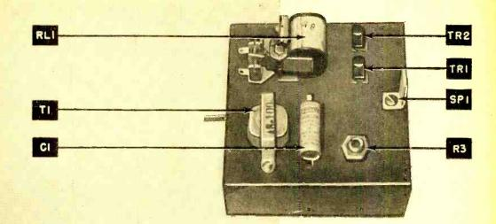
Since this relay is suitable for many uses, each setup will be best determined by the constructor. The one shown in the photo is an experimental hookup with plenty of open space, although it is assembled on a chassis measuring only  $3\frac{1}{2}$ " x  $3\frac{1}{2}$ " x 1". The photocell should be thoroughly shielded by a hood or a suitable length of cardboard tubing to prevent extraneous light from entering the cell.
