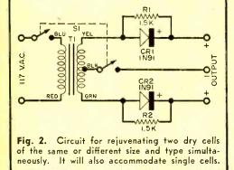
mount slide switch *S1* and the three Fahnestock clips on the cover. Then cement the transformer in the lower half at the hinge end. The red and blue leads should be toward the hinges.
