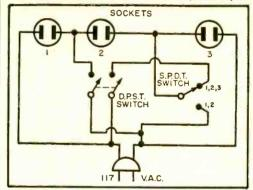
ating. Closing the double-pole switch puts the lamps in parallel; opening it puts them in series. Always dim the lights when switching between two and three bulbs.
