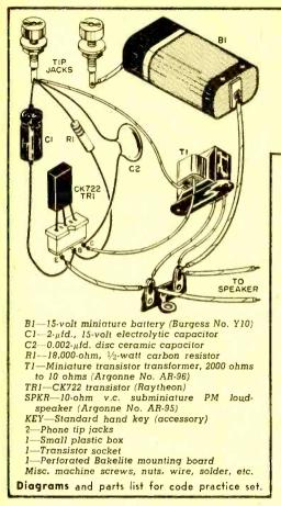
ted over the ends of the phone tip jacks which serve as the hand key terminals. Transformer T1 is mounted on the subminiature loudspeaker's frame.
