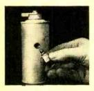
with miniaturized equipment. Aerosol pressure cans are an excellent source of such knobs. These are threaded and may be removed by simply unscrewing them from the can. If the knob is to
