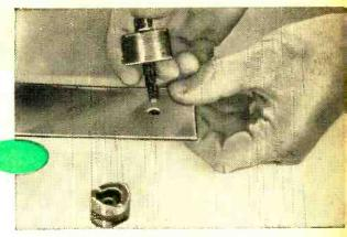
**Cutting element** of chassis punch is threaded onto the bolt from below the chassis. Bolt is now turned a few times with a wrench (photo at right). This action draws the cutter through the metal and into the socket. Result is a perfectly round, very clean-cut hole. These tools come in numerous diameters.
