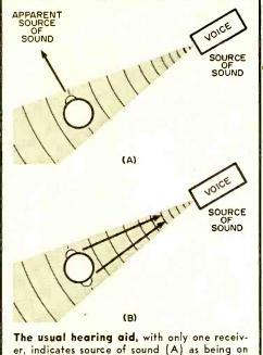
er, indicates source of sound (A) as being on the side the aid is worn. Wearing binaural aid, the hard-of-hearing would be able to pinpoint source of sound (B), even with eyes closed, since it gives "stereophonic" hearing.
