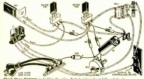
Check these diagrams in building the relay. Parts layout need not follow photo above; you may
