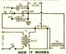
This is a slide-wire type of bridge circuit. Whenever the bridge is adjusted to null, the resistance between points A and B of potentiometer RI is in the same ratio to the resistance hetween B and C as the standard capacitor (C1, C2 or C3) is to the unknown capacitor. At the mid-scale setting of potentiometer RI, the resistance from A to B equals the resistance from B to C, the ratio is 1, and the un-
