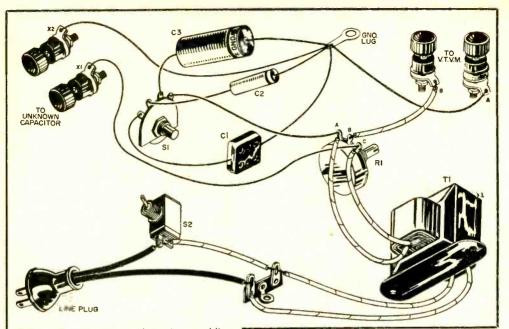
Follow the diagrams and text in assembling your capacitance bridge. See parts list below.
