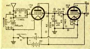
PARTS LIST B1--1.5-volt "D" cell B2--67.5-volt battery C1--365-µµfd. variable capacitor C2--250-µµfd., 300-volt capacitor C3, C4--0.005-µfd., 300-volt capacitor L1--Feri-Loopstick R1--1.5-megohm resistor R2--250,000-ohm resistor R3--1-megohm resistor S1--"On-off" switch (see text) V1--1T4 tube V2---3S4 tube
