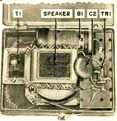
Layout of parts is not critical, but if you want to color the plastic case, don't mount the parts until atter the paint has dried. Check all wiring before connecting the hand key or trying the unit.
