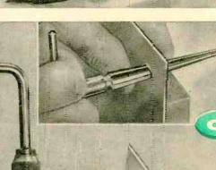
Chassis punch is excellent tool for making mounting holes for tube sockets, i.f. transformers, electrolytic can capacitors, phono jacks, auto radio antennas, and the like. First step is to drill a starting hole in the metal the size of the bolt. Then, assemble the upper two parts of the punch—the bolt and a socket the size of the hole to be made. Third part is the actual cutter, shown in photo at right resting on work table.
