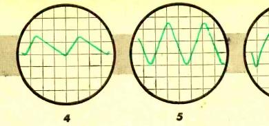
shown on the screen. When the sweep frequency is onehalf of the signal frequency observed, two full cycles are displayed on the trace.
