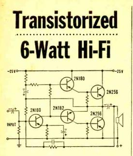
New experimental all-transistor hi-fi amplifier delivers 6 watts with:  $\pm 1.5$  db response from 30-15,000 cps, less than 1% harmonic and 2.5% intermodulation distortion, noise level 74 db down. Simple circuit features: pre-driver, driver, and final amplifier using low-cost CBS 2N256 power transistors . . . negative feedback . . . complementary-symmetry driver . . . direct coupling . . . economical power supply.
