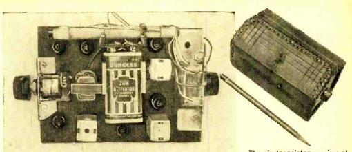
Brooklyn 30, N. Y., can supply small currents (up to a few ma.) at moderate and low voltages. Easy to use and completely shock-free, it is valuable for checking out one- and two-stage transistor circuits.
