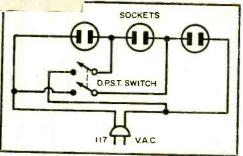
box when the front panel is secured to it. Interconnecting wires between receptacles and switch must not be smaller than #18 gauge and should be tinned for easy soldering. The line cord carries the full load—almost 15 amperes in the parallel connection—and so must not be smaller than #14 gauge. The toggle switch must be capable of carrying 10 amperes. —Harvey Pollack
