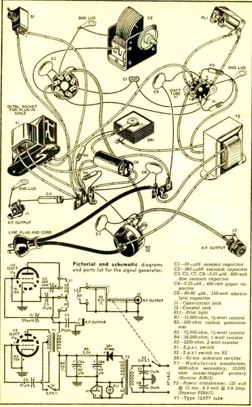
with a  $4\frac{3}{2}$  x  $5\frac{1}{2}$  steel shelf. The 12AT7 is mounted vertically under the chassis, and the coil socket is mounted on a right-angle bracket formed from a  $1\frac{3}{2}$  x  $2\frac{1}{2}$  piece of steel. If short leads are maintained in the coil (L1) and variable capacitor (C2) circuitry, you will find that there is nothing critical in the wiring.
