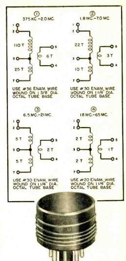
Four plug-in coils, such as the one shown here, cover the basic frequency range. Data for each coil is given in the box above. You can salvage the coil forms from defective octal tubes as described in the text.
