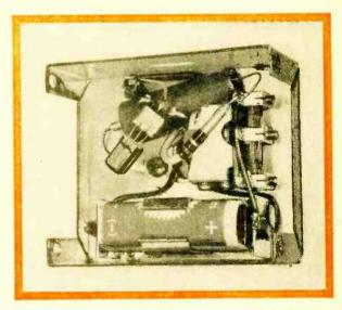
Inside the slave unit. Sun Battery is mounted behind opening in box, and special miniaturized relay is at the right.
