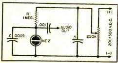
shown in the diagram will work to approximately 3000 cycles before oscillation ceases. At this "drop-out" point, the NE-2 will glow brightly, indicating that it is completely ionized.
