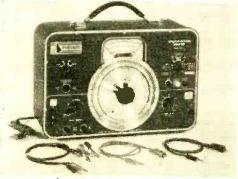
vacuum-tube ohmmeter scale reads accurate insulation resistance of capacitors.
