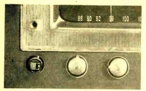
Mounting the control behind the front panel takes little time and effort. Control shafts may be cut to any desired length for neat, correct fit.
