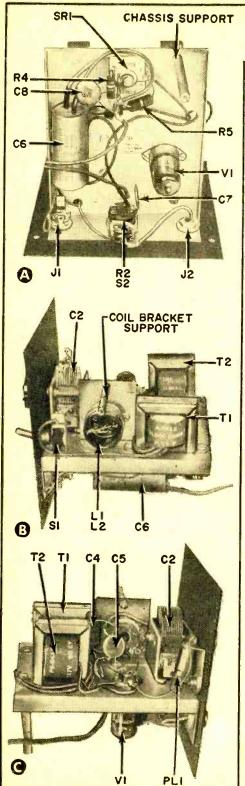
Three views of the "Economy" signal generator chassis show placement of the major components: (A) bottom view; (B) right side view; and O left side view. Layout is very critical.
