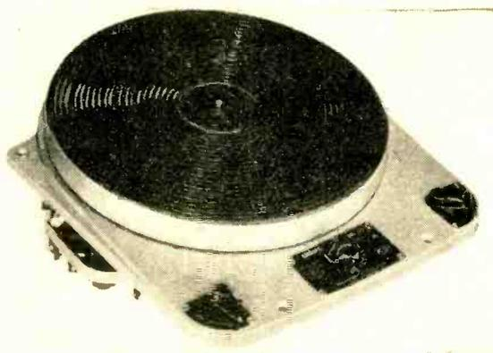
**Presto Model T-18** is heavy, carefully machined and balanced aluminum casting driven by mechanism of utmost simplicity. Three idlers, one for each speed, transmit power from motor to turntable. Idlers are disengaged in "off" position. Reported performance data: speed accuracy, 0.25%; noise level of shaded pole motor, -40 db, of hysteresis motor, -50 db. Net, \$53.50 for shaded-pole motor; \$108.00 for hysteresis motor. Presto Recording Corp., Paramus, N. J.
