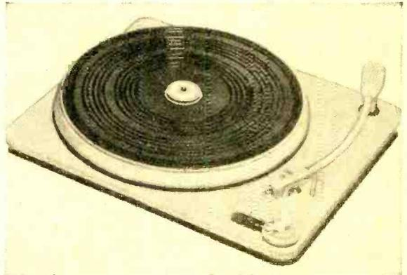
Components Corporation Model PBT gets maximum flywheel effect from 25-lb. cast-iron turntable. Nylon sleeve bearing, in which it rotates, reduces metal-to-metal contact. Motor is double-shock-mounted at maximum distance from turntable to reduce magnetic hum pickup. Reported performance data: 0.25% speed accuracy; 0.05% wow and flutter; -70 db rumble. Special spindle centers record on turntable and prevents slipping. Net, \$99.50. Components Corp., Denville, N. J.
