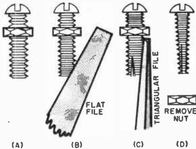
Finally, remove the nut, as shown in (D), thus restoring any damaged threads . . . . . L.G.
