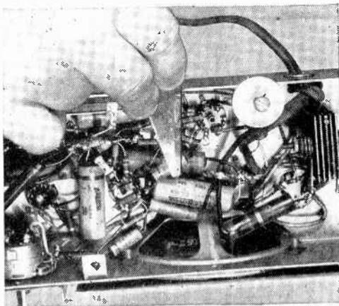
referring to a tube manual. If there is a d.c. voltage across this resistor, with the grid end positive, either the coupling capacitor is leaky or the output tube is "gassy" (a tube tester check will frequently fail to identify a "gassy" tube).
