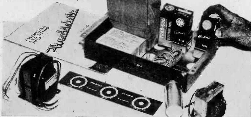
Underchassis view after "fixed" components are mounted. Wires at top are from output (left) and power transformer (right).
