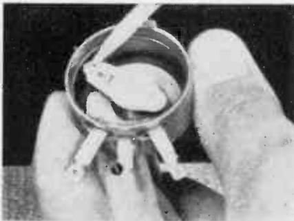
A typical volume control with the cover removed to show the sliding arm and circular contact. Dirt often appears between the arm and contact ring, resulting in noisy reception.
