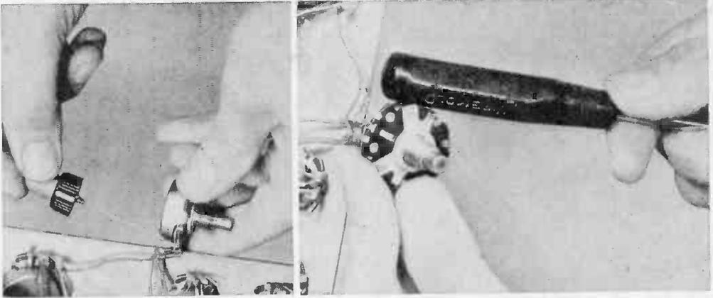
(Left) Before changing a control try a drop of contact cleaner. This fluid may be inserted wherever there is an open place or allowed to slide down the shaft. This is usually a temporary expedient. (Right) Another technique that produces the same results is tapping the control case with a hard rubber tool, as shown.
