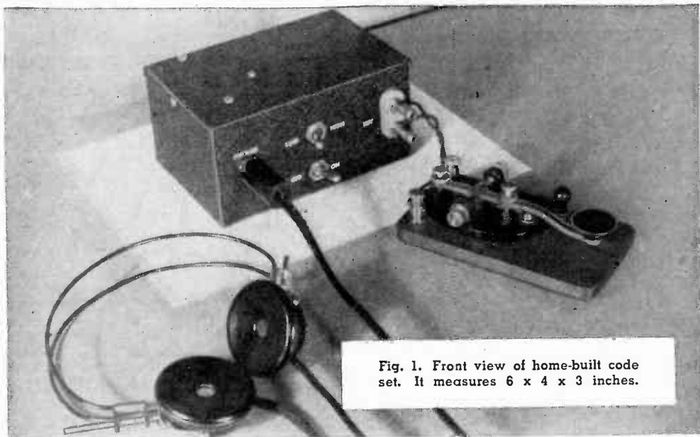
Fig. 1. Front view of home-built code set. It measures 6 x 4 x 3 inches.
