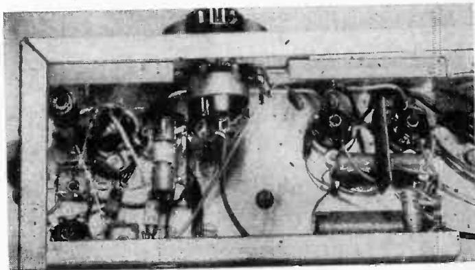
Fig. 9. Under chassis view of the completely wired radio.
