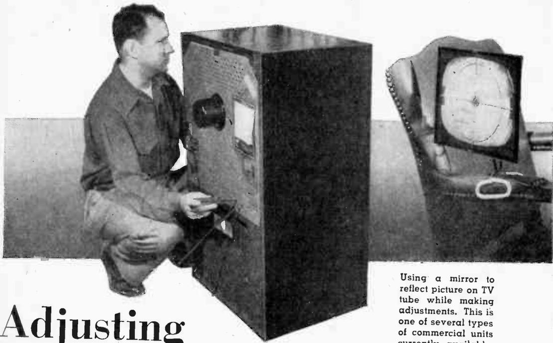
Using a mirror to reflect picture on TV tube while making adjustments. This is one of several types of commercial units currently available.
