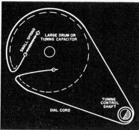
Fig. 4. Basic technique for replacing worn or broken dial cord. Special stringing arrangements may involve reference to service books.
