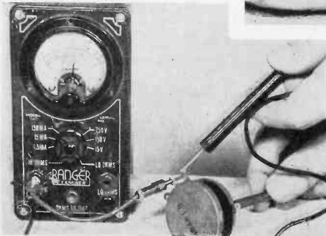
By disconnecting the suspected control from its circuit, with receiver inoperative, an ohmmeter may be connected from middle terminal to first one and then other terminal and by moving the shaft slowly, operation of control can be checked.
