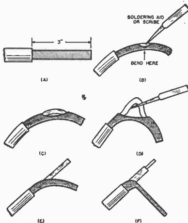
stripping insulation from the inner conductor and flatten the extra length of braid to form a ground strap as shown in (F) . . . . . L.G.
