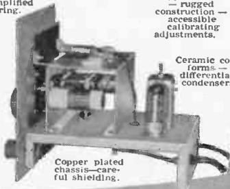
Ceramic coil forms—differential condenser.
