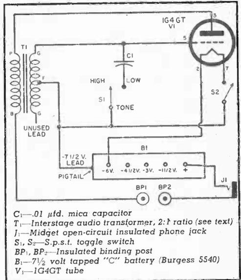
battery-operated tube is used in a simple hookup. The transformer, *T*<sub>1</sub>, is a small audio unit. Almost any audio transformer sold as an "interstage coupling" unit will work in this circuit.
