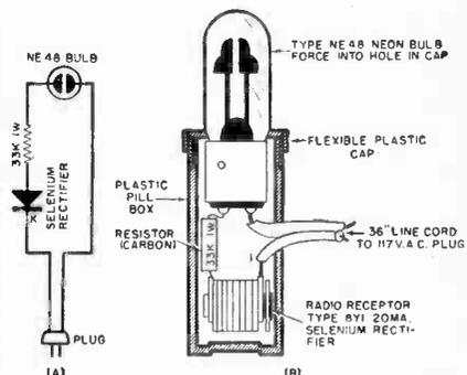
Fig. 3. Proper way to use the 60-cycle strobo diagrammed above. Technicians and audiophiles will find this handy for checking the speed of phonograph turntables.
