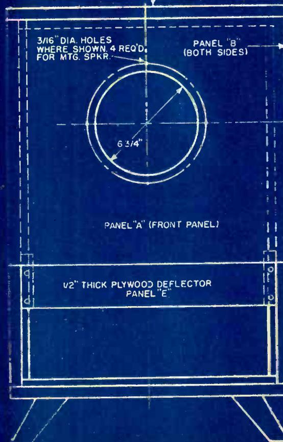
3/16" DIA. HOLES WHERE SHOWN, 4 REQ'D. FOR MTG. SPKR.
