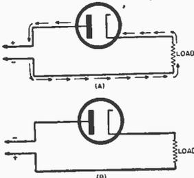
Although alternating voltage is applied to the circuit, current flows only in one direction. This particular process is known as "rectification". Thus the tube
