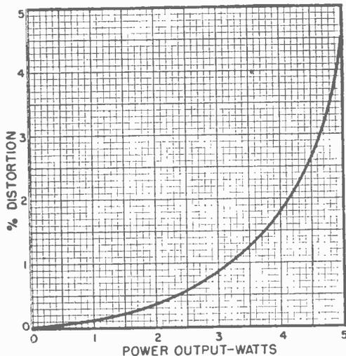
Fig. 2. Total harmonic distortion of the amplifier measured at 1200 cycles across a 16-ohm resistive load. Refer to article.
