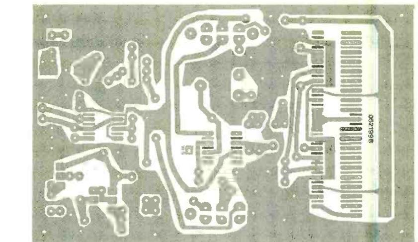
Fig. 3. The RF Field-Strength Meter is built on a single-sided PC board. No ground plane is needed on the opposite side.
