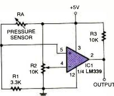
*Fig. 5. This circuit converts the output of a conductive foam pressure sensor to an on/off type switch output.*
