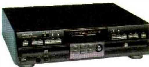
The dual-tray XC-RW700 CD recorder (\$650) from Aiwa offers 4X dubbing that allows a 60-minute CD to be copied in just 15 minutes. One tray is playback only, and the other can be used for both playback and recording. The unit is compatible with both CD-R and CD-RW discs.
