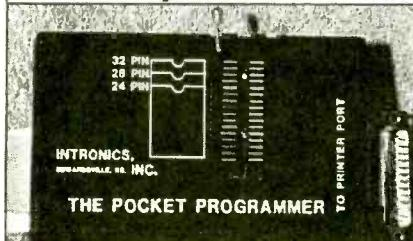
The portable programmer that uses the printer port of your PC instead of a internal card. Easy to use software that programs Eprom, EEPROM, Flash & Dallas Ram. 27(C) / 28(C) / 28F / 29F / 29C & 25XX series from 16K to 8 Megabit with a 32 pin socket. Adapters available for Pic, PLCC, 5-Gang, 874X, 875X MCU's, 40-Pin X 16 & Serial Eprom's, 82/74 Prom's and Eprom Emulator to 32K X 8.
