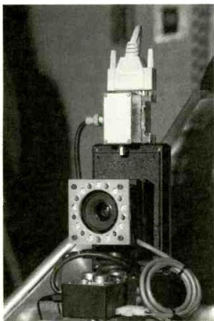
Infrared Ranging via Image Subtraction (IRIS) sensors can see through fog. IRIS capitalizes on the fact that all vehicles contain retroreflective surfaces. On automobiles, these are found in taillights. IRIS captures and compares two images: one illuminated with its infrared beam and the other illuminated by ambient light. The difference between the two images is the retroreflective surface, enabling you to see taillights or a reflective bumper sticker.
