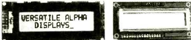
First, (shown above left) from Solomon, the LM1140-SYLU, with LED backlight. Standard 16 x 2 arrangement of 5 x 7 dot matrix characters 2.95mmW x 5.56mmH with cursor. COB driver with 8 bit parallel interface. Module size: 85mmW x 36mmH. Viewing area: 63.5mmW x 15.8mmH with dots. **Brand New.**
