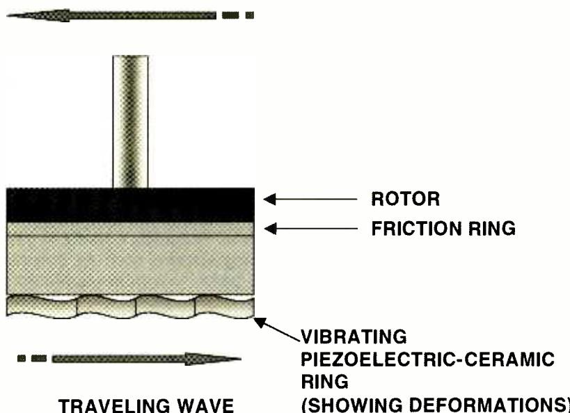
Fig. 2. This side view of a typical ultrasonic motor shows how the ripples in the stator resemble ocean waves. Like water, the piezo-ceramic crystals don't move laterally—only up and down—but the energy moves across the stator face at a high rate of speed.
