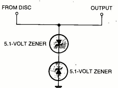
Fig. 7. A suitable interface circuit connects a piezo disc to a TTL-compatible input or op-amp.
