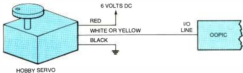
Fig. 1. Follow this basic wiring diagram to connect a standard R/C servo to the OOPic. Most servos use consistent color coding for their wiring: black for ground, red for +V, and yellow or white for the input signal.
