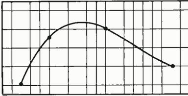
Fig. 5. The Postscript code given in Listing 1 draws a Bezier cubic-spline curve through four selected data points; here is an example of that program's output.
