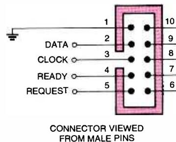
Fig. 1. The connector pinouts for the Mitutoyo Digimatic machine-tool gauge interface use a standard 2-by-5-pin header; it can be used with a ten-conductor flat cable.
