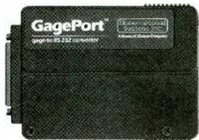
Fig. 2. Here is a typical older Digimatic-to-computer interface.
