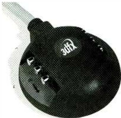
Except for cable TV and FM antenna, connections to the 3500 TV are made via the innovative I/O Pod shown here. Forget about reaching behind your PC to work with video sources.
