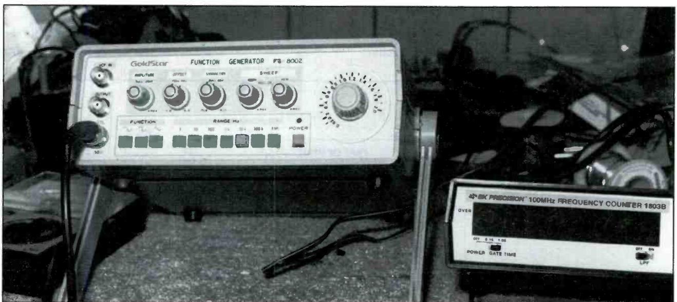
Figure 3. You can use a function generator, or audio signal generator, in conjunction with an oscilloscope and external audio amplifier to isolate most sound problems.
