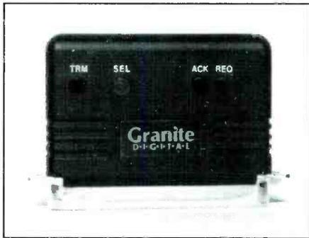
**Figure 2.** The SCSI bus analyzer has four LEDs that are used to monitor four control lines on the SCSI Bus. By “reading” the LEDs, the analyzer provides the technician with information on the status of the SCSI Bus.
