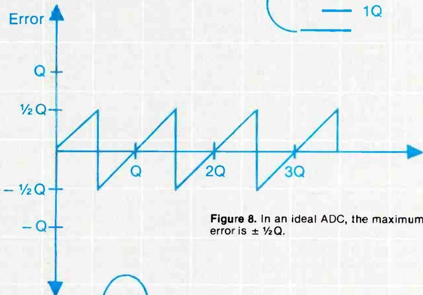
**Figure 8.** In an ideal ADC, the maximum error is  $\pm \frac{1}{2}Q$ .
