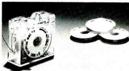
solid-copper wire. To operate the cut/strip mechanism, the wire is first drawn out to the desired length. Then a built-in plunger cuts the length free from the roll while a gentle pull through the stripping blade removes the insulation.
