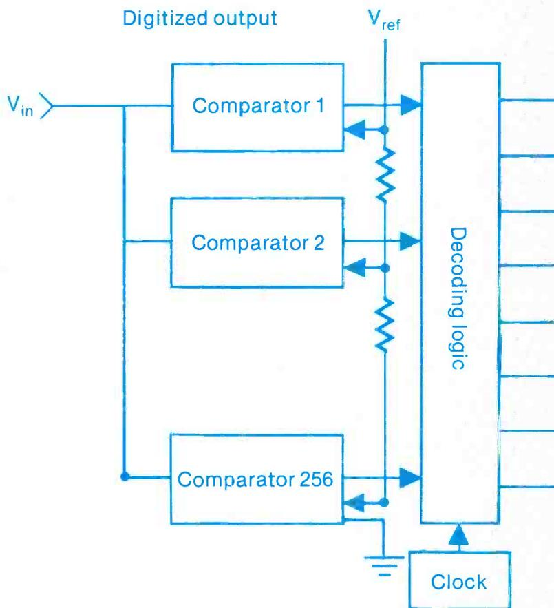
Figure 13. The flash converter utilizes a row of comparators in parallel to perform a conversion in one clock period.
