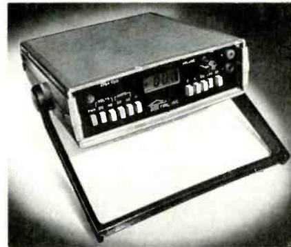
cuits, this multimeter is an analog input instrument adaptable to particular needs. The battery-powered multimeter is accurate to  $\pm 0.1\% \pm 1$  LSD on dc voltage and speaks every seven seconds or on the press of a button.
