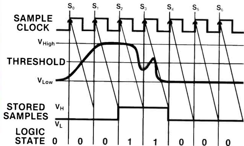
Figure 6. The ones and zeroes displayed by a logic analyzer are logic-level indications of the level of the input signal when the analyzer clock signal edge occurred.
