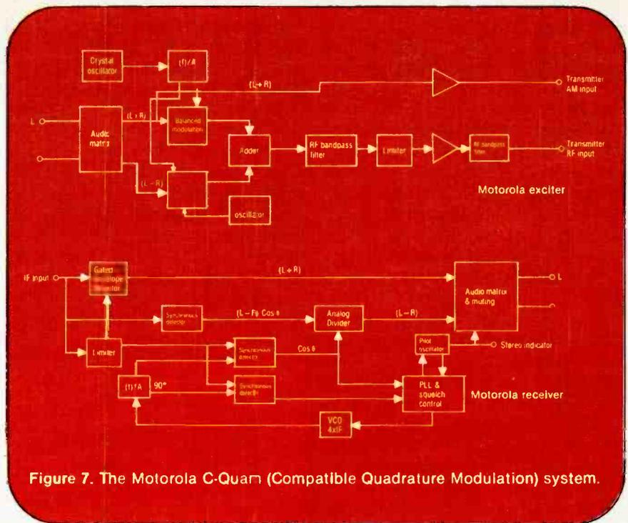
Figure 7. The *Motorola C-Quam* (Compatible Quadrature Modulation) system.
