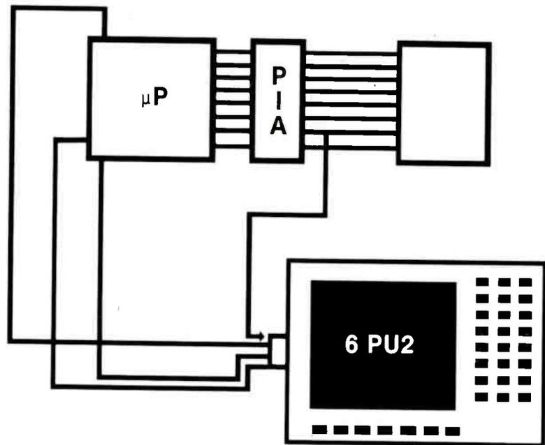
Figure 5. Signature analysis takes advantage of the fact that any pin of a digital integrated circuit has a specific pattern of ones and zeroes flowing through it.
