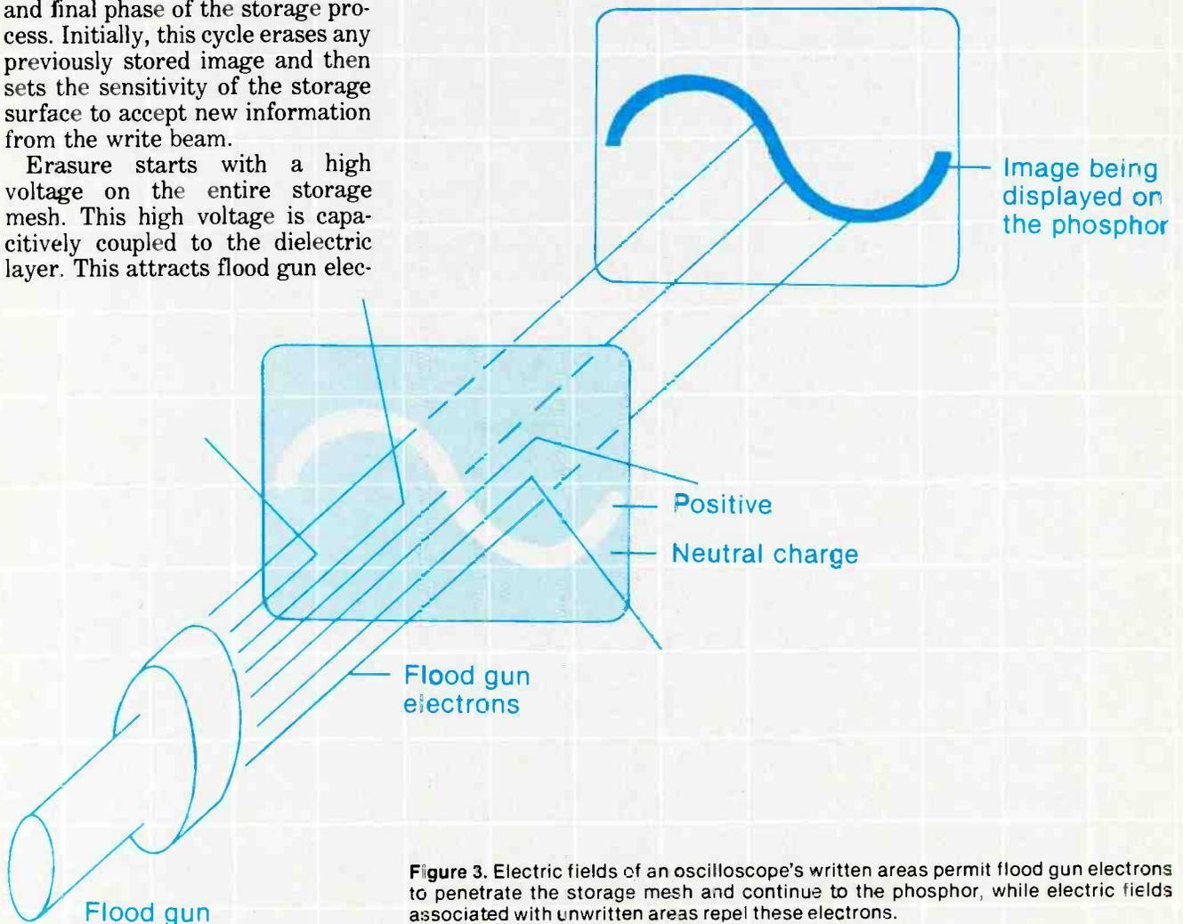
**Figure 3.** Electric fields of an oscilloscope's written areas permit flood gun electrons to penetrate the storage mesh and continue to the phosphor, while electric fields associated with unwritten areas repel these electrons.
