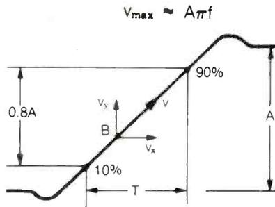
Assuming that the maximum spot velocity equals the average velocity between the 10% and 90% points, then  $V_y = 0.8A/T$ , where  $T =$  observed pulse rise time.
