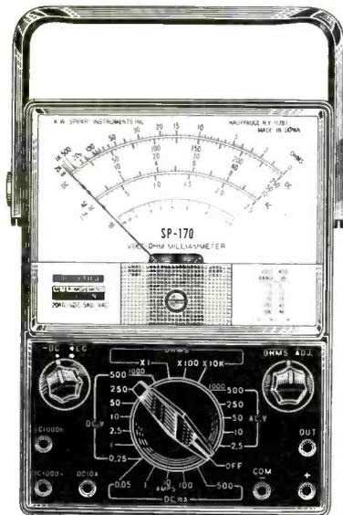
ac/dc multi-tester. The unit features a 21-position selector switch with an off position, full-view window, easy-reading 2-color scale, fuse protection on all ranges except 10Adc, safety-designed front panel and a simplified polarity selector switch. Sensitivity is 20K  $\Omega$ /Vdc and 5K  $\Omega$ /Vac.
