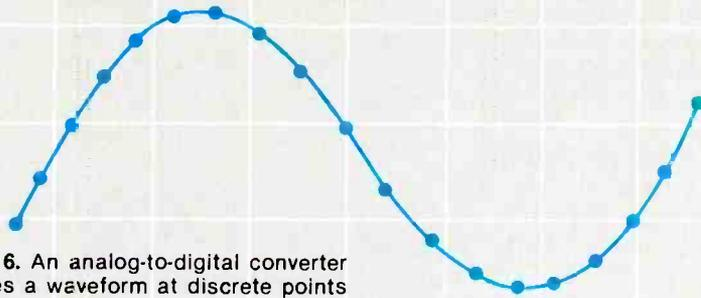
**Figure 6.** An analog-to-digital converter samples a waveform at discrete points and converts the analog voltage into a digital value.
