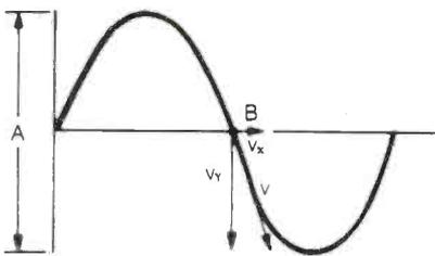
When a beam writes a sine wave, the vector spot velocity ( $V$ ) is composed of both the vertical ( $V_y$ ) and horizontal ( $V_x$ ) component, which are related as:
