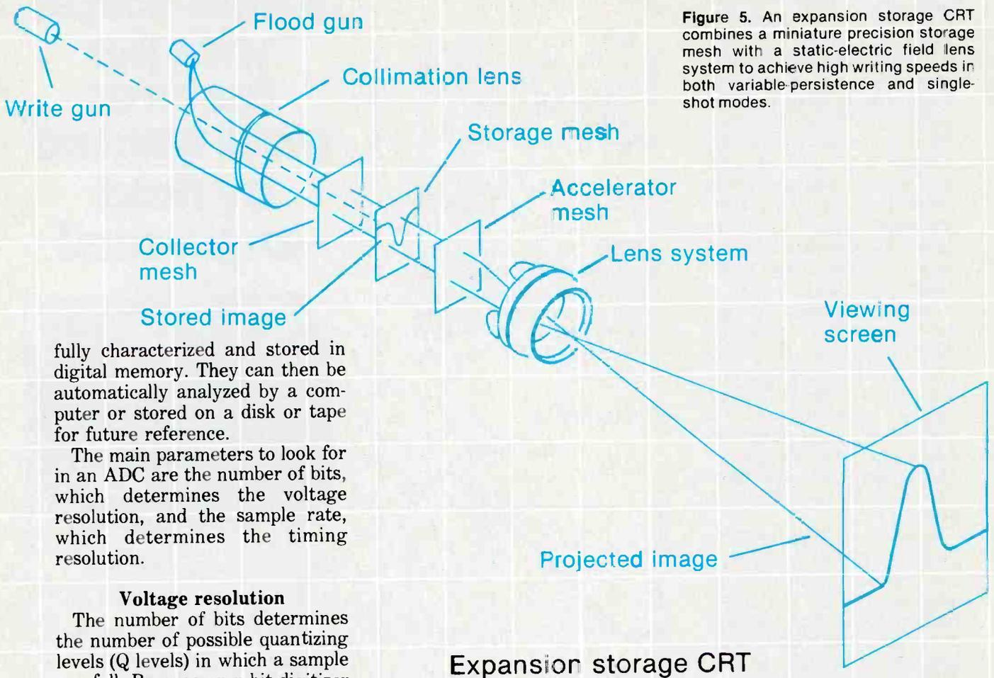
Figure 5. An expansion storage CRT combines a miniature precision storage mesh with a static-electric field lens system to achieve high writing speeds in both variable-persistence and single-shot modes.
