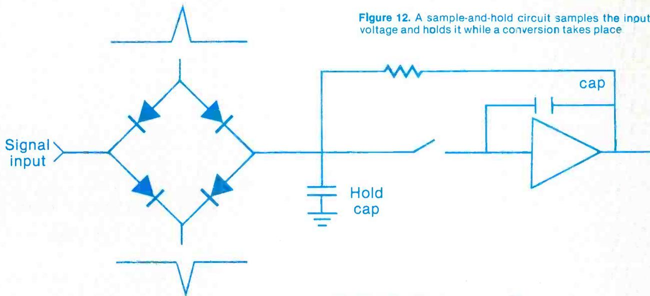
Figure 12. A sample-and-hold circuit samples the input voltage and holds it while a conversion takes place
