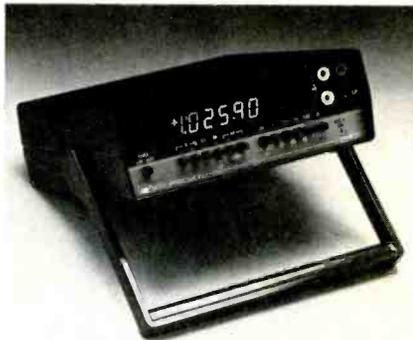
resolution. Designed for bench-type use, these instruments provide manual ranging and manual function control only.
