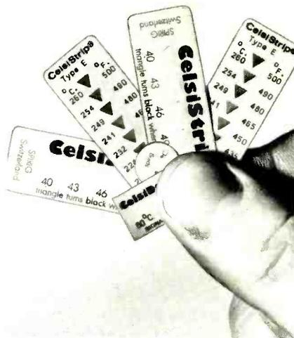
sensitive white triangle turns irreversibly black when the surface reaches the specific temperature level of that triangle, and is accurate to +1%.
