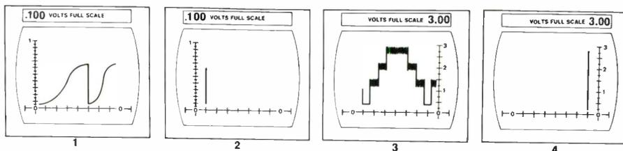
To read peak-to-peak voltages utilizing Cali-Brain, note the full scale voltage reading in the bezel above the screen (fig. 1—.100 volts full scale) (fig. 3—3.00 volts full scale). Pull out the Cali-Brain knob and you will notice that the 1st waveform in fig. 2. reads .067 volts P-P and the second waveform in fig. 4. reads 2.95 volts P-P.
