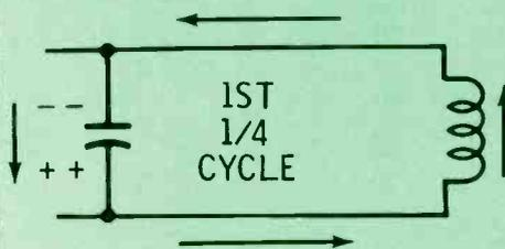
When the battery was disconnected, "positive" coil current flowed from the coil (source of power) into the capacitor and charged it with a negative voltage. The coil current gradually decreased in step with the increase in capacitor voltage. This action is shown between points "A" and "B" in Photo 2.
