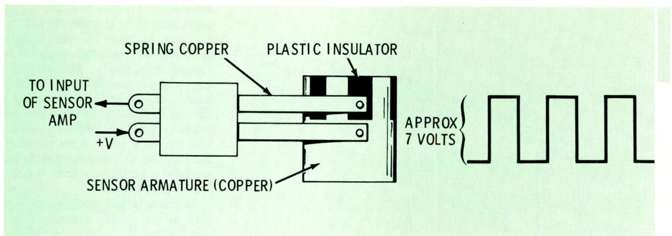
Fig. 8 A) Drawing of cartridge-stop sensor mechanism used in many cassette tape players. B) Rectangular pulse, produced by sensor mechanism, drives sensor amplifier.
