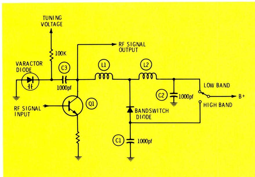
Fig. 3 Representative RF amplifier with bandswitching and varactor tuning.
