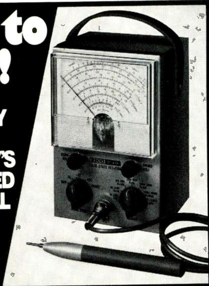
Use the battery powered Solid State EICO 239 on your bench or in the field. Check semiconductor and vacuum tube circuits. 11 Megohm DC input impedance. Read AC rms and DC voltages in seven steps from 1 to 1000 volts on large 4 1/2" meter. Measure and read peak-to-peak AC to 2800 volts. Check resistance from 0.2Ω to 1000MΩ on seven ranges. Provides a total of 28 useful ranges on 12 accurate scales. Automatic battery check. Includes exclusive DC/AC ohms Uniprobe™. Factory Assembled, \$59.95.
