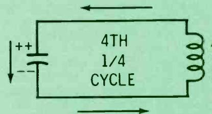
Positive voltage from the capacitor (source) flowed into the coil producing an increasing "positive" coil current. This action is between points "D" and "E" in Photo 2. The capacitor voltage was zero and the "positive" coil current maximum at point "E".
