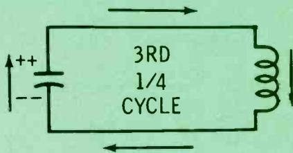
"Negative" coil current (source) decreased as it charged the capacitor with positive voltage. Points "C" to "D" in Photo 2.
