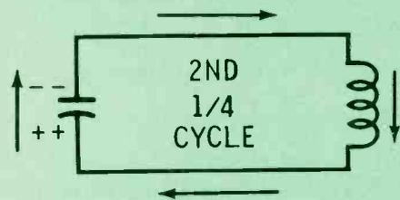
The negative capacitor voltage (source) discharged back into the coil and caused "negative" coil current. This corresponds to the waveform portion "B" to "C" in Photo 2.
