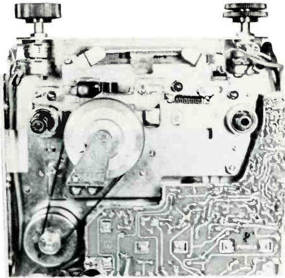
**Fig. 5** Bottom view of Craig Model 3501 cassette tape player, which employs a belt between the motor pulley and the flywheel, but uses idler wheels to drive the take-up sprocket.
