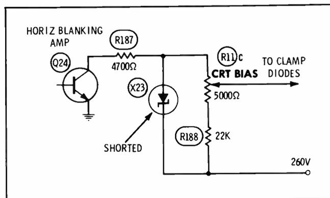
An ohmmeter test of the zener diode should be sufficient to detect such leakage. ▲
