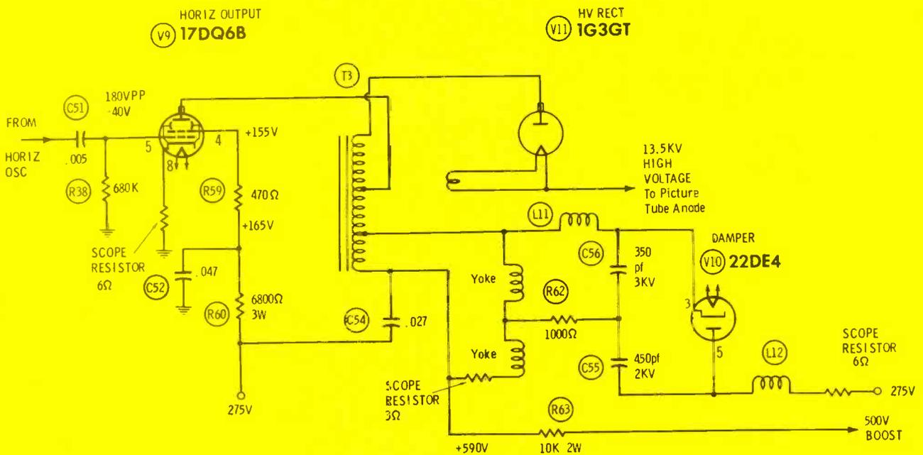
Fig. 5 Complete schematic of the horizontal sweep and high-voltage section of the Sears 456/528.51912 b-w television chassis. Normal DC voltages for this one individual chassis are included. Waveforms will be added next month, to illustrate a detailed discussion about troubleshooting the horizontal sweep sections of television receivers.
