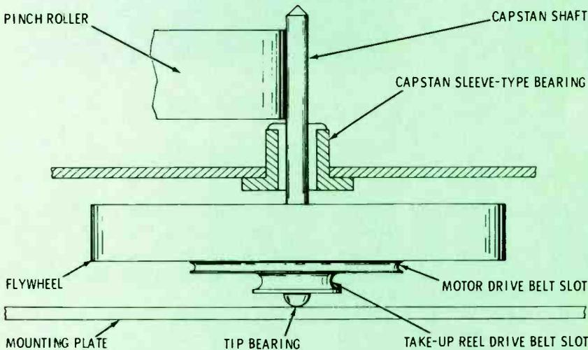
**Fig. 6** Side-view drawing of capstan and flywheel assembly used in most automotive cassette tape players.
