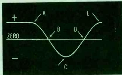
Shows the power supply voltage and the first cycle of the sine wave of coil current. Beginning and ending points of each 1/4 cycle are indicated by letters.
