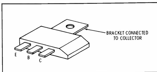
Replacement transistors, Zenith part number 964-27986, have an adequate heat sink that is part of the transistor and is connected internally to the collector. These extruded flat brackets, projecting from the tops of replacement transistors, should NOT be clipped to the aluminum shield, because this would short the collector circuit.
