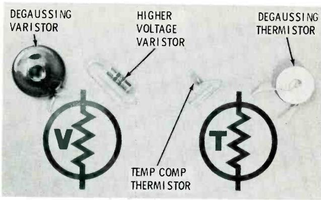
Fig. 1 Examples of varistors and thermistors and their symbols.
