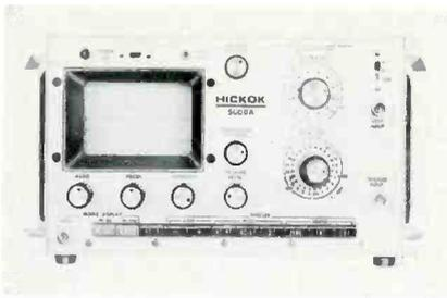
with a vertical bandwidth from DC to 25 MHz (-3 dB point), has been introduced by the Hickok Company.
