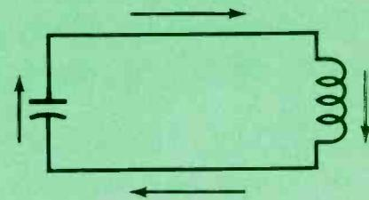
The capacitor voltage (source) was zero, and the "negative" coil current was maximum at point "C".
