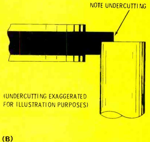
**Fig. 13** A) Side-view drawing of take-up spindle drive mechanism. B) Enlarged view of drive shaft and rubber tire on take-up reel, showing undercutting of tire by shaft, caused by improper alignment and/or wear.
