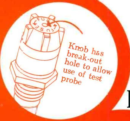
Knob has break-out hole to allow use of test probe
