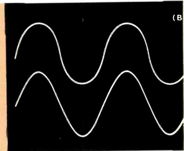
**Fig. 6** A varistor passes the same amount of current whether the applied voltage is positive or negative, provided the amplitude of the applied voltage is the same. A) Circuit of a sine wave applied to a varistor. B) Bottom waveform is the input sine wave for comparison; both the positive and negative peaks of the top waveform have been rounded by varistor current. The existence of identical positive and negative alterations prove that a varistor has no diode characteristics.
