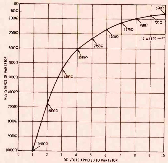
Fig. 3 A graph of applied voltage versus resistance can be computed by Ohm's law, using the values in Fig. 2.
