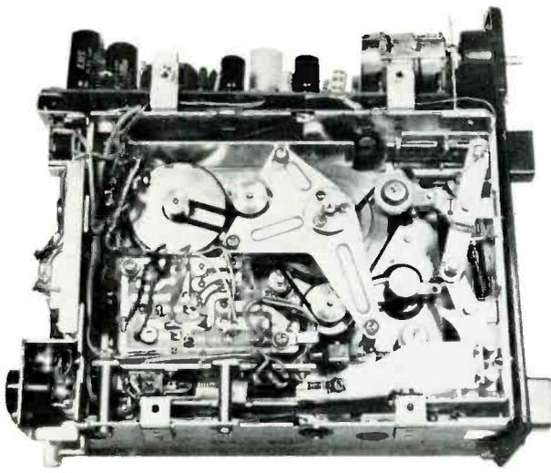
**Fig. 4** Bottom view of Automatic Radio Model ACS-6000 cassette tape player, which used a belt-drive system between motor and flywheel and take-up sprocket.
