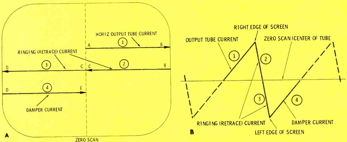
**Fig. 1** Locations where the four steps of horizontal deflection occur on the screen of the picture tube, and also where they are located on the waveform of yoke current. This information can help technicians correlate visual symptoms with the area of the circuit where the defect is most likely to be. A) Power to scan from the center of the picture tube screen (point A) to the right edge (point B) is supplied by plate current of the horizontal-output tube. Current from
