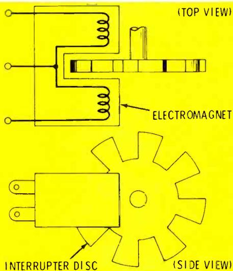
Fig. 10 Top- and side-view drawings of interrupter-disc-type of cassette-stop sensor.
