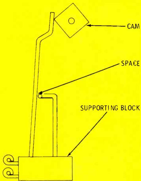
Fig. 9 Drawing of cam-type of cassette-stop sensor mechanism.
