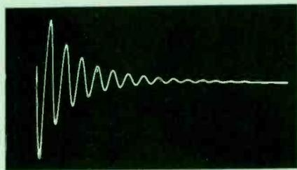
A DC supply voltage was connected to a tuned circuit long enough for the current to reach maximum. When the power supply was suddenly disconnected the damped wavetrain of sine waves shown here was produced. The first 1/4 cycle is not displayed on the scope screen because the vertical amplifier section of this particular triggered-sweep scope is not equipped with a delay line.
