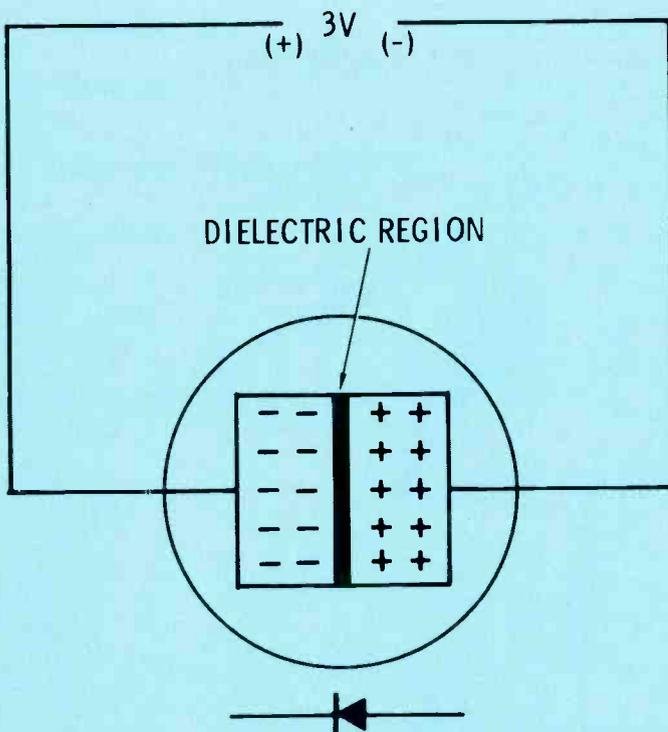
Fig. 1 Varactor diode with moderate reverse bias.
