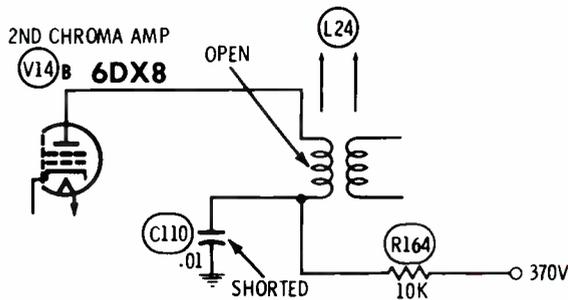
**Symptom**—no color; no plate voltage on pin 6 of V14
