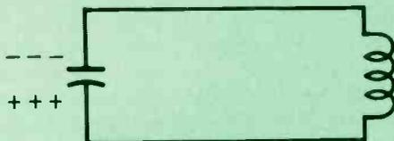
The coil current was zero at point "B" in Photo 2, and the negative voltage across the capacitor was nearly 50 times larger than the original battery voltage.
