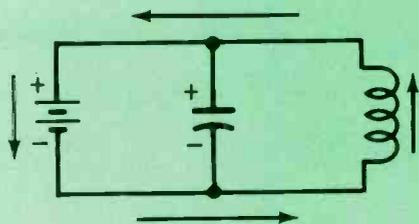
A battery was the source of the maximum "positive" coil current. The small battery voltage also appeared across the capacitor.
