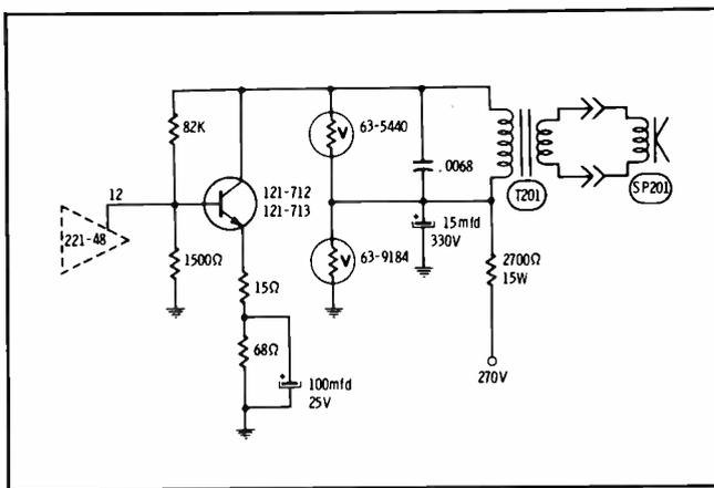
Do not service the receiver without a speaker or a load resistor connected across the speaker output leads, because the output transistor and the varistor can be damaged by the high peak voltages which can result.
