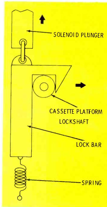
**Fig. 12** Drawing of lock mechanism which holds cassette platform in play position until cassette-stop/eject amplifier energizes eject solenoid K1. Lock bar is then pulled up by solenoid plunger and cassette platform drops to "rest" position, forcing cassette out slot in front of player.
