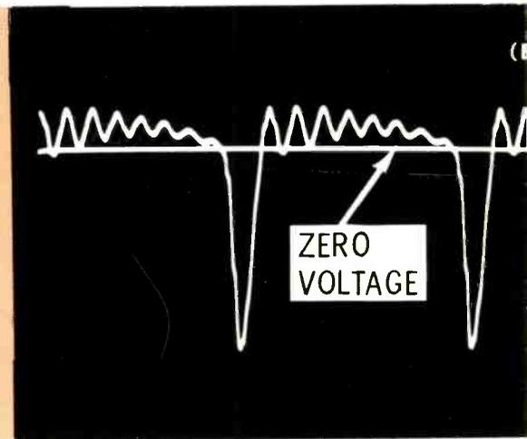
**Fig. 7** DC voltage can be obtained from varistors, if the applied waveform is non-symmetrical. A) Circuit which produced the waveforms and DC voltages. B) Scope waveform of the input signal, showing the true zero voltage line. The negative-going voltage is greater than the positive-going.
