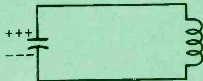
The coil "negative" current (source) reached zero, and the capacitor was charged to maximum positive voltage at point "D" in Photo 2.
