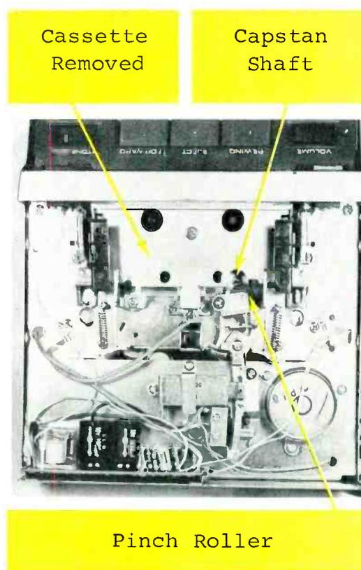
Fig. 3 A typical automotive cassette-type tape player, Craig Model 3501. A) Front view. B) Top view, with cassette in position to play. C) Top view, with cassette removed.
