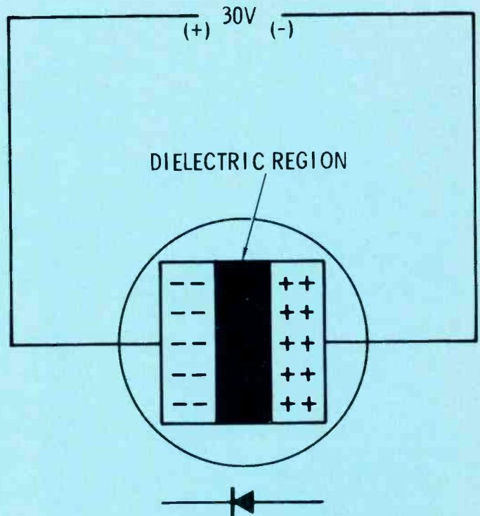
Fig. 2 Varactor diode with high reverse bias.
