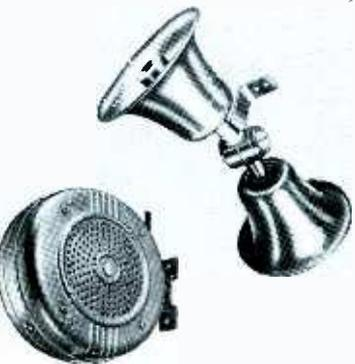
Paging speakers can also serve as microphones. Frequency response may be broad enough to permit use in combined intercom and background-music systems. Power ratings vary from 5-40 watts—depending on size. Most are single re-entrant horns, but special units may be used for bi-directional coverage.
