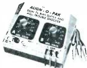
The SENCORE Model BE113 "Align-o-pak," a dual version of the Model BE3, is designed to supply two individually-variable negative DC voltages for AGC clamping and similar applications. The output from each section of this AC-powered unit ranges from 0 to 20 volts with less than 0.1% ripple. Dealer net price is \$12.75.
