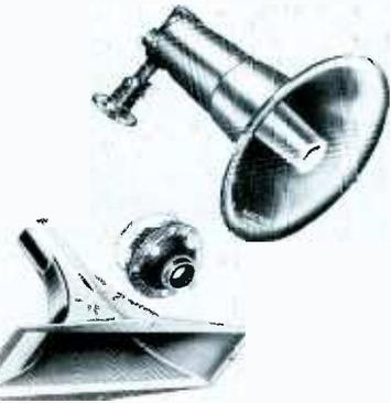
Many horns used in public address applications are two-piece units, with the voice coil and magnet housed in a detachable driver. However, one-piece horns are gaining popularity because of advantages such as lower price. Both integrated and two-piece types have similar electrical ratings—for example, outputs of 10-100 watts and frequency response of 75-7000 or 100-10,000 cps.
