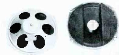
Speakers used in aircraft applications must be light in weight and compact in size. Most have a 30-ohm voice coil and are moistureproofed to guarantee long service. Types with 3-5 watt output, used as intercoms between crew positions, replace separate microphones and conventional speakers to save weight.
