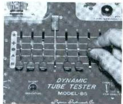
Fig. 9. Tube-element levers are moved up one at a time to check for shorts.
