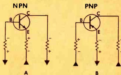
Fig. 2. Voltage drops caused by current flow in NPN and PNP transistors.
