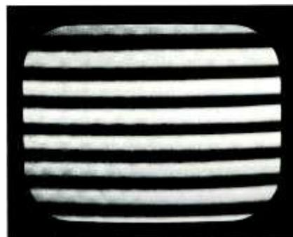
Fig. 3. Precision's square-wave generator produces these bar patterns on CRT.
