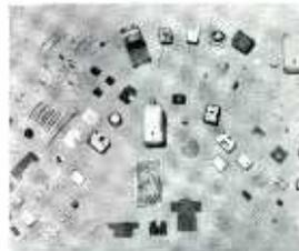
Sonotone's new super-sensitive transistorized hearing aid, weighing only 1/2 oz. with battery, and measuring 1/2" x 11/16" x 1 1/4", contains 153 parts in only a half cubic inch of space. Known as the Model "66," the miniature aid is powered by a 70-hour aspirin-sized battery that sells for about 35¢, and provides amplification of 10,000 times even at temperatures of 120° or more.
