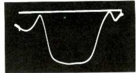
Fig. 3. Overloading produces deceptively flat bottom on response curve.
