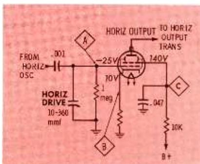
Fig. 1. Loss of horizontal drive signal is usual cause of "red-hot" tube.
