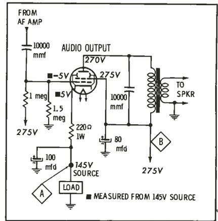
**Fig. 2. Overloaded low B+ line may cause red glow at audio-output plate.**
