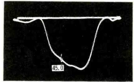
Fig. 6. If marker output is properly adjusted, pip will appear as shown.
