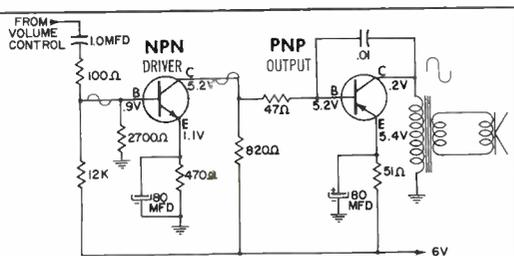
Fig. 6. Circuit using both NPN and PNP transistors is ideal for analysis.
