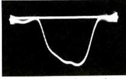
**Fig. 8. Radiation from horizontal sweep circuit causes "hash" on curve.**
