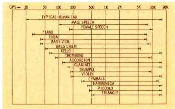
Fig. 2. Musical instruments produce many harmonics, some extending to or beyond the upper limit of human hearing.
