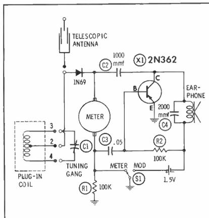
Fig. 6. Complete schematic of Model FS-3 reveals its transistor stage.
