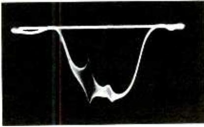
**Fig. 7. Excessive output from marker generator seriously distorts curve.**
