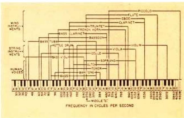
Fig. 1. The fundamental frequencies of most musical notes lie within the relatively narrow range of 40-4000 cps.
