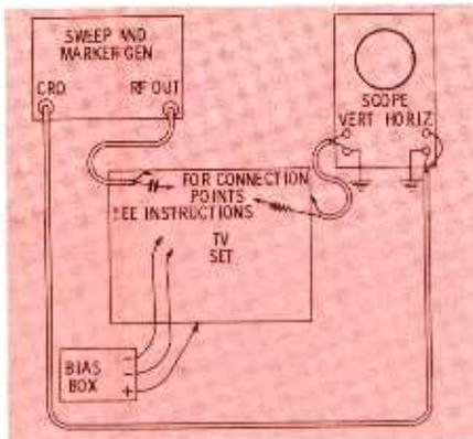
Fig. 2. Basic test equipment hook-up for performing a sweep alignment.
