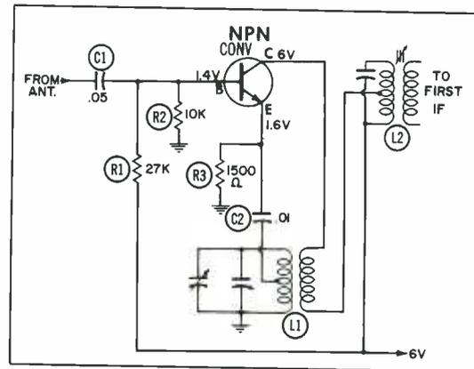
Fig. 5. Tuning gang must be rotated in order to check oscillator voltage. significant, and so our readings must be accurate.
