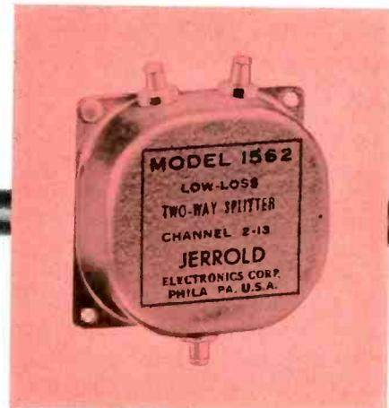
In the distribution lines running from the amplifier to the various receivers, splitters are used to divide main lines into additional branches. Minimum signal attenuation and maximum isolation are the important characteristics of these units.
