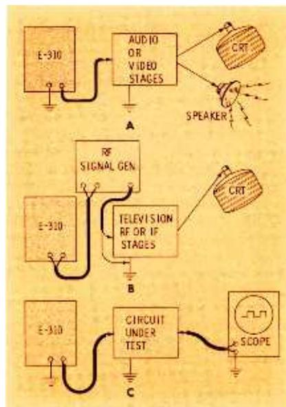
Fig. 2. Basic arrangements for signal-tracing with Model E-310 Generator.
