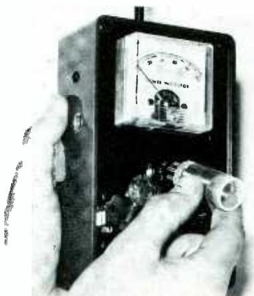
Fig. 5. Tuning coils for Model FS-3 plug into socket on the front panel.
