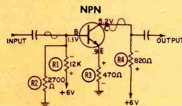
Fig. 3. NPN emitter and collector voltages follow pattern similar to tube.
