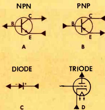
Fig. 1. Electron flow in NPN and PNP transistors, crystal diode, and tube.
