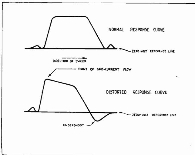
FIG. 7. Normal and distorted response curves. The undershoot distortion in the i-f curve is caused by grid-current flow in the first amplifier stage.
