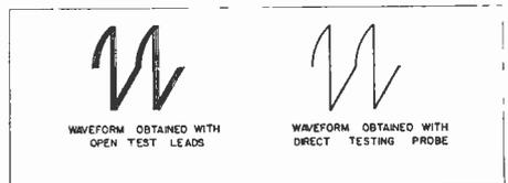
Fig. 10. The direct testing probe with its shielded coaxial cable avoids stray field pick-up.
