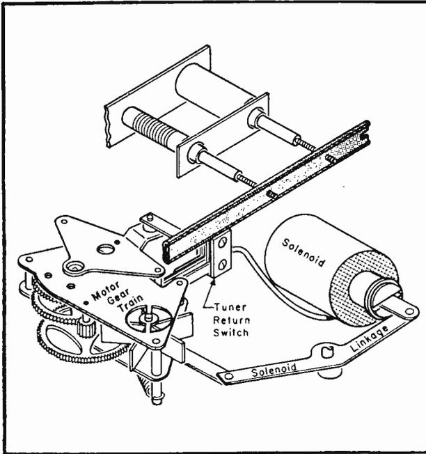
Figure 1B. Search tuners mechanical arrangement.
