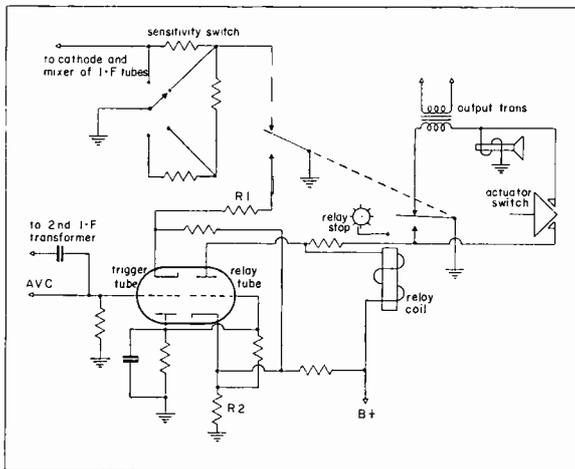
FIG. 3. Typical search tuner-spring motor.
