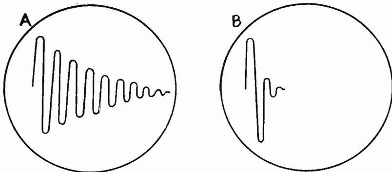
Fig. 1. Waveform produced by a good component, A; and waveform produced by a defective component, B.
