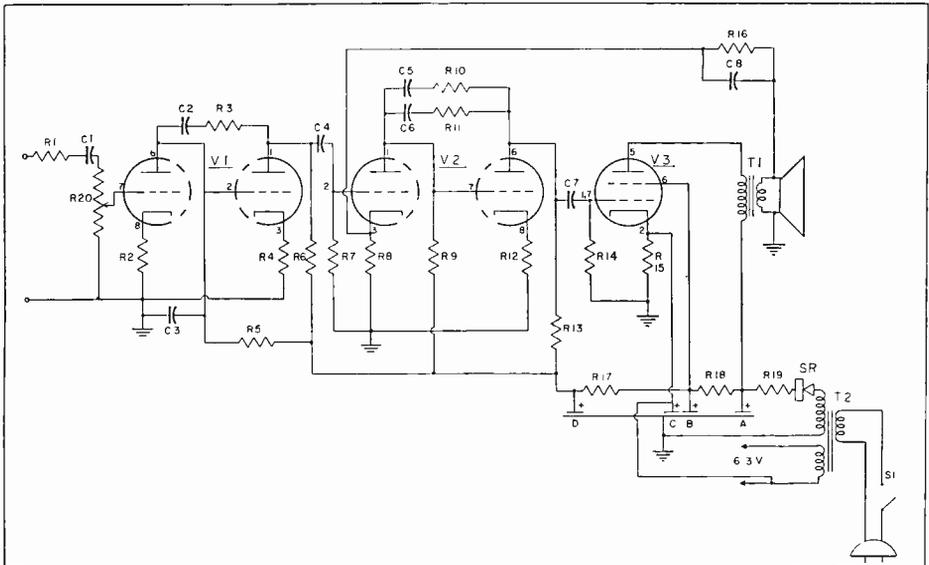
Fig. 3 Schematic diagram of the Synthetic Stereo amplifier.
