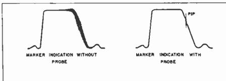
FIG. 9. The operation of a resistor-isolated probe.
