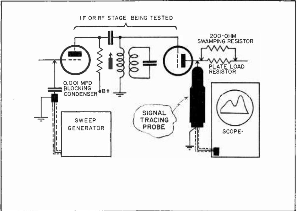
FIG. 8. Test set-up for checking single stage response using a demodulator probe.
