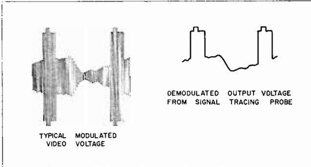
FIG. 5. The basic demodulation or detection operation of a crystal probe. Since the RF or I-F carriers are almost invariably too high in frequency for direct application to general-purpose scopes, the crystal probe rectifies the modulated carrier and transmits only the modulation information to the scope input.
