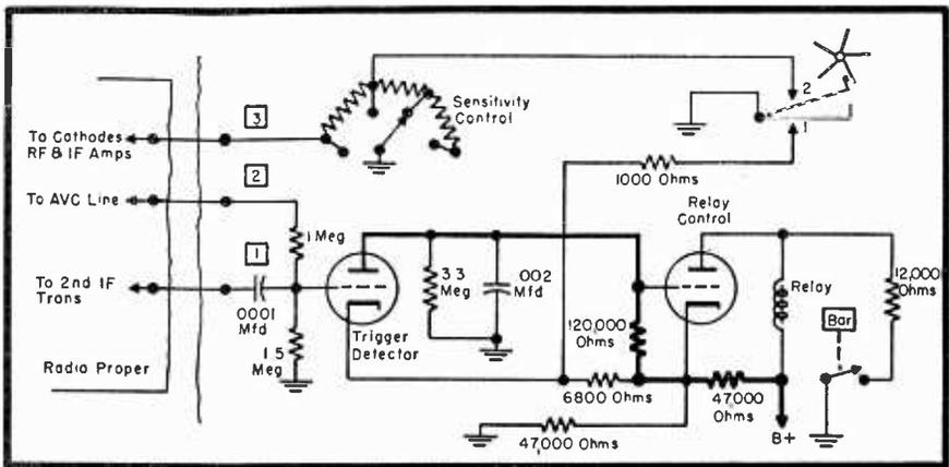
FIG. 2. Signal-seeking tuning circuit.
