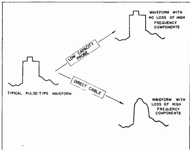
FIG. 4. Basic operation of a low-capacity probe.
