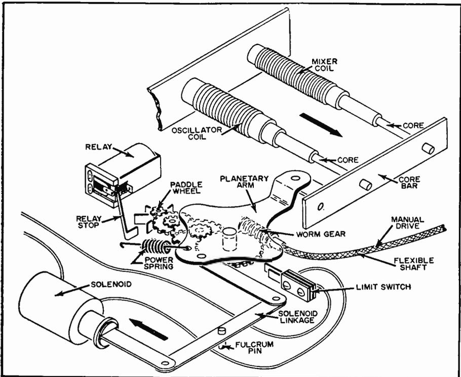
FIG. 1A Search tuners-mechanical arrangement.
