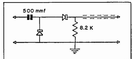
FIG. 6. A voltage-doubler type demodulator probe.
