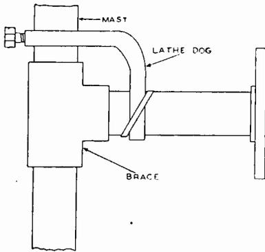
Fig. 4. A lathe dog on the bottom brace makes a very fine lock for the mast.
