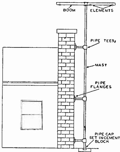
Fig. 3. The bottom of the mast rests in a pipe cap in a cement block. The over-size pipe tees form the bearings and the mast is free to rotate. The braces are fastened to the side of the house or the chimney.
