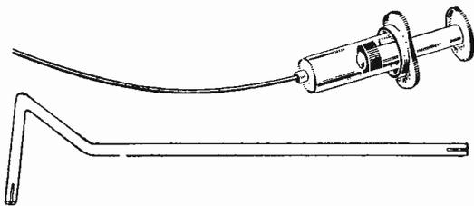
Fig. 7. (above) Hypodermic type injector, offered by Walsco; (below) Contact Adjuster, offered by several companies, including the General Cement Company, Rockford, Ill.
