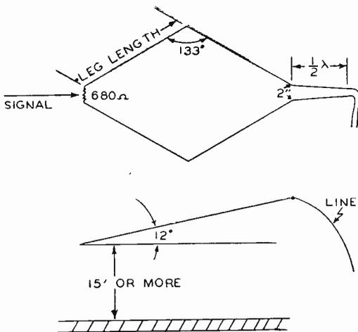
Fig. 8. Rhombic Type Antenna.
