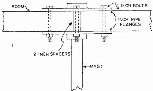
Fig. 5. The mast is attached to the boom by means of two pipe flanges and four bolts. The two-inch spacers are made from short pieces of the aluminum tubing.
