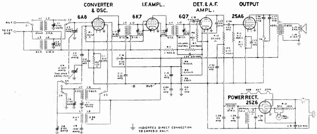
Fig. 6. G-E A-54 Circuit Diagram.
