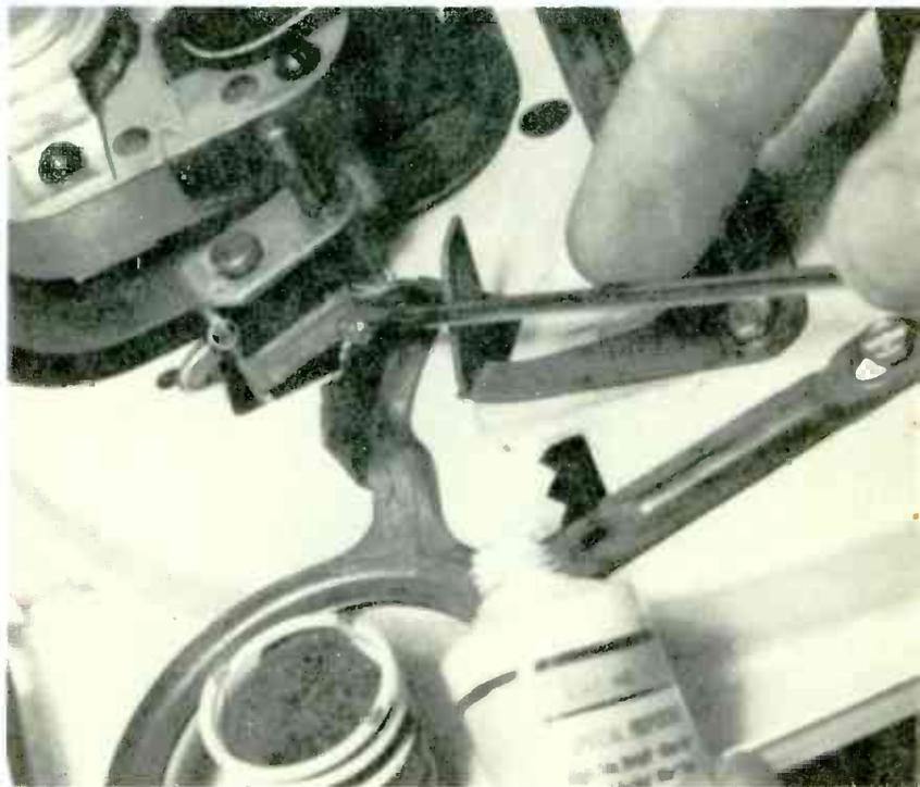
Figure 10. With the changer turned off, turn it over so you can inspect the sliding mechanical parts on the underside. Apply a small amount of non-hardening grease to all sliding surfaces which appear to transfer any amount of force.
