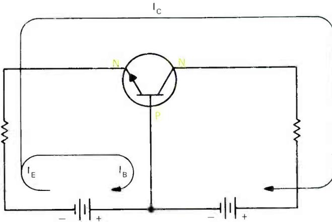
FIGURE 1. PROPER BIAS FOR AN NPN TRANSISTOR.
