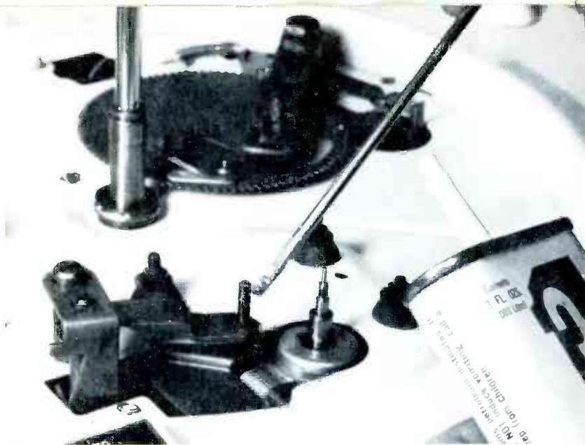
Figure 7. Clean both the hole in the idler wheel and the shaft on which it revolves with your tuner cleaner and then lightly oil both the shaft and the hole in the wheel. Re-install the idler wheel and the "C" clip and spin the wheel to make sure it turns freely.
