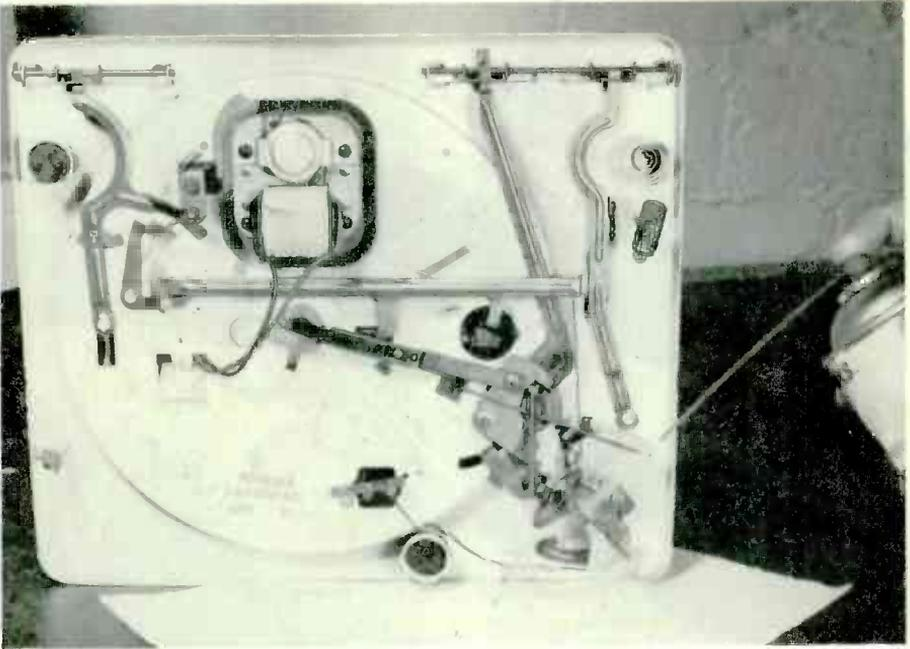
Figure 4. With most of the dirt removed, spray the moving parts with a tuner cleaner and lubricant to remove any deep-down dirt and lint. This will also remove caked grease if done properly.
