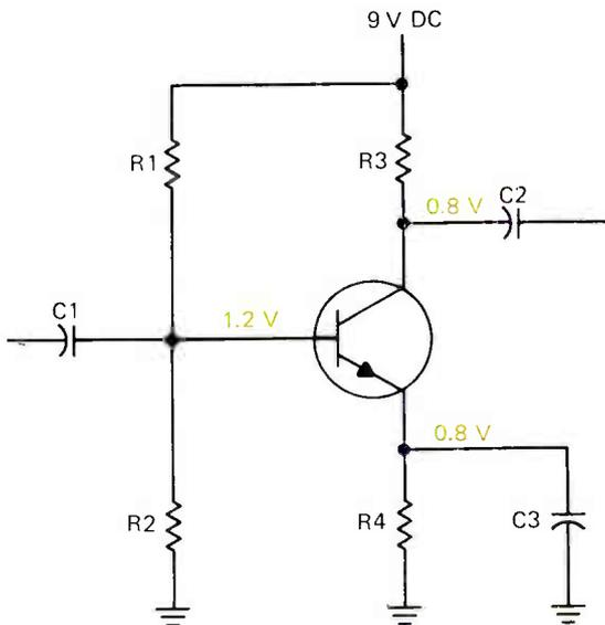
FIGURE 3. A SATURATED TRANSISTOR.
