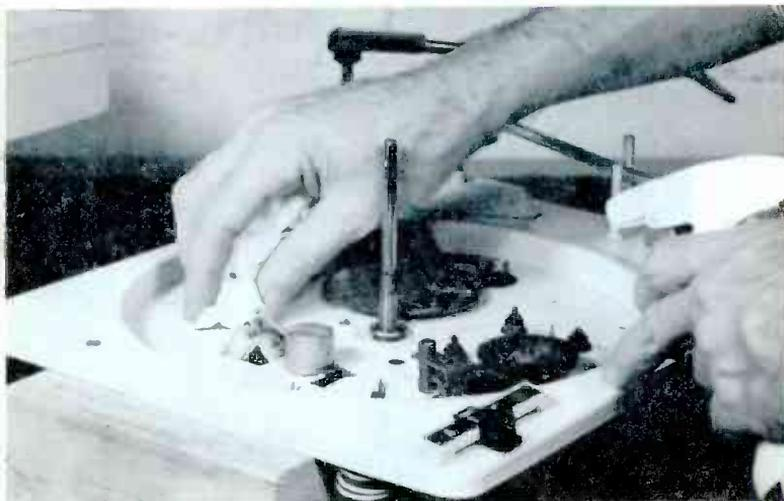
Figure 5. Now go over the top side of the changer with the spray detergent and a paper towel. Do the entire top of the changer base and the tone arm itself. This won't make the changer work any better, but the customer will surely appreciate the neat, almost-new look the cleaning will impart to the machine.
