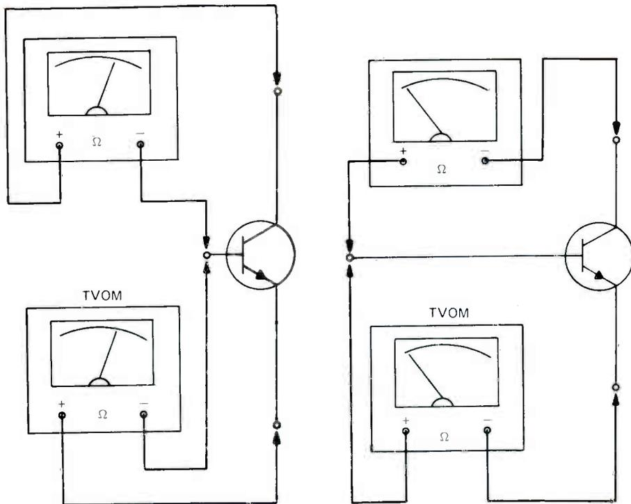
FIGURE 6. HOW TO TEST A TRANSISTOR WITH A TVOM. (L.) REVERSE BIAS, HIGH RESISTANCE. (R.) FORWARD BIAS, LOW RESISTANCE.
