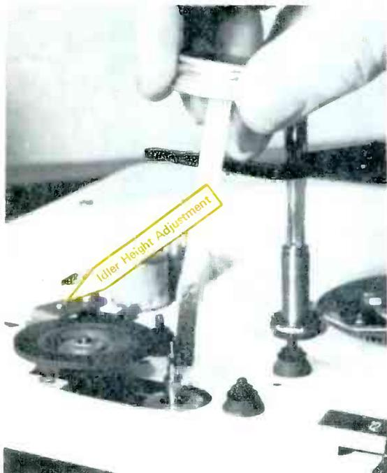
Figure 9. With the motor back together again and running smoothly, apply a small amount of Chemtronics Non-Slip to the surfaces of the driving pulley and to the idler wheel. Do this with the motor running. Now run the speed change lever through its positions and check to be sure that the idler wheel sits squarely in the middle of each step of the driving pulley. If it does not, adjust the idler height screw with a screwdriver.
