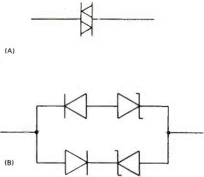
FIGURE 8. (A) DIAC SYMBOL. (B) EQUIVALENT CIRCUIT.
