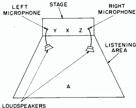
FIG. 1. Basic stereo system.
