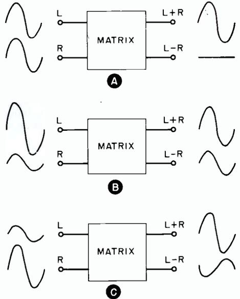
FIG. 3. Matrix input and output signals when (A)  $L$  is equal to  $R$ , (B)  $L$  is greater than  $R$  and (C) when  $R$  is greater than  $L$ .
