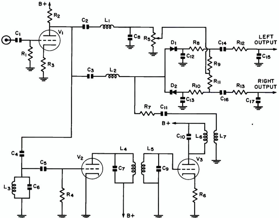
FIG. 8. Simplified schematic of multiplex adapter circuit.
