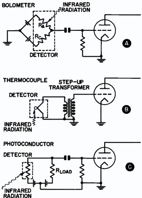
FIG. 4. Thermistor bolometer detector.
