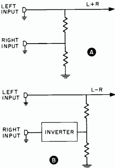
FIG. 2. Simplified matrix circuit.
