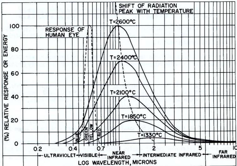
FIG. 1. The Visible and Infrared Spectrum.
