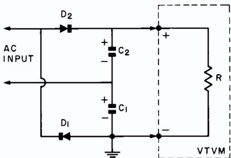
FIG. 6. Peak-to-peak probe for vtvm's.
