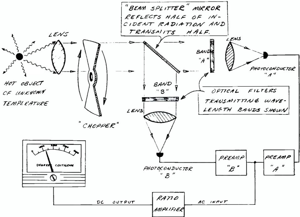
FIG. 9. Simplified color pyrometer.
