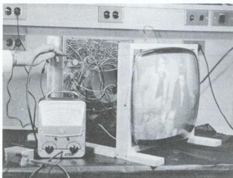
FIG. 7. Measuring peak-to-peak drive to CRT with special probe and Model 211 vtvm.
