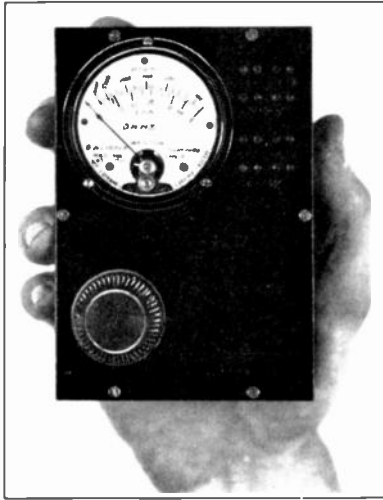
A 2-range ohmmeter by G. H. Cooper. With a self-contained one-cell battery it gives useful ranges of 1 to 100 and 100 to 10,000 ohms. The upper tip-jacks are the ones labelled A and B in the diagrams and are for the high (series) range. The two lower jacks are for the low (shunt) range, the shunt circuit being made by the split jack D, as shown in the diagrams. The knob at the lower left is the clarostat used to effect zero compensation.
