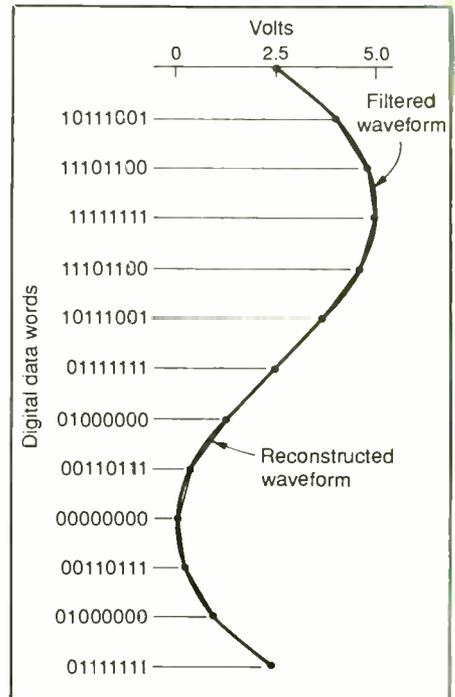
Fig. 11. An analog filter at the output smoothes out the sudden changes in the DAC's converted waveform to improve the quality of the regenerated audio signal.
