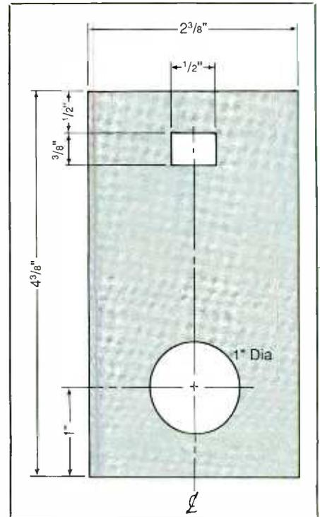
Fig. 4. Fabrication details for front panel of specified enclosure. If you use an enclosure that has different dimensions, make suitable adjustments in machining details.
