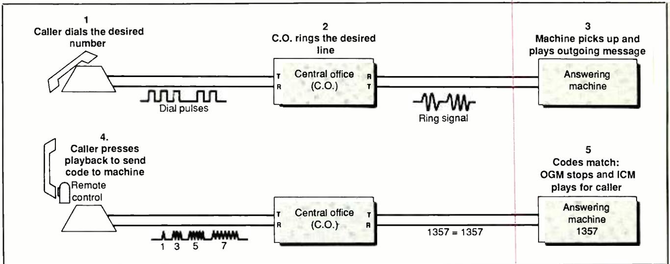
Fig. 7. When using remote control, the answering machine resets the outgoing message tape, rewinds and plays the incoming-message tape, and transmits any recorded messages back to the calling party.
