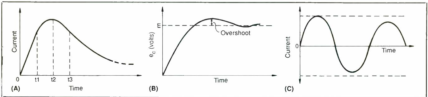
Fig. 6. Square-wave overshoot and ringing modes: (A) critical damping where  $Q$  is 1 and overshoot is a single surge; (B) where  $Q$  is slightly greater than 1 and overshoot is followed by a half-cycle of ringing; (C) where  $Q$  is comparatively high and overshoot is followed by a substantial ringing sequence.
