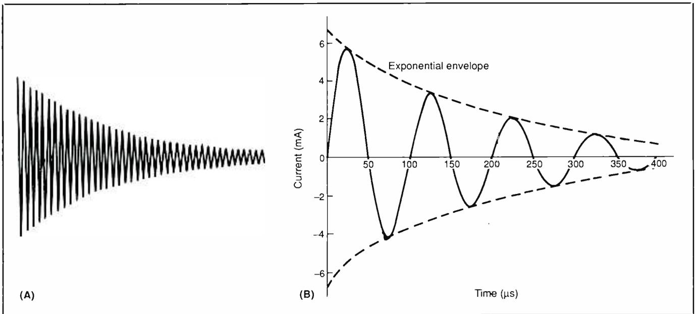
Fig. 2. Example of a ringing waveform with exponential decay. (A) is the pattern of the waveform as it would appear on the screen of an oscilloscope; (B) is the graphed plot of the waveform parameters versus time.
