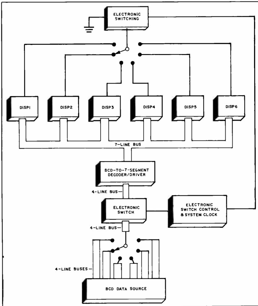
Fig. 1. Block diagram of the subsections that make up the project.
