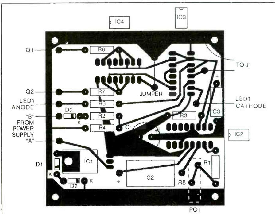
Fig. 4. Component-placement guide for pc board.
