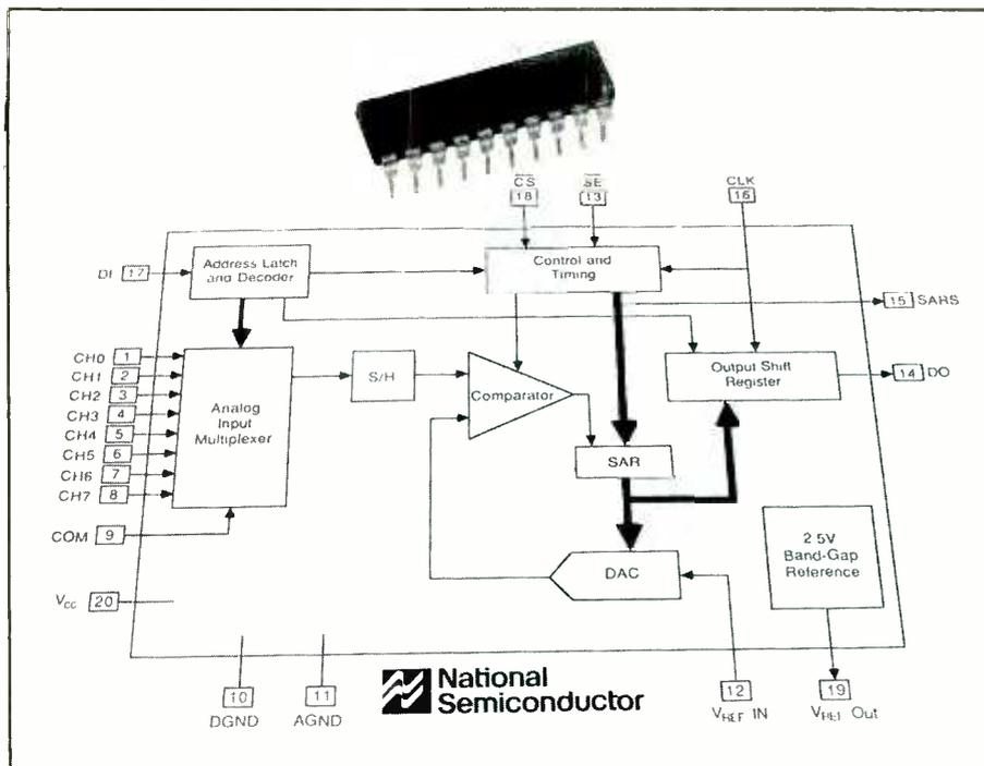
Fig. 3. National Semiconductor's ADC080xx A/D converter series include on-board reference, multiplexer and track-and-hold functions.
