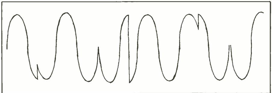
Waveform of phase-shift-keyed (PSK) modulation.
