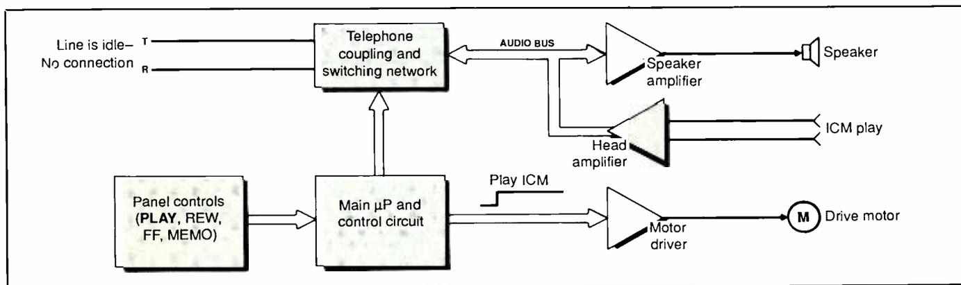
Fig. 6. Buttons on an answering machine permit the incoming-message tape to be manipulated as in any other audio cassette recorder in the play mode.
