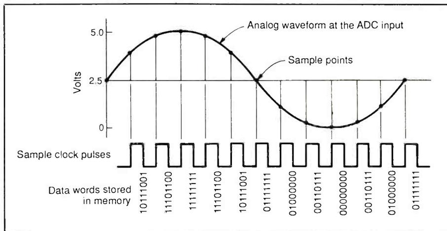
Fig. 9. An example of an analog waveform (upper) and its pulse equivalent and data word codes (lower) after digital conversion.
