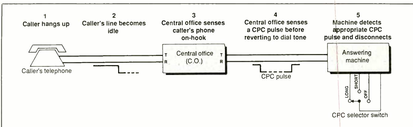
Fig. 5. The CPC switch usually offers a choice of pulse-duration and "off" positions to accommodate differences in Central Office equipment.
