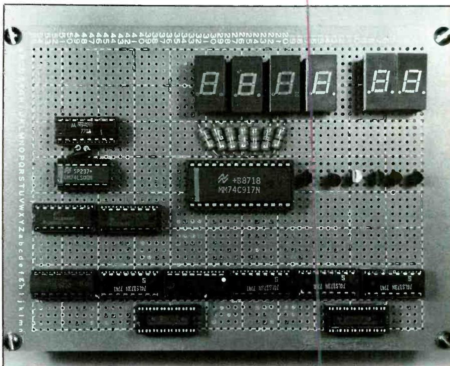
switched, four bits at a time, by the Electronic Switch to a BCD-to-7-Segment Decoder/Driver. This section decodes the binary data to hexadecimal format and routes it to the appropriate decade in the display string (DISP1 through DISP4). Finally, the proper segments of the appropriate display decade must be turned on, which is accomplished with another Electronic Switch under control of the Electronic Switch Control & System Clock block.
