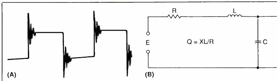
Fig. 5. Example of ringing reproduced square wave with rapid decay interval: (A) as it would appear on the screen of an oscilloscope; (B) rapidly of decay depends on the Q value of the equivalent RLC network.
