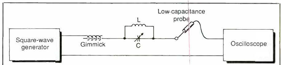
Fig. 1. Test setup that minimizes circuit loading for displaying a ringing waveform.
