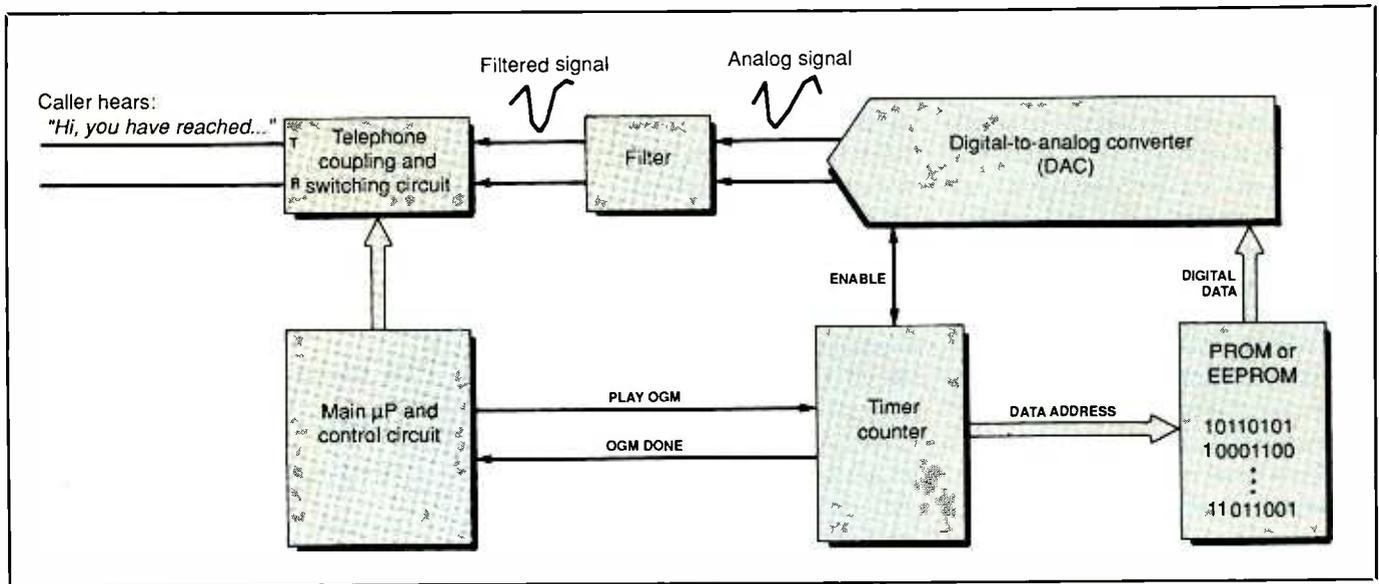
Fig. 10. To generate the outgoing message, a DAC in the voice synthesizer converts EEPROM data into analog form for transmission over the telephone line.
