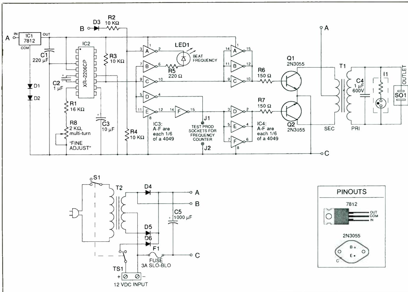
Fig. 2. Complete schematic diagram of Tide Clock electronic drive circuitry.
