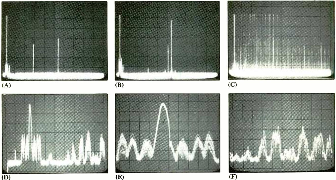
Fig. 3. Spectrum Probe oscilloscope displays showing: (A) simultaneous 27- and 49-MHz CB transmitter carrier signals; (B) two closely spaced signals of a cordless telephone system; (C) broad-spectrum noise produced by dc motor; (D) expanded view of index marker and received local AM radio station; (E) highly expanded view of index marker generated by Spectrum Probe; and (F) expanded portion of trace showing signal from AM radio broadcast-band stations.
