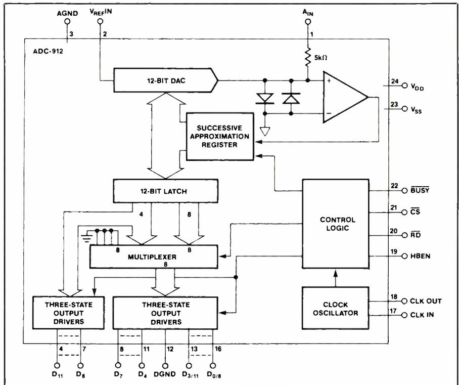
Fig. 1. Precision Monolithics' ADC-912 A/D converter offers successive-approximation conversion.
