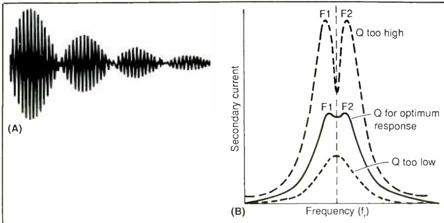
Fig. 4. Example of a ringing waveform for a tuned i-f transformer illustrating the effect of two ringing frequencies: (A) as it would appear on the screen of an oscilloscope; (B) graph of ringing frequencies F1 and F2.
