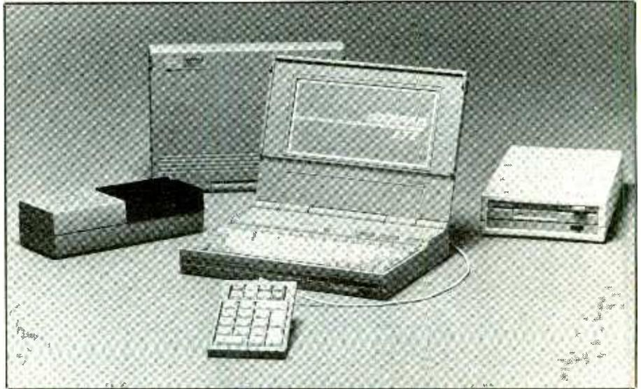
Compaq's LTE notebook computer comes in two versions: the PC compatible 8086 LTE and the 80286 286/LTE versions. Key options include (left to right) external Fast Charger/ac Adapter, numeric keypad and 5 1/4-inch floppy-disk drive or 40-MB hard disk.
