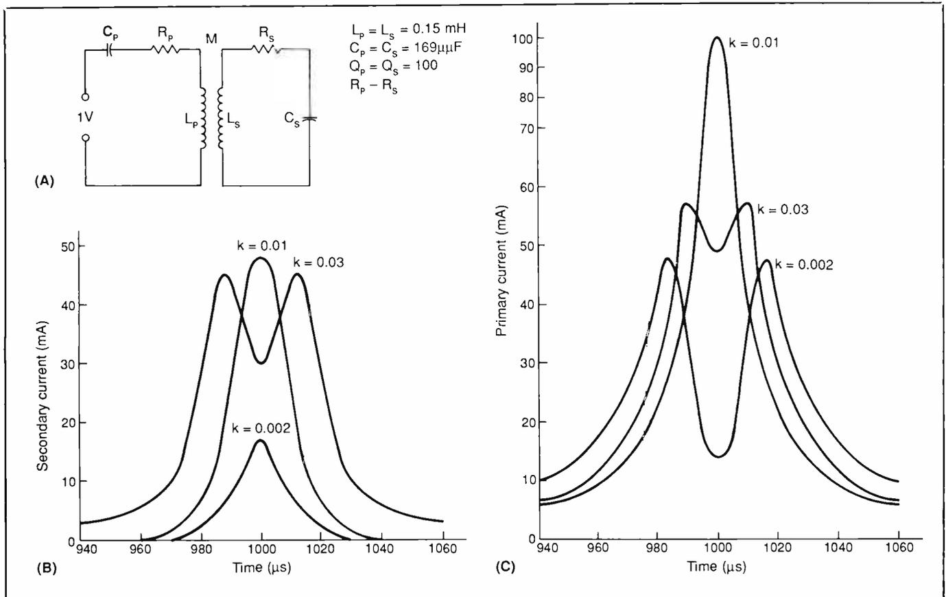
Fig. 3. Details of an AM i-f transformer: (A) Thevenin representation; (B) plots of primary signal-current flow of three degrees of coupling; (C) plots of secondary current flow of three degrees of coupling.
