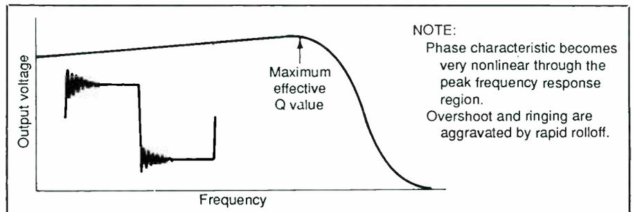
Fig. 7. Plot of an RC amplifier that has rising high-frequency response is equivalent to a basic amplifier plus an RLC peaking network that has a moderately high  $Q$ .
