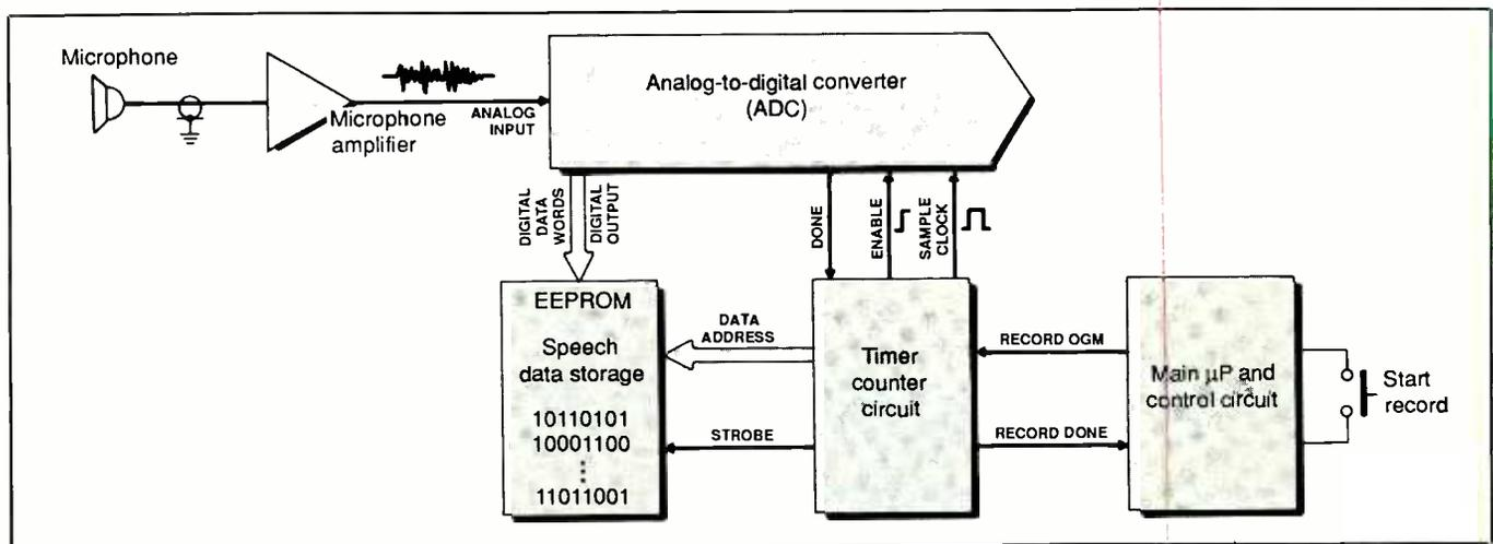
Fig. 8. One possible approach for assembling a voice digitizer/recorder.
