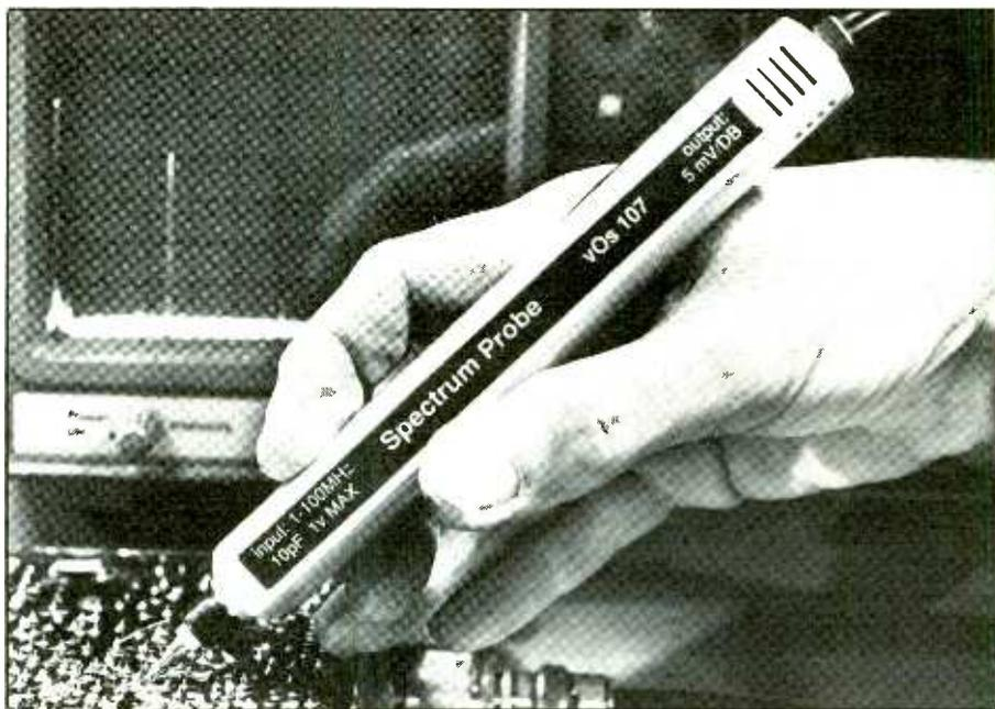
Fig. 1. The Spectrum Probe spectrum analyzer in operation with an oscilloscope.
