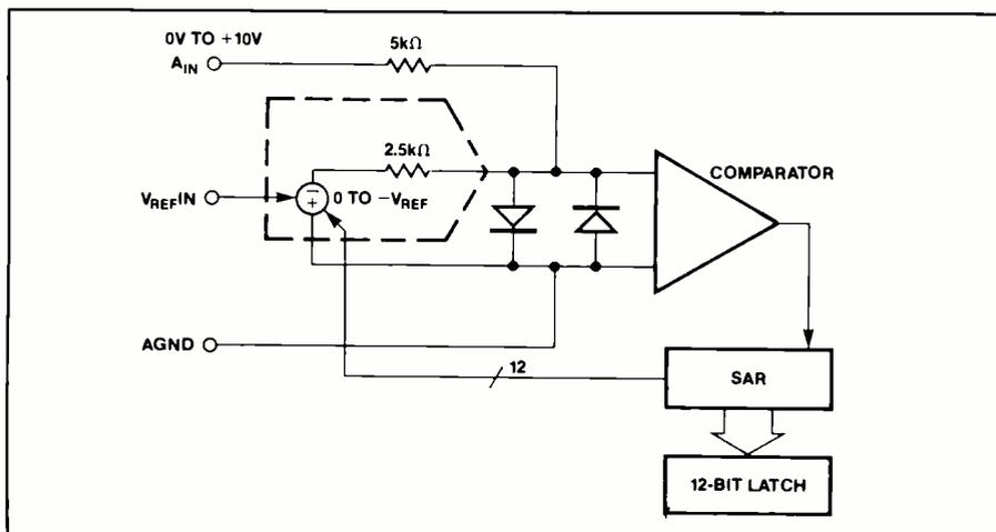
Fig. 2. The ADC-912 has a 2,500-ohm input resistor that connects to the same comparator input as the external 5,000-ohm resistor that couples the input signal into the device.
