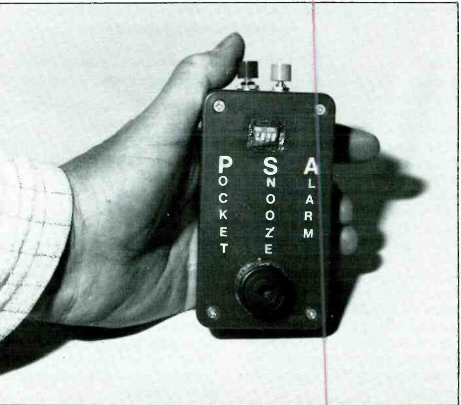
*R4*, depending on which is selected by *S2*, and capacitor *C1*. With the values specified for *R1* through *R4*, snooze periods of approximately 5, 10, 15 and 30 minutes, respectively, are available with the 470-microfarad value specified for *C1*.
