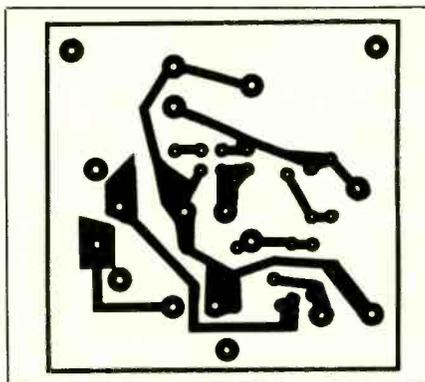
Fig. 2. Actual-size etching-and-drilling guide for receiver's printed-circuit board.
