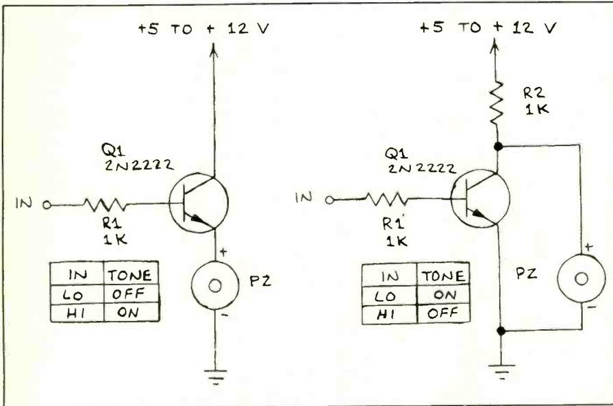
Fig. 6. Piezoelectric buzzer logic interfaces.
