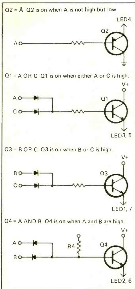
Fig. 3. The logic expressions and electronic equivalents for each driver transistor.
