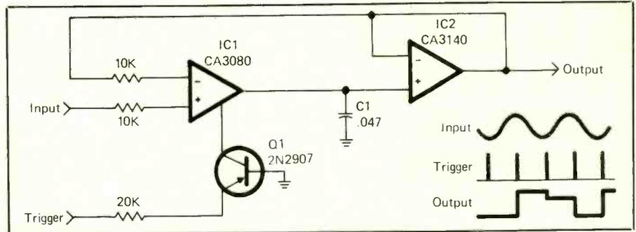
Fig. 5. A typical OTA sample/hold circuit.
