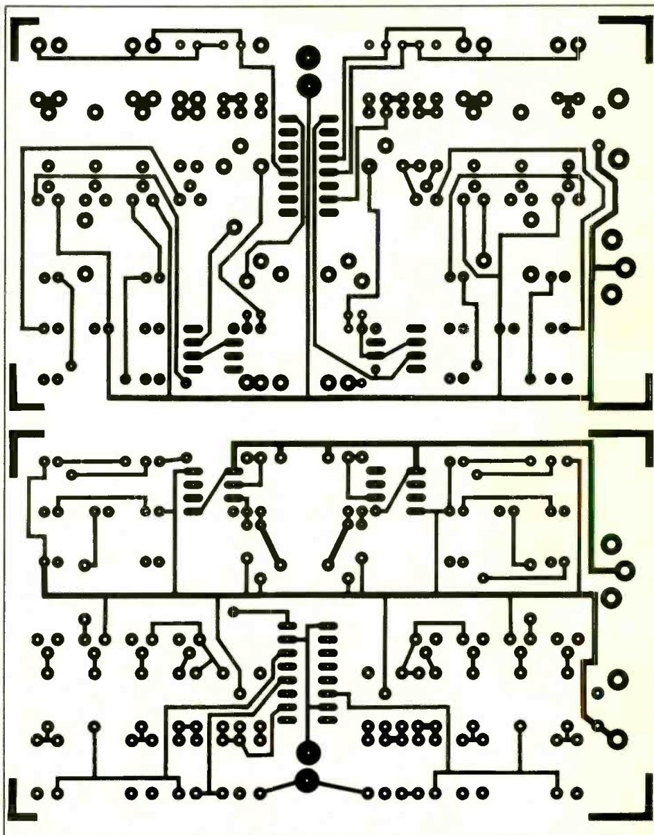
Fig. 4. Actual-size etching-and-drilling guides for both sides of printed-circuit board.
