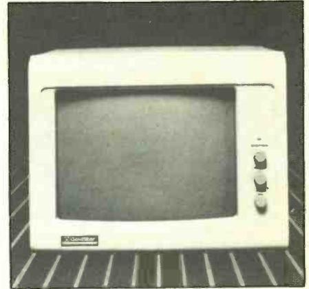
which makes it compatible with any computer that has a composite output. Additional features include power, brightness and contrast controls. The MBH-2003 measures 13.8"W x 12.6"H x 10.9"D. \$185.
