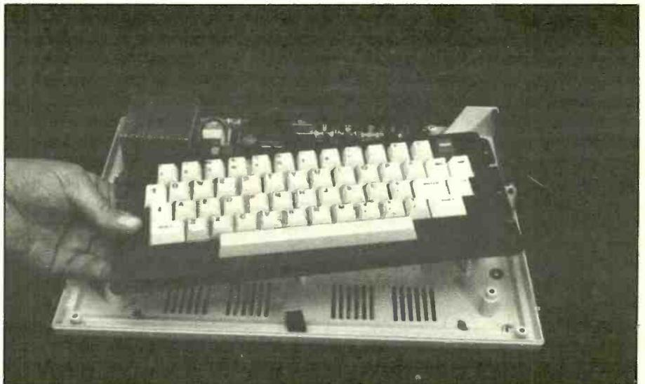
To remove the keyboard, lift it straight up and gently flip it back to the rear.
