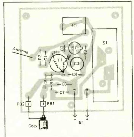
Fig. 3. Components-placement/orientation diagram.
