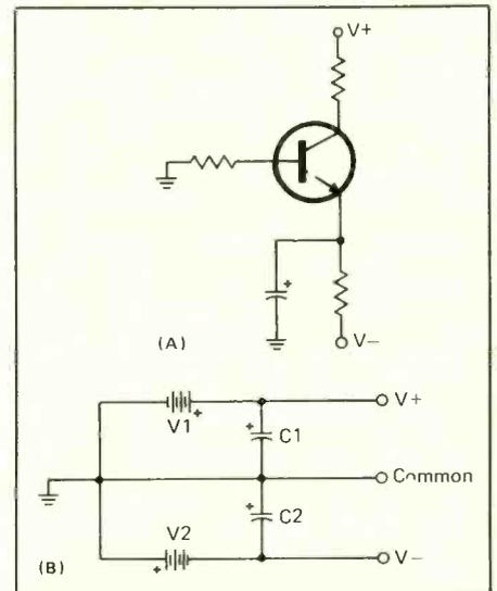
Fig. 2. An amplifier biased for dual-polarity power supply operation (A) and a typical dual-polarity power supply (B).
