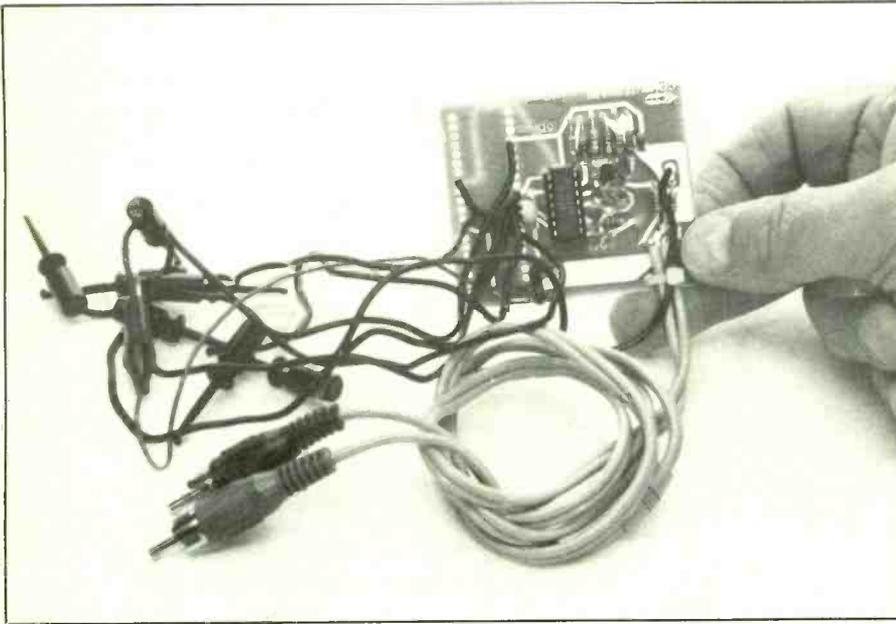
*Interconnects from the small commercially available video adapter board connect to the CoCo via wires terminated in mini-clips. The two cables terminated in phono plugs are the new video and sound outputs.*
