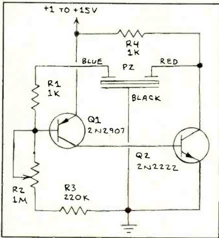
Fig. 9. Adjustable-frequency piezoelectric buzzer element driver.
