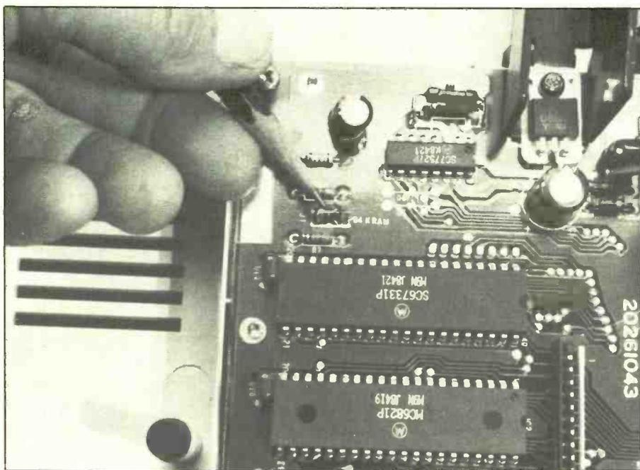
*Program the CoCo to address 64K of RAM by soldering a wire across the two “64K” solder pads located at the upper-left of the motherboard.*
