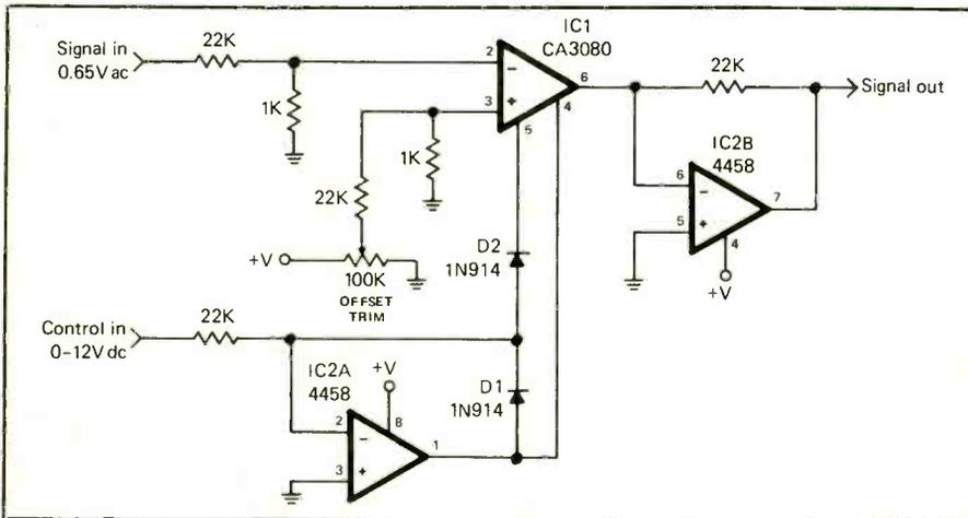
Fig. 3. Improved voltage-controlled amplifier uses ordinary operational amplifiers as a voltage-controlled circuit source and an output buffer.
