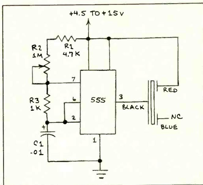
Fig. 12. Piezoelectric buzzer element driver built around 555 timer.
