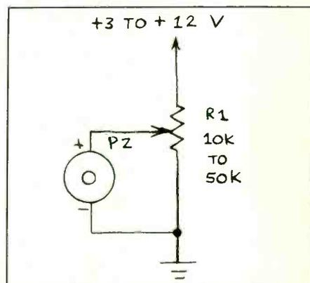
Fig. 4. Controlling the volume of a piezoelectric buzzer.
