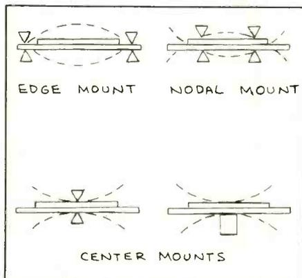
Fig. 3. Mounting arrangements for piezoelectric buzzer elements.
