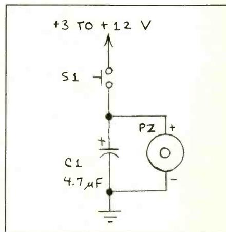
Fig. 5. Achieving a bell-like sound from a piezoelectric buzzer.
