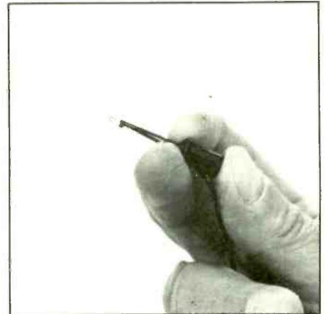
*The display board's mini-clips provide a secure connection when the spring-loaded "body" is released.*
