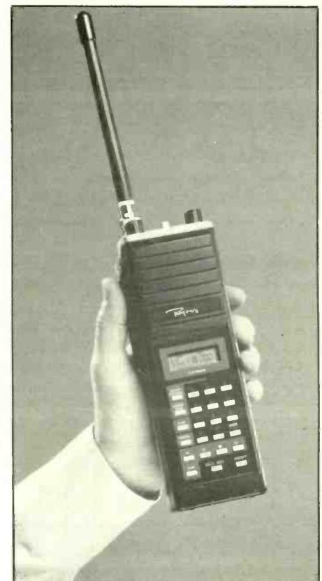
nel banks. Designed to compete in versatility with basestation units, it is claimed to offer more channel capacity than any other scanner on the market. Band coverage includes 10-meter Amateur; vhf low; vhf AM; vhf/AM Aircraft; Space Research; vhf Amateur; vhf high; Federal and Government Land Mobile; uhf Amateur; uhf; and uhf-T.
