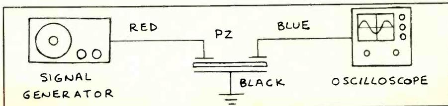
Fig. 13. Using a piezoelectric buzzer element as an audio signal filter.
