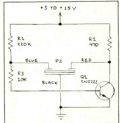
Fig. 7. Single-transistor piezoelectric buzzer element driver.
