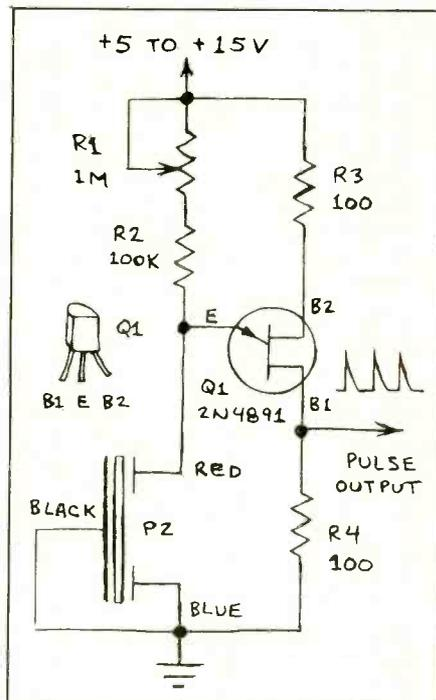
Fig. 10. Unijunction transistor piezoelectric buzzer element driver.
