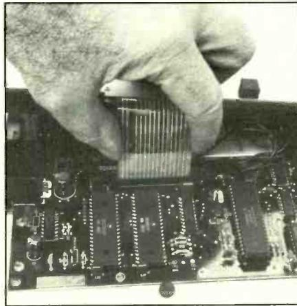
*Do not grip the keyboard's ribbon cable as shown to unplug it from the motherboard; it might be damaged. Instead, grip it on both sides between thumb and forefinger and lift straight out.*
