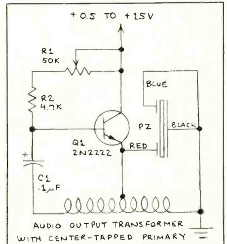
Fig. 8. Hartley oscillator piezoelectric buzzer element driver.
