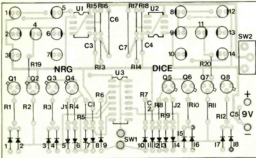
Fig. 5. Components placement/orientation diagram for pc board.
