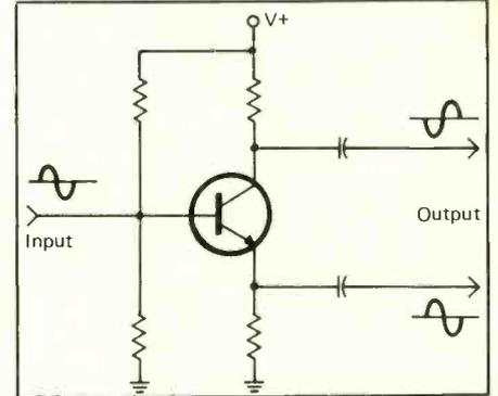
Fig. 8. A transistor phase inverter is one possible replacement for the interstage (input) transformer needed for the opposite-polarity driving signals for the two halves of the push-pull amplifier circuit.
