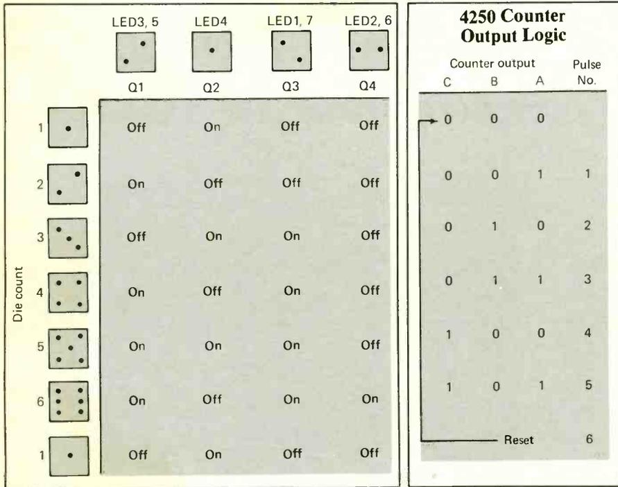
Fig. 2. Conditions for each driver transistor for specific die counts.
