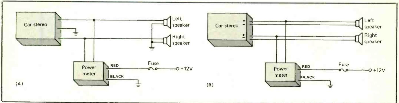
Fig. 7. Power Meter can be connected into conventional grounded (A) and floating ground (B) systems.
