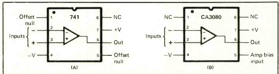
Fig. 1. Pinouts of the ordinary 741 op amp (left) and CA3080 operational transconductance amplifier (right). Though both appear to be identical, note that the 741 has offset null, while the CA3080 has a bias input.
