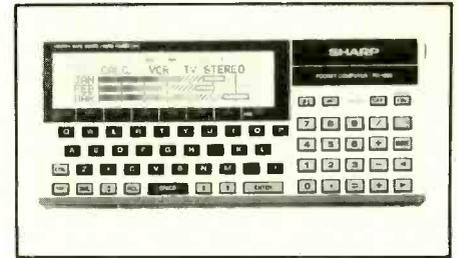
Featured are: 16K of RAM (expandable to 80K); a 4-line by 26-character LCD display; the fiber-optic interface; an analog input; an RS-232C serial interface; separate alphabetic keyboard and numeric keypad; a 60-pin I/O bus; and BASIC interpreter in ROM. Options include the microfloppy drive with 128K capacity; a 4-color pen plotter/cassette interface and a 32K RAM module. The computer measures 8"L x 3.5"W and weighs less than 1 lb. \$345.
