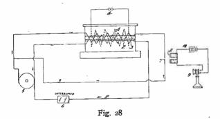
An arc light 7 is introduced in series in the primary 3, and the current flowing through this primary in series with the arc light being a continuous one, generates an unvaried magnetic field which, owing to its steadiness, neutralizes the variations of the magnetic field of the primary 2 which are caused by the interrupter 6, and consequently no discharge takes place at the spark gap 4.
