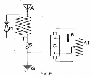
the spark gap will be varied by the impulses of the human voice energizing the electro magnet, and through its producing variations in the arc light and in the circuit in which it is located.
