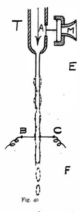
a sound of a given rate, such as a musical note, in the microphone, the water column is found to con-
