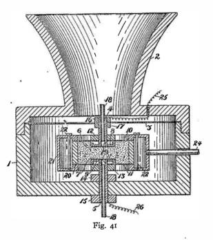
Referring to fig. 41, 1 indicates a casing of a telephone transmitter, and 2 the mouth piece thereof, screwed to the casing. and between which and the casing is clamped the main diaphragm 3, which is of metal, and of the usual construction.
