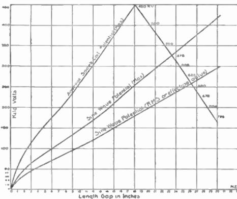
The spark gap method of measuring potential is preferred as its potential value is dependent upon the "maximum voltage," and is independent of wave form, and hence is a limit on the maximum electric stress to which an insulator is subjected, but the spark gap is not conveniently adapted for comparatively low voltages, say below 4,000-5,000.
