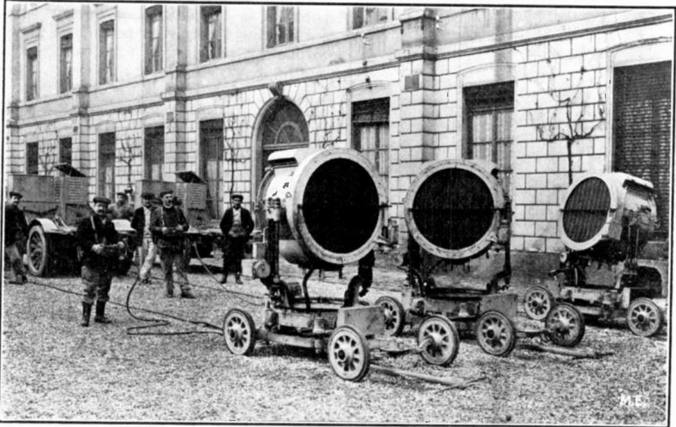
SEARCHLIGHTS ON GROUND READY FOR ACTION. NOTE CONTROLLING APPARATUS CARRIED BY OPERATORS
