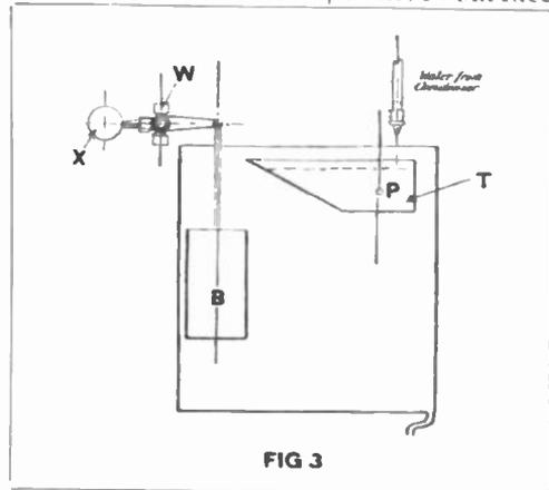
and hasten the evaporation, the receiver often has a coil of pipe connected with it. In many cases this coil is immersed in a tank of brine or other non-freezing solution. This brine acts as a store for a large quantity of cold and maintains a uniform temperature during time when the apparatus is not being worked.
