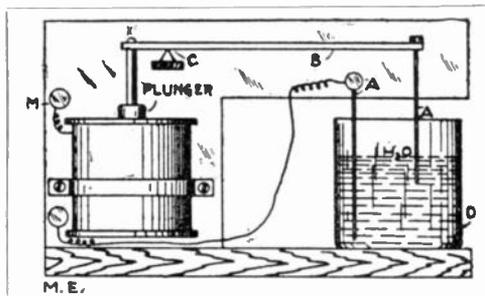
ting off the power before the amount wanted is being delivered, either reduce the number of turns in the solenoid or weight the arm, B. The regulation in any particular case is also aided by cutting off the wire, A, to the best length as indicated by experiment.
