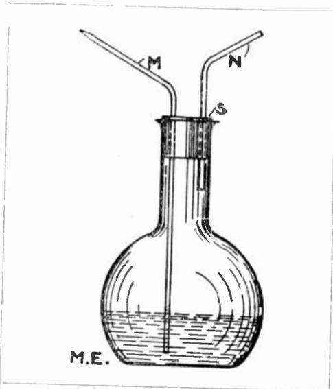
$\frac{3}{16}$  inch internal diameter are bent to the shape shown by M and N, these tubes being fitted into the holes of the stopper. The lower end of M reaches nearly to the bottom of the flask, while the lower end of N is about  $\frac{1}{2}$  inch below the bottom of the stopper. The upper end of M is drawn down until the opening is about  $\frac{1}{16}$  inch in diameter.
