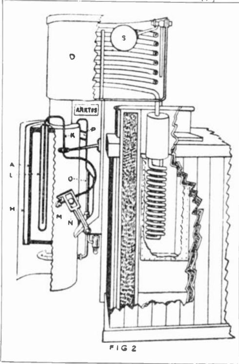
and requires no motive power. From the drawings it will be noted that the essential part of the device includes a combined absorber and generator (or still), a condenser and a receiver.
