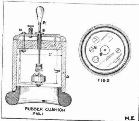
other for screw N. After cutting, drilling and bending a strip of  $\frac{1}{2}$  in. brass, as shown, the parts are ready to assemble, as shown in Fig. 1.
