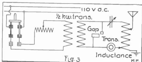
connected a 1/2 kw wireless transformer through some form of resistance for regulating the current when necessary. Across the terminals of the secondary of the transformer is a special form
