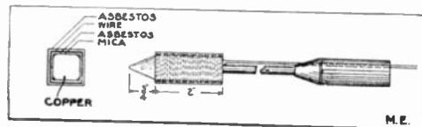
point. Over this are put four pieces of sheet asbestos the same size as the mica.
