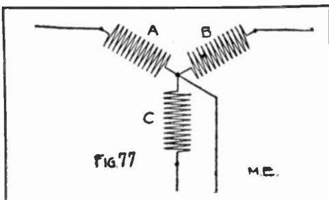
terminals of each winding are led out to separate collector rings. This style of connection is very rarely used, on account of the number of collector rings and brushes required.
