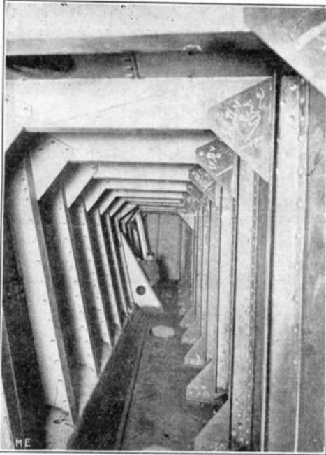
SPACE BETWEEN THE INNER AND OUTER SKINS OF THE DOUBLE HULL
