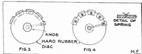
points and space these pieces of copper as far apart as a pair of switch points are. Then fasten on another piece of copper only one-half as wide so that it will only cover one switch point. But then continue this piece of copper right down to the centre of the disc so that it will make a connection with the bolt, which will fasten this disc to the secondary head, and from which one of the two wires of
