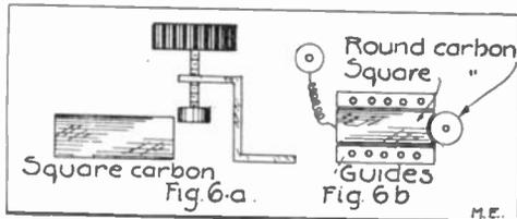
is round and filed flat on its sparking end. It is parallel with the upper face of the square carbon and should never be brought below the edge of the upper surface, Fig. 6a. The square carbon electrode is mounted so that it can slide forward toward the micrometer electrode, varying the distance between
