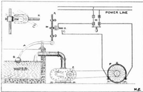
rises and falls with the water by means of a float B. As the water is used up arm A falls which in turn raises M (switch closing device) which closes switch K on contact C.
