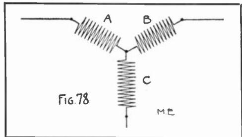
not be left out altogether, provided the loads on the three circuits are equal. There are then only three collector rings needed. This is often done, and the resulting winding, shown in Fig. 78, is commonly known as the "star," or "Y" winding for three-phase apparatus. It is used extensively when the load on each circuit is equal.
