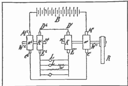
of Steglitz, near Berlin, Germany, in his Patent No. 1,059,076 is to obtain an approximately constant potential at the terminals of the working circuit irrespective of great variations in speed of the mechanically driven power shaft. To this end there is provided a second shaft and electrical means, consisting of one or
