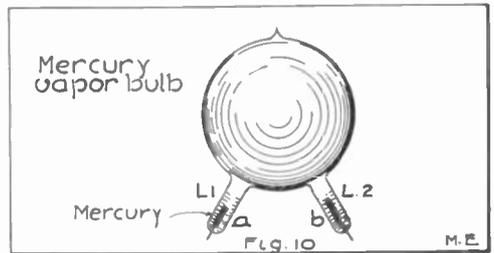
may be copper, silver plated, is mercury which comes nearly up to the top of the legs, L1 and L2. Wires that connect to the electrodes pass on to binding posts on the top of the wooden frame. The whole is then immersed in a can of transformer oil to keep the
