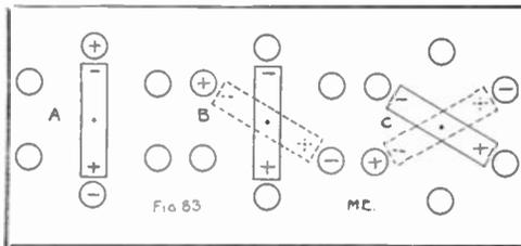
nets marked + and - at B. The armature retaining some of its magnetism will now tend to arrange itself in the position shown by the dotted lines. An instant later, the strongest field-magnets will again have changed, pulling the armature up a bit more, as at C; and this is carried on indefinitely.
