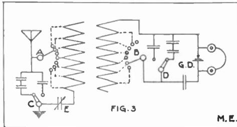
ground. Using the fixed condensers and the variable one high wave lengths can be reached and great selectivity can be obtained.
