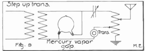
may be employed instead of the carbon spark gap, as indicated in Fig. 9. For cut of mercury vapor bulb see Fig. 8. Into a glass bulb of the form shown are sealed two silver electrodes, A and B, Fig. 10. The air is exhausted from the tube and it is mounted as in Fig. 11, to keep the bulb from being injured. Wooden discs are cut and large holes to fit the bulb are made to hold it in place and in an upright position. Around the silver electrodes, which
