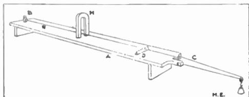
means of a pendulum. The following method makes use of the tone emitted by a vibrating string and the fact that a conductor in which a current is flowing tends to move in a direction at right angles to the lines of force when placed in a magnetic field.
