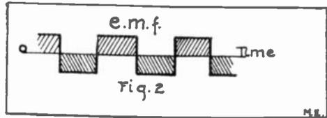
force or current, its "effective value" is invariably understood, unless expressly stipulated otherwise. This effective value is the equivalent of the direct current which would produce the same heating effect in the circuit.
