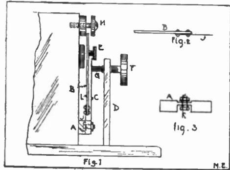
dle. The only other thing which needs explanation is H, which is a machine screw with rubber washers. These washers not only reduce the noise, but by their elasticity also increase the speed of vibration.
