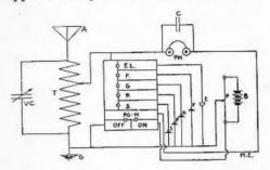
"Electrolytic." This connects that detector in circuit. Now to connect the potentiometer, place the second plug between the plates "potentiometer" and "on." When not in use the plugs may be kept in the holes in the blank plate, provided for that purpose.
