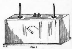
On top of cabinet should be screwed three pieces of polished hard rubber, one piece 6 by 2 by 3/8 inches and the other two should be 3 by 3 by 3/4 inches. These pieces should be mounted in a relative position, shown in Fig. 2.
