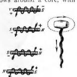
twist, the north pole of the magnet is at the far end of the core.
