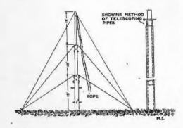
section easily. The third section can be made as long as desired and is small enough so as to slip into the second joint easily. The novel part of the mast is the method by which the sections are fastened at the joints. Two holes are bored at each end of the pipes, one foot apart, and two more bored at right angles to them, as shown in sketch. A step made of strap iron is fastened on the first joint to aid in erecting it.
