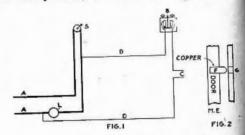
is represented by light lines in the diagram. AA are service lines and S is a snap switch at the head of stairs leading to the cellar. L is a light or many lights. C is the contact made at the door, which is shown in detail in Fig. 2. One wire is connected at F and the other at G. B is an ordinary telephone magneto bell, either of 600 or 1,000 chms, mounted on a block of wood.
