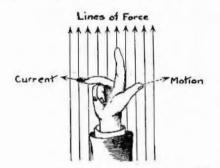
movement, the induced current will then flow in the direction of the middle finger.
