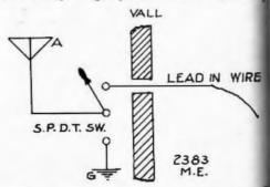
nection running to the ground from this switch should be as straight as possible, with no sharp turns or abrupt
