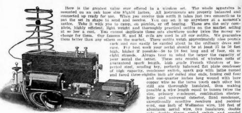
of high capacity, condenser switch, spark gap with lathe turned and faced three-eighths inch air coiled zine ends, tuning coil four and one-quarter inches long wound with bare
