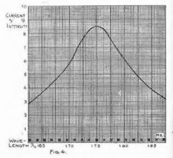
than 1.1 of it. For example, suppose the standard wavelength of the set is 175 metres, then the central vertical line would be marked as shown in the illustration. The other wavelengths would also be marked as indicated. Along the vertical line at the extreme left, numbers are put corresponding to
