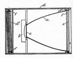
diaphragm which is positioned approximately in the focal plane of the paraboloid and contiguous with the rear edge of the horn.
