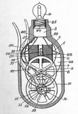
leasing the pressure spring 18 forces the lever back. Each inward movement of the outer projecting end of the lever spins the armature of generator 4, through action of the pawl and ratchet called "Birkeland"—arcs are formed on account of the physical law above referred to. But if the ends of the arc are prevented in some manner from moving along the electrodes, which in such case
