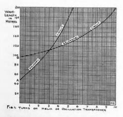
I, must be had, and along the last horizontal line numbers are put corresponding to the turns on the helix or oscillation transformer. In this instance it is assumed that the total number of turns is ten. Along the extreme left vertical line numbers are placed corresponding to wavelengths from o to 200 meters. The transmitting set is then connected together, as shown in Fig. 2, with one
