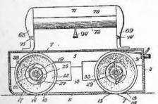
the interior of the casing, 2. 94 is a finger contact lever for reversing the motion in the propelling roll, 15, said lever being shown here in its normal, neutral position, in which both the motor and the heating elements are cut out of circuit. The roll, 14, is hollow in construction and is provided with a cylindrical shaft, 19, whose extremities are journaled in suitable bearings carried by the side walls, 10, respectively, of the
