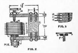
lower support of the gap. 9 has no groove in it, as electrode, 8, has the necessary groove.
