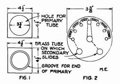
describe the making of the base. The base is made of whitewood. It should have the dimensions  $18 \times 12\frac{1}{2}\times 3\frac{1}{4}$  inches. The edges should be beveled. The ends which support the primary should be  $4\frac{1}{2}\times 4\frac{1}{2}\times \frac{1}{2}$  inches. In one of these pieces a round hole must be cut
