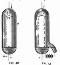
On account of the necessity of using full-sized apparatus, together with a corresponding amount of electric current to be able to perform experiments with this device, these are very difficult and beyond the scope of this article; consequently none will be described. However, the mercury-arc rectifier is too important a piece of apparatus to pass by here without explaining its construction and operation. The principle on which it is based is as follows:
