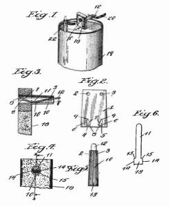
perhaps more. The working of this binding post is identically the same, the spring, 12, being depressed in order to uncover the hole, 3, Fig. 3, which breaks the connecting wire, 20, Fig. 1. The trouble with the present post is that it is too stiff and unwieldy and also looks dangerous on account of the sharp points.
