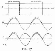
given by the rectifiers just described. The rotary converter\* gives a current curve about like that shown by the full lines at A, Fig. 47, if the alternating current supplied to it is as represented by the dashed lines (the mechanical converter,† which † See p. 155, May issue.
