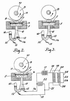
breaker in which effective means are utilized for overcoming the tendency of the contact points to oxidize. This and other objects we attain in an apparatus described and illustrated in the accompanying drawings, throughout the several views of which like parts are denoted by corresponding numerals.
