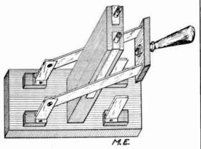
This switch has been in use in my station now for over a year and has proved satisfactory in every respect. It is so simple that any amateur can make one. As will be seen only a throw of  $30^{\circ}$  is required to change
