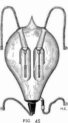
This starts an arc with the upper electrodes, and completes either of circuits MGDLJM or MFDLKM, depending on which part of the A. C. cycle is being generated, by M, at that particular moment. In either case current flows through L in the same direction. It therefore follows that the current always flows through L in that direction, since it does so at any part of any cycle.
