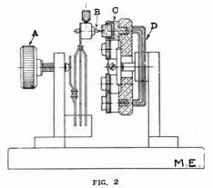
the design of the instrument enables a light yet reliable pressure to be maintained.
