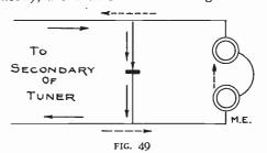
If, however, we put a rectifer (the detector) in series with the receivers, the oscillations are rectified to a pulsating direct current. Inasmuch as direct current, even when pulsating, cannot be entirely choked back by mere self-induction, it is now able to produce a sound in the telephone receivers.
