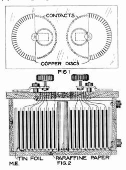
but a core about 4 by  $1\frac{1}{2}$  inches is right for the average station. The tinfoil is applied between sheets of paper as is usual. Bring the lug or connector of the first sheet out at one end and the lug of the second sheet out at the other end, and so on, staggering the lugs at one end and keeping them in line at the other end, until about 120 sheets are ap-plied. Now connect the 60 lugs that line up together and place this end down in a case
