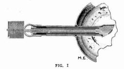
new tube which has a tungsten target attached to a metal rod which is brought out through the neck of the tube and provided with radiators. Anyone familiar with the subject, will at once recognize the advantage of the new construction, for with the old arrangement, the heat had to be radiated through the glass forming the neck of the bulb, while in the present arrangement the heat is conducted directly to the outside air and the
