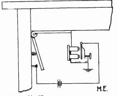
wireless table like cut. I use this "key" on my buzzer test circuit and when I am operating I have both hands iree to work switches, etc. To operate the "key": sit near enough to the hinge to press it with your knee and close the circuit.
