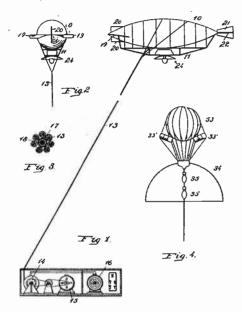
In the accompanying drawing, Fig. 1, is a view of a dirigible type of balloon, moored to suitable mechanism, and carrying a light and reflecting apparatus. Fig. 2 is an end view of the balloon. Fig. 3 is a section of the cable employed. Fig. 4 is a view of a spherical type of balloon, with a modified type of lighting and reflecting apparatus.
