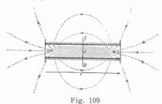
It is usually agreed that the lines of force go from the north to the south pole. This is shown in Fig. 109, which represents the lines of force in a solenoid or magnet; they form closed curves and seek to traverse the shortest path.
