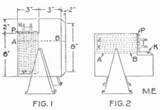
held at any desired angle. A one-half inch hole is bored at K, into which a tight fitting cork is inserted after battery is charged. For charging pour in three ounces of Bichroniate of Potassium, six ounces of Sal-Ammoniac, then fill up with water and allow to dissolve. If a weak solution of Sulphuric Acid be used in place of the Sal-Ammoniac, we get a more energetic current, but the life of both the zinc and the solution will be greatly shortened.
