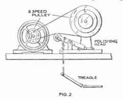
9 inches, the intermediate one 7 inches and the smallest 5 inches in diameter. These pulleys may be easily made by
