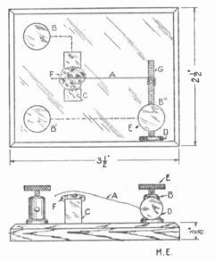
A, is the silver wire; B, B', B" are binding posts; C, is crystal holder; F, is crystal; E, is a lock screw on wire holder; D, is rubber knob; and G, the threaded rod.
