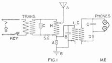
The connections shown below are provided to overcome the necessity of having this key contact and they work very satisfactorily on a half kilowatt outfit and will probably work the same with larger outfits. In the diagram, at A, is inserted a knife edge spark gap which can be made of sheet copper as shown in Fig. 2. This gap is merely an anchor gap inserted between the helix and the ground and it is set very close so that the current will pass into the ground direct. The in-
