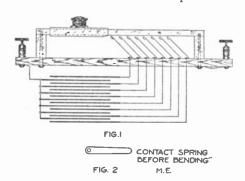
and fasten to the wood with small screws, connecting a section of the condenser to each one. Bend them up until each one nearly touches the one-quarter inch rod. Now, when the five-sixteenths inch tube slides over the rod it
