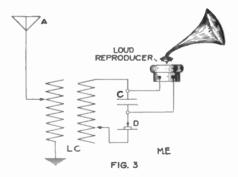
phone is constant and its diaphragm does not disturb the air with sound waves; but as soon as wireless signals pulsate through the receiver (R) its diaphragm vibrates according to the frequency of the received oscillations and lets the current flow through the microphonic contact accordingly. The battery used consists of three dry cells.
