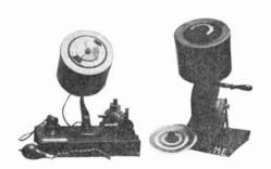
discs are adjustable so that any amount of the three primary colors may be combined to match any given color. A graduated circle shows the exact amount of each color used. An apparatus of this sort is very useful in matching or analyzing colors. The motor operates on the lighting current with a resistance in series. At the right is also shown a hand operated machine.
