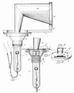
First—The part, p. is a screw portion fitting the part, n. Thus the electromagnets, e', are made to approach or recede from the diaphragm, to obtain the best results.
