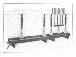
meter connected to a step down transformer of known ratio. If the voltage must be measured directly a needle point spark gap must be used. The illustration shows such a gap for very high potentials, connected in series
