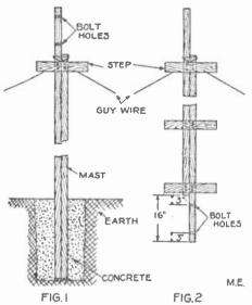
four feet deep. The guy posts are four inches square and eight feet long. They, and the mast are set in concrete as in Fig. 1.
