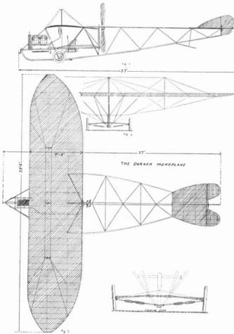
allow plenty of clearance, but taper to a point both front and rear. The fuse-lage uprights are put in slanting fashion, thereby acting as cross braces and eliminating the necessity of wire bracing. Owing to the depth of the fuselage in front the pilot is provided with roomy seating accommodation and also has an unobstructed view in all directions.
