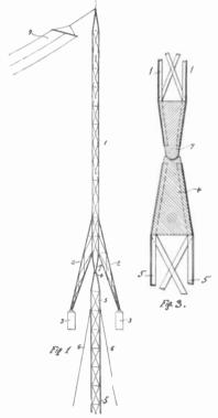
mous, in order to put even a small strain upon the aerial, 9. The inventor also states that four counterweights, instead of two, could be used.
