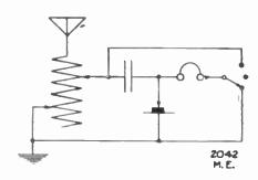
Q. 2.—How far would the above set receive with an acrial about 40 feet high at one end, 25 feet at the other, and 60 feet long?
