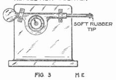
against the belt, tightening it, and starting the lathe. This arrangement will be found especially valuable for coil winding. The lathe can be stopped instantly, and started without any jerk.
