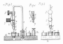
used for an electrolytic detector, and the Wollaston wire, p, is clamped by the spring, o, also a novel arrangement.
