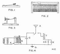
twelve dry cells connected in multipleseries (two rows of six cells in series). These batteries I got for nothing at different garages in the city, being considered no longer fit for use; but I found I could get quite a respectable current from them when a large number was used.
