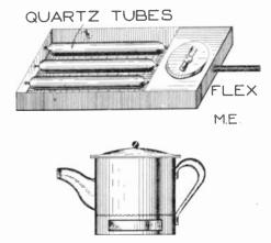
incandescent units having the heating wire sealed into exhausted tubes. This arrangement allows the heat to be freely radiated, with little absorption, and, at the same time protects the wire against oxidation. The heater is adapted to slide into a recess in the bottom of the double bottomed kettle, like a drawer in a cabinet, and is provided with a heat regulating switch.
