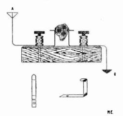
top of these screws place a thin washer (cut out of the same material as the prongs); next cut out two pieces of thin brass as shown in Fig. 2 and bend them at the dotted lines with a pair of pliers so that they correspond with Fig. 3. Now under the binding posts and on top of the washers place these two pieces so they will stand upright in the form of two prongs. When you have gotten the detector assembled it should be shellaced and varnished.
