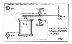
ing as many oscillations per second as any double magnet type, this is due to the double contact.
