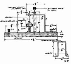
sions and shows how the detector is assembled.
