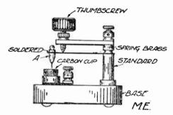
ment for holding the delicate Wollaston wire. Amateurs become disgusted with fingering minute screws and discard a most excellent detector for a more convenient, if not so efficient, type.
