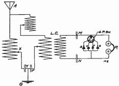
X and Y were added, to cut out static, the tone of the signals was reduced
