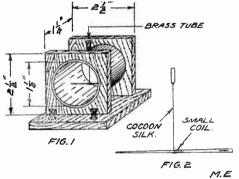
tube at the top. Wind about onefourth pound of No. 30 D.C.C. wire on the reel. Be sure that the same amount of wire is wound on either side of tiihe.
