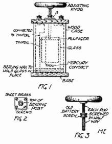
2. About one-half pound of mercury. The mercury is used as one of the conducting surfaces of the condenser. Its level is raised or lowered by turning the adjusting screw. If desired, water may be substituted for the mercury, but this will increase the resistance and the water also has a tendency to "creep."
