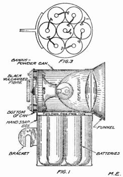
that the lamp may be conveniently attached there. The cover of this can should be punched with two holes, of the same diameter. In the box the batteries are placed and sealed. These batteries consist of small test-tubes which will easily fit into the box, and when as many as possible have been crowded in, melted paraffine should be poured around them, until it comes on a level with the top of the test-tubes.
