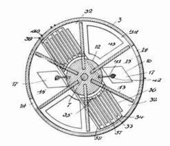
mal position. At each actuation of the trap the conveyer is moved through a semi-revolution and carries the rat into one of the compartments 32 where the rat is electrocuted by contacting with the bars 33 and 34, and after it is electrocuted it is precipitated through the opening 43 into the pit or well 1, from which the rat can be removed by shifting the trap from over the pit or well.
