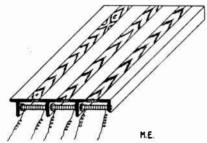
magnets between them as shown. Strips of wood are fitted in between the iron pieces to make the surface of the floor smooth.
