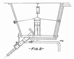
situated in front of the lamp to regulate the voltage and amperage. The method of arranging the arc lamp and the telescope is shown in Fig. 2.
