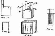
While it is true that some storage battery plates have lugs by which they are supported on the edges of the jar, it adds an inactive weight to the battery and does not provide for the support of proper separators for the plates.
