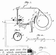
pulses are sent over the line Z, which energizes magnet M, which in turn operates the stylus m<sup>5</sup>. The drum A<sup>1</sup> is practically the same as transmitting drum A.
