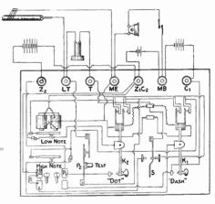
pressed for "sending," and raised for "receiving"; if, however, automatic switching be preferred, it is always feasible. The contacts on keys 1 and 2 are arranged so as to be suitable for use, if required, with two electro-
