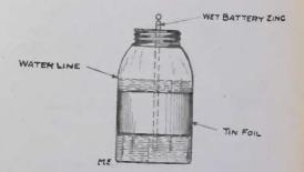
and long enough to go around the jar, and a wet battery zinc. Remove the glass from under the can cover and bore a hole in the top of the cover, next fill with water up to dotted line on sketch, add a teaspoonful of salt to the water. The sketch will explain the rest.
