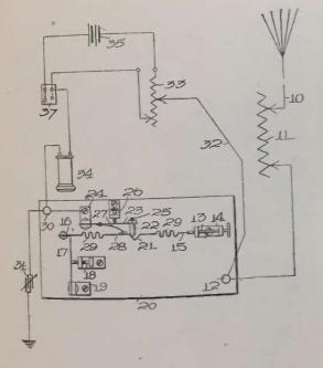
made to vibrate longitudinally, thus contacting with the part 22 which has a conical point and engages with the off-set portion 21 of the conductor 15.
