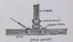
The skids, skid braces and seat rests are joined with small pieces of sheet steel and <sup>1</sup>/<sub>8</sub> inch diameter stove bolts. This is also clearly illustrated.
