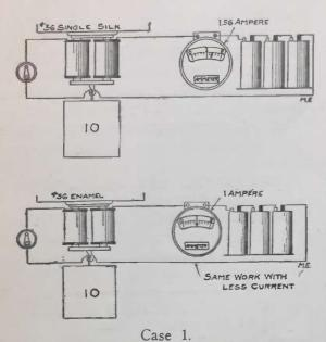
through the use of enameled wire for winding magnets.
