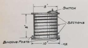
One half inch from the top of the tube start winding the wire and continue winding until a section one-half inch wide has been completed. Break off the wire allowing about one foot for lead and fasten. Measure one-half inch from completed section and wind
