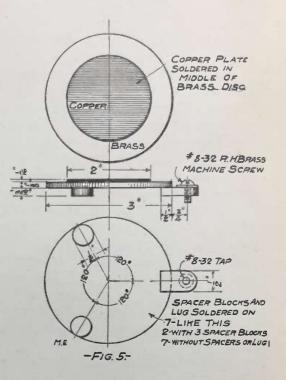
brass discs. Lay each small disc on the middle of one of the brass discs, (with the tinned sides facing each other), heat until the solder melts, then press firmly together and allow to cool while still under pressure. Seven of these composite discs are now finished as far as soldering is concerned, and may be laid aside.
