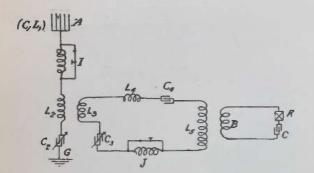
In practice Mr. Hogan constructs the tuning box L2 and L3 and C 2 with leads attached to connect the antenna and ground in circuit with L2 and he uses but a single variable pointer or indicator, that is, the slide of the coil represented by L2. Thus any kind of tuning element may be varied as long as it is common to both circuits.
