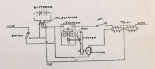
At the first tick the relay closes, starting up the motor which turns the roll of paper. The sounder presses the pen down on the paper making a dash. The pen then proceeds to take down the message until finished, when the operator at the other end of the line changes the direction of the current he is sending. The relay is then opened and the motor stops.
