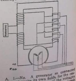
would not excite its own fields, for the rea-son that the algebraic sum of the voltages in the three physics of the phase circuit in the three phases of a three phase circuit is always zero. Hence there would no current to excite the fields.
