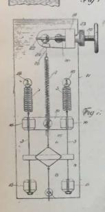
Van Wagenen Mr. uses a hydrometer 9, which floats in the solution of the storage battery electrolyte 10. As the battery is charged the hydrometer 9 rises, and moves up the rod 8, which is held by a spring 7. The rod 8 also moves a metal connection piece 4, which slides on the resistance wires 3, 3. Thus any variation of the slider 4 will naturally make a difference in potential and this difference will be recorded in the recording Inasvoltmeter 14. much as this voltmeter
