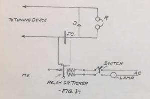
contact points, are connected to the two sides of the fixed condenser in the receiving circuit. Two different hookups are shown below.
