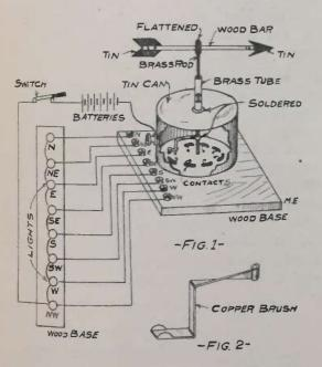
the vane revolves according to the direction of the wind, the brush comes in contact with the brass pieces and completes the circuit through one of the lamps. The lamps are marked with letters corresponding to the points of the compass. The brush, Fig. 2, is made of sheet copper.
