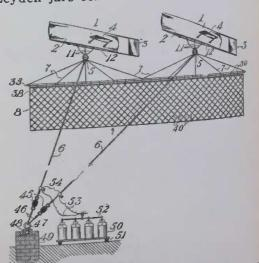
Mr. Pennock employs a metal netting 8. which is held suspended by balloons 1 attached to a swivel arrangement 5. In order that the electricity does not rush to the ground whereby a terrible loss would surely be the result, the inventor uses the in-sulators 45, which check the flow of elec-tricity and force it to trickle down into the jars 50
