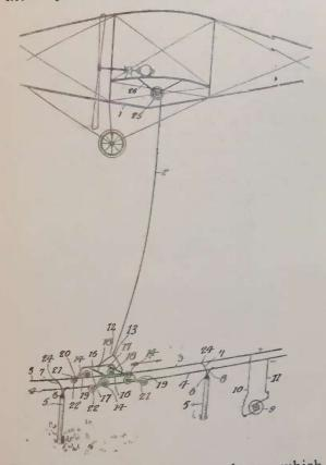
uses a double set of trolleys as shown, which are made to run from the electrical highway formed of the cables 3 and 4, to which power is furnished by generator 9. The power is thus transmitted to the cable 2 and acts on the electric motor of the airship
