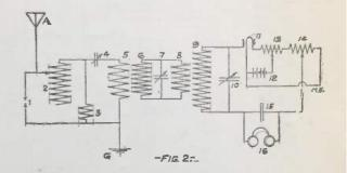
tuner, the coils of the loose couplers are not variable, and all the tuning is done by means of the variable loading coil, the variable condensers, and by varying the coupling between the primaries and secondaries.
