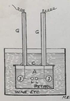
and a pair of larger aluminum balls (J) which serve as oscillators. The apparatus is connected to a spark coil by means of the wires extending up through the tubes. The tubes also serve to allow any gases that form in the tank (A) to escape to the atmosphere.
