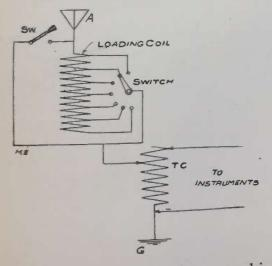
Continue making another section. these sections until the tube has been filled but a space of one-half inch should separate each section. The lead from each section should be led to a switch and connected as per diagram.
