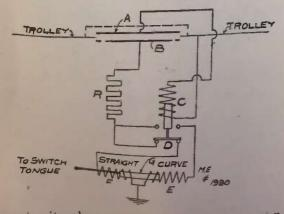
to raise its plunger and the disc D into connection with the upper contacts. Current from B then flows through the resistance R disc D and upper contacts, and solenoid E to ground, moving plunger G to right and setting switch for the curve.
