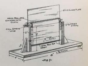
springs, one for each end of the condenser. These are slipped over the screws together with the brass strips before the screws are put into the wood rolls. I have found this to give fine results and it works very smoothly when glass plate is moved up or down. As the brass springs hold rolls firmly against plate nearly perfect con-
