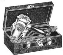
The hair dryer consists of a small motor driving a blower. In the large tube leading from the blower, a heating unit made of many turns of resistance wire is placed, with a rheostat in the circuit for regulating the temperature. The motor is of the very best construction, with the best of materials used, insuring perfect satisfaction under the worst treatment. One of the illustrations shows the apparatus placed in its carrying case, while the other
