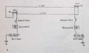
actly as shown; that is, each line wire is to be connected to different posts on opposite ends, and the sounder wire is to be connected to the back contact of key at each end. The break key should be similar to the "Electro" double-circuit "Cinch" key, using the upper contact. Diagram shows battery at each end, although it may be placed at one end if desired. A good ground is absolutely necessary to get good results. Contributed by
