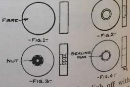
with sealing wax and polish off with a piece of emery cloth. You then have a handsome and serviceable thumbscrew.
