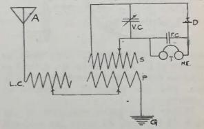
waves properly, was because better selectivety could be secured by having a small primary, and then using a loading coil for taking in long waves.
