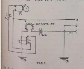
he led together and the coil placed at the end as in the diagram. The closedcircuit trips CC are connected in series, while the open circuit ones are in Parallel. One of the relays R is adjusted (by the spring) so that it is normally attracted and away from the
