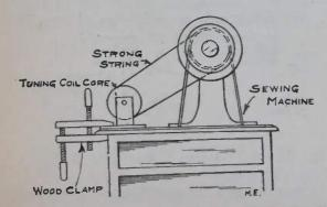
make a frame by taking a piece of board about 2 in. longer than the core, and nail two pieces upright on each
