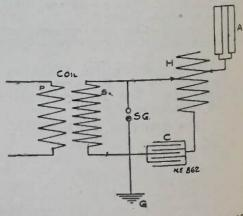
A. 2.-We think you could transmit about 40 miles and perhaps 50 with your transmitting set of perhaps in However, transmitting set as described. However, we do not quite understand what you mean with tubular accordent with tubular condensers, as tubular condensers are usually used for receiving only. You probably are referring to leyden jars.
