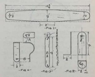
this bend should be regulated after the headband is finished so as to make the phones fit properly. The remaining piece is cut lengthwise into two pieces, each  $\frac{1}{2}$ " by  $4\frac{1}{8}$ ". These strips are rounded on the ends, and each has holes in the ends to fit the screws in the sides of the receivers, and a  $\frac{1}{8}$ " hole in the center.
