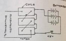
also suggest using about 20 dry cells in series multiple to work the coils. This would in all probability transmit the required distance with the large aerial you have.
