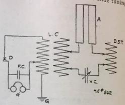
coil, double-slide receiving transformer, rotary plate variable condenser, Murdock improved silicon detector, fixed condenser and phones with a joint resistance of 4000ohms, aerial composed of four No. 14 aluminum wires 60 feet high and 60 feet long, ground on water pipe and chicken netting in moist ground?
