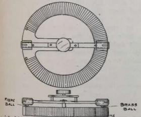
with No. 24 enameled wire. All arms are of square brass 1/4 inch by 1/4 inch. The supports of a somewhat smaller diameter. Sliders are mounted on ends
