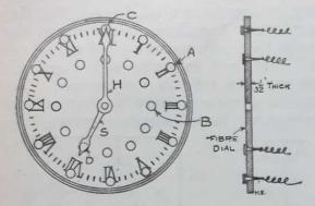
numerials are driven 12 more tacks as shown at B. These tacks are driven as close as possible to the surface of the fibre, and not separated therefrom by washers.
