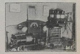
gap, key and six volt, sixty ampere storage battery for coil and lamps.
