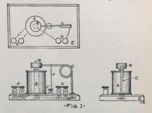
trolling high tension current such as used in the use of a wireless telegraph
