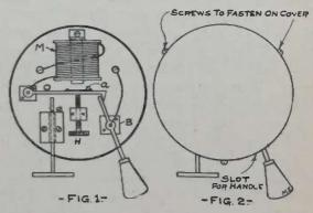
The levers are supported on blocks of hard wood which are screwed to the base. The binding parts are on the back, as the circuit-breaker was made for switch-board. The arm O can be adjusted by the screw H so that it will break at a small or large current.
