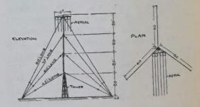
ing first seen that the mast is perpendicular. The spreaders should be 15 feet long, six wires giving a distance of three feet between each one. Insulators capable of withstanding the energy to be used are inserted about eight inches from the spreaders, which should be shaped and supported as shown in the drawings.
