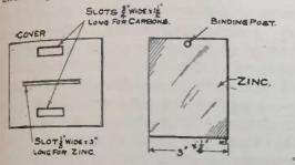
inch from the bottom of the crock. Now take the cover and cut three (3) holes in the top as per sketch, insert the carbons with the binding posts on. Next put the zinc in with a binding post on, which will also serve as a
