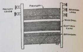
Over the secondary a few layers of paper are wound to serve as insulation tube.
