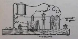
splendidly. Wind a bell magnet full of No. 14 insulated wire and secure to a brass standard as shown in drawing. Make a base of any hard wood-the
