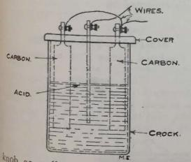
knob as well as a connection. make a solution of Potassium Bicro-Now mate 8 oz; Sulphuric Acid 17 oz. and Water 56 oz. Connect the carbons together and bring one wire out for connections from both carbons and one from the zinc. When the battery is Not in use take out the zinc as the acid eats it very rapidly. This battery Will give two volts if properly constructed. If four cells are used will <sup>tun</sup> a one inch coil. Contributed by
