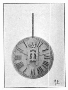
influence of the coil the armature is impelled against the pendulum, driving it forward, after which the circuit is broken, leaving the armature free to be returned to its original position under the momentum of the pendulum in its return swing. The swinging pendulum also operates the escapement lever by which the clock mechanism is advanced so no weights or springs are necessary.
