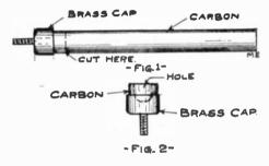
Hunt about until you find an old dry battery having a round carbon and the binding post on top, such as the Ever Ready battery has. Now proceed to take the carbon out, being careful not to injure the brass cap or the thread. With a hack saw cut the carbon about  $\frac{1}{4}$  inch from the cap, as in Fig. 1. Now, with a  $\frac{1}{4}$ -inch drill, drill a hole about  $\frac{3}{8}$  inch deep, as in Fig. 2. You now have your carbon cup complete.
