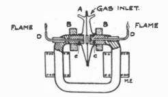
A very sensitive receiver which can be used either for wireless work or for ordinary telegraphy is here represented. The current coming in on the line gives fluctuations in a pair of small flames, corresponding to the signals, so that
