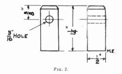
rod are also made of hard wood  $\frac{1}{2} \times \frac{1}{2} \times \frac{1}{4}$  inch. A hole  $\frac{3}{16}$  inch in diameter, to fit the sliding rod, should be bored with its center  $\frac{3}{8}$  inch down from the top of each support and  $\frac{1}{4}$  inch in from each side. A small bevel can be cut around the top of each supports are shown complete in diagram 2.
