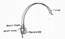
some stiff 1-inch brass long enough to go over the head and 2 inches to spare. Bend over about 1 inch on each end and pass a stiff wire through where it is bent. Now wrap clear across with tape. Now bore two holes in each receiver on opposite sides and place wire in them. When bent to fit the head, the headband is complete.
