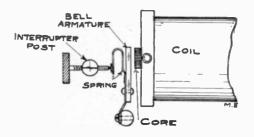
by merely bending the copper contact, which bears the platinum, around to come in contact with the thumb screw bearing the other contact, as per drawing.
