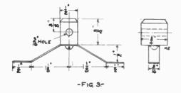
The slider should be put on the sliding rod and then the ends should be put into the supports. The supports are held down to the base by countersunk screws passed up through the bottom.
