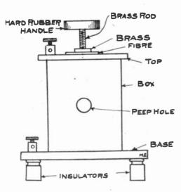
a 3/16 inch hole in the center of the fibre and screw the brass to the fibre, the fibre to one *end* and that in turn to the cover of the box.
