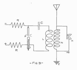
cuit slightly, and also affects the current in the sending aerial. Words spoken into the mouthpiece, therefore, produce an effect upon the amplitude of the emitted electric waves, and these are, so to speak, moulded into speech form, that is to say, made to vary as to the ordinates of a wave curve representing the change of air pressure taking place in the transmitter.
