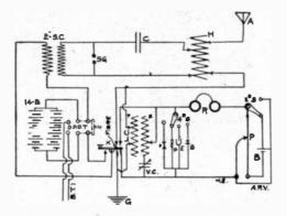
The receiving set consists of one tuning transformer, variable condenser, silicon, ferron, perikon and electrolytic detectors, 2 1,000-ohm phones, and a potentiometer.
