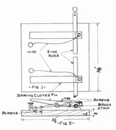
clothes-pins to posts in middle of base. Place zinc rods in the jaws and your spark gap is complete. Contributed by
