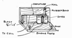
the binding posts. Then connect the wires from your key to the dimes and use your key to work this instrument. It works well on three dry batteries.
