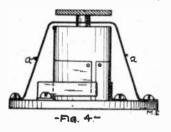
in the center of which a hole has been bored to insert the axle for the spool. Get a steel or brass strip and bend it as shown at a Fig. 4. Make a handle by boring a hole the same size as the axle in a small strip of wood. Put on the
