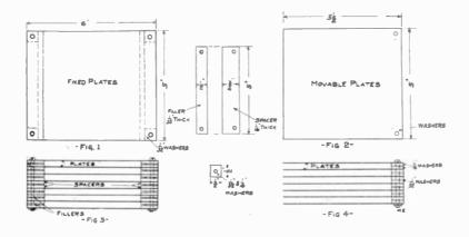
In the up-to-date receiving station a variable condenser is an absolute necessity. Of the various types, those employing sliding plates, with air as a dielectric, are preferred by many. The difficulty, however, of grooving a frame to receive the plates has deterred many amateurs from constructing a condeser of this type.
