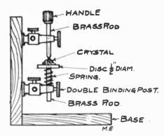
brass rod. The spring (6) presses this upward and as the crystal (7) is placed on this disk a firm pressure is maintained on the crystal by the pointed upper electrode. The upper electrode
