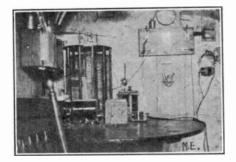
ers (under table and operated from above), electrolytic and silicon detectors with 3,000-ohm phones.
