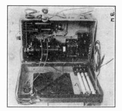
and enhance the sending power. The complete outfit can easily be carried by one man.
