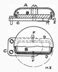
ries the tapper for the bell. On the base plate, C, is mounted an iron piece, B, which serves as a core for the movable coil and the magnetic circuit is completed by the iron bell A. The coil, D, sur-
