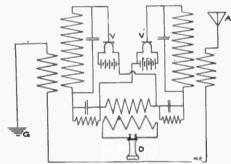
One of the circuits is in resonance with the waves to be received, while the natural period of the other circuit is made slightly different. The detectors are connected so that when the capacities and couplings are well adjusted, the currents which they supply to the common telephone receiver, D, due to the disturbing influences, will oppose and neutralize each other.
