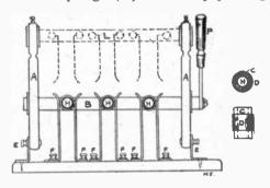
or pulling handle (P) you can operate switches on either side. (E) is brass strips bent in L-shape and fastened to
