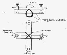
be made from two poreclain cleats, two binding posts, two nails and a little string. Such a gap when finished can be screwed to almost anything and is capable of carrying about one hundred watts with ease, in fact, the writer uses a similar one with a one-quarter kilowatt open core transformer using an electrolytic interrupter.
