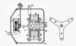
being mounted on a star-shaped spring piece somewhat as we have just seen. When the rod E moves back and forth, it gives a variable pressure on the carbon grains and a strong current, N, is sent through these. Variations in the telephone circuit are thus translated into like variations in the strong current circuit.
