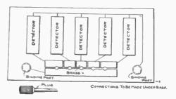
base for detectors and device for cutting in any number in multiple. There is
