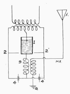
disturbances. The second figure shows a double valve connection. The cooled electrode (1) is connected at the middle point of the transformer secondary, with the other electrodes (2) (21) in separate circuit with the condensers (4) (41) and a common induction coil (9) so that first
