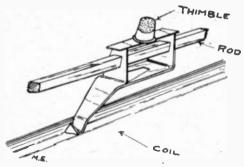
slider that works good on a square rod. The diagrams explain themselves therefore a description is not necessary.
