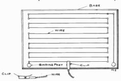
inches and tack on about 20 small nails about half way in. Now procure some German silver wire about the size of a thread and wind it on the nails, as per sketch, about 10 or 15 feet is sufficient, which can be purchased for 5 cents.
