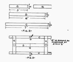
fasten them on the under side of the pieces a a, as shown in Fig. 3, and then solder a short piece of flexible cord to the center of each at D D, Fig. 3, which go to binding posts 1 and 2, Fig. 5, for the aerial and ground. This entire framework sets on the pivot B, Fig. 1. From a piece of No. 26 or No. 28 spring brass cut out four pieces like Fig. 4, and after making the holes, bend at right angles on the dotted lines. Two of these pieces
