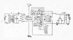
2.—My sending set consists of a 2-inch coil, key, helix made of 30 feet of No. 8 copper wire, wound one inch apart, leyden jar condenser, six Edison primary batteries, and same aerial, water pipe ground, and zinc spark gap. Are my instruments well proportioned?
