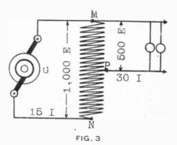
In effect, the device may be considered an alternating current inductive potentiometer.\* By taking out a number of taps from different portions of the winding and connecting them to a multiplepoint switch, any desired potential can be obtained. A higher pressure than
