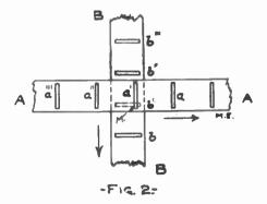
pass across its whole length. The band B then comes down one step so that another of the slits B comes into place, and this is again passed over by A, etc. However, the spacing of the vertical slits is such that at each move, the next slit B will come to a point lying next under the former position, so that a new line of the image is uncovered each time. This is done by spacing the slits B at, say, 9/10
