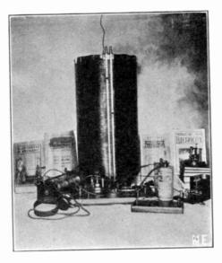
front of board is the fixed condenser and battery.
