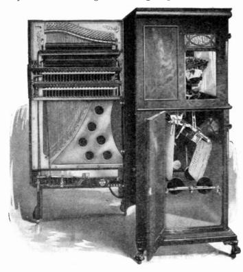
is performed by a bank of electro-magnets, whose armatures depress mechanical fingers over the strings on the finger-board. The effects of staccato,
