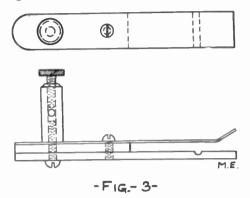
If very heavy wire is used, a piece of brass as thick as necessary, 1/2 inch wide and 1 5/8 inches long may be placed between spring and bottom, as seen in Figure 3 with arrow pointing it out. This is done so the strain on the spring is not so great. This will prove an excellent helix clip when finished.
