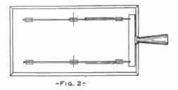
switch, the length should be about one and one-half times the length of the blade. They are next offset in the man-
