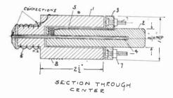
After part 1 has been shellacked and rubbed down, the wire is run onto it, first drilling hole through to part 6 and shoving wire in and soldering it to outside of base. Each turn is separated from the next by its own thickness. The other end of wire is wrapped around a small brad and tacked fast. It is well to have the sliding brass strip touch two turns of wire at a time, giving good, broad contact and preventing slider from digging in between turns.
