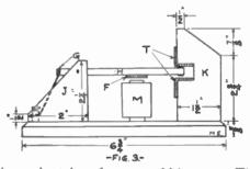
A can be taken from an old battery. The rubber R is fastened from the lever to the base to bring the lever up. C is a brass plate 5/8 inch by 3/4 inch to make contact with A. D is a brass plate so
