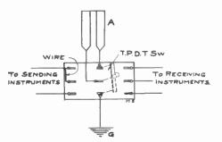
and connect the two aerial lead-in wires to two of the levers and the ground to the third. To one side connect the receiving instruments as in any other switch. On the other side run a wire (about No. 14 for average use) from one post to the other, which makes contact with the aerial, thus bridging across. Now connect as with a straight aerial switch.
