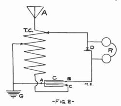
condenser is connected, and connecting C to the end of the coil winding, the signals come in a great deal louder than by the ordinary way by connecting.
