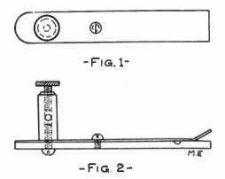
spring brass and bend as seen in Figures 2 and 3, 1/4 inch from front. Then drill and tap for a 5/32 inch machine screw, 1 1/8 inch from back end, then take a binding post and drill hole 1/2 inch from
