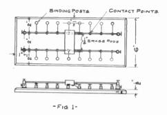
battery and file out the screw part smooth. Two of these should be used for every detector. Bore 9 holes 2 inches from each side and end. Place 18 of these bolts in the holes and put nuts on
