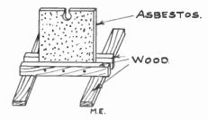
lumber nailed to some cross-pieces (Fig. 1.) with a small groove in the top to hold the wire will answer the purpose. A square of hard rubber or shellacked wood with the groove lined with asbestos is also good. About one inch below the top and in the center, bore a hole, a little larger than the lead-in wire. Then saw a narrow slit down from the top.
