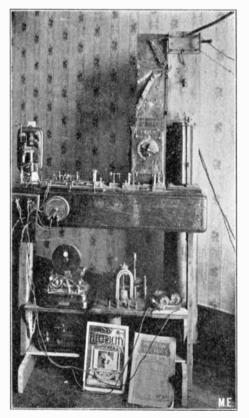
contacts. I use a heavy telegraph key to operate the coil and seven storage cells to supply current. From the secondary terminals of the coil I can get a heavy flame of fire about an inch long. By using a glass plate condenser this spark can be cut down to a white flash from a quarter to an eighth of an inch in length.
