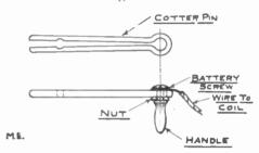
Secure at any hardware store a oneinch cotter-pin, hold the sides apart and file a notch of suitable size one-quarter inch from the end.
