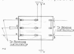
front connection fuseless switch has been used by me. Binding posts 1 and 2 are short-circuited with a copper bar or wire. This is a very simple switch and works very well. Throw to right for sending, to left for receiving.
