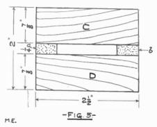
groove which you made, and fasten the two ends of the wire to two binding posts. After you have wound the wire the compass will just fit under the wire and between the blocks a and b.
