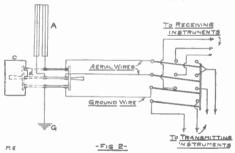
The binding posts on one end of the switch are connected by a heavy copper wire e, about No. 10 B. & S. Wires a and b from the other two posts go to the instruments.
