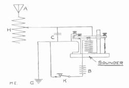
as shown here. The armature should be connected so as to buzz or vibrate when key is pressed.
