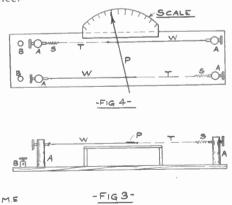
The operation of the instrument is as follows: The current passes through one of the fine wires, thence through the pointer and out the other fine wire. As (Continued on Page 586)
