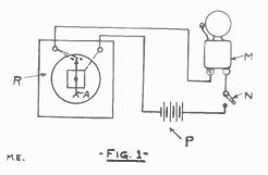
The instrument must be placed in such a manner that the needle will rest between the tacks, touching neither. Connect it in series with a bell and bat-
