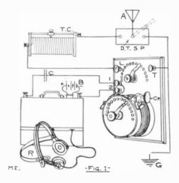
give a closer tuning in the case of great wave lengths. The switch serves to put the aerial to ground when not in use or in case of storms.
