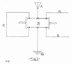
I have an easy and quick method for grounding aerial during storm, etc.
