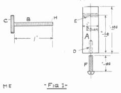
E should be about ¼-in. from the top, at D drill and tap out a short hole to receive the screw F, this should be about ½-in. long and made of ⅙-in. stock. This screw is to hold the post A in an upright position on the base, which is done by passing it up through one of the holes H (Fig. 8), and then screwing the post on top of it.
