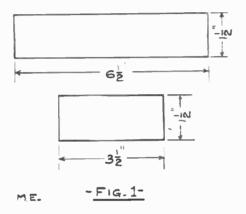
The core laminations are cut as shown in Fig. 1, from stovepipe iron about twenty to the inch. Only two sizes are made 1½ in. by 6½ in. and 1½ by 3½ in. Enough of each size should be cut to make a pile three inches deep. This is best done at a tinshop on the square shears, as then all the pieces will be of a uniform size.
