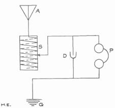
a small copper wire as a slide and connecting one end of the layer of brass wire to the aerial this simple tuning coil worked with great efficiency. With only a small indoor aerial and a 75-ohm phone it received a distance of about twenty miles.
