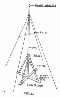
and place it in the hole, and insert it in the end of the pipe. Now get two pieces of hard wood three feet long and two others three feet six inches long for (Continued on Page 548)
