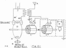
through the receiver R. The discs at the sending and receiving posts are driven at the same rate by synchronous motors.
