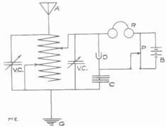
able condenser is sufficient with a double slide tuner.
