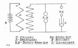
connected across the same terminals with the spark gap "S G," as shown in diagram, with another spark gap "S' G" a trifle smaller than "S G," so that the spark will jump here instead of the other.
