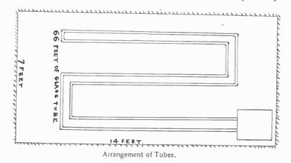
134 inches in diameter, containing a rarefied gas. The ends of this tube enter a terminal box containing the necessary electrical apparatus, and when electric current flows through the tube it produces a soft and extremely well diffused illumination throughout the tube.
