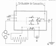
TRICS. All the binding posts, switches, etc., are mounted on a board of convenient size (about  $12 \times 15$  inches). The dotted lines show how binding posts are wired on under side of board. In center of board is shown a three-point switch with which either of the three detectors, electro-lytic, silicon or carborundum, may be thrown in circuit.
