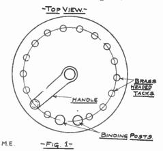
brass-headed tacks, 5 feet No. 20 B. & S. bare German silver wire, a box of small tacks 1/8 of an inch long, 3 binding posts, and a piece of wood 2 1/2 inches long, by 3/8 inch wide, by 1/8 inch thick.
