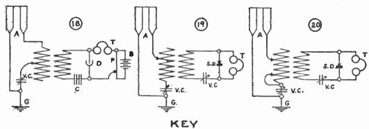
A = AERIAL B = BATTERY C = FIXED CONDENSER D = DETECTOR G = GROUND S.D= SILICON DETECTOR T = TELEPHONES V.C.= VARIABLE CONDENSER SINGLE SLIDE TUNING COIL STRAIGHTAWAY AERIAL DOUBLE 0 Ø CLOSE COUPLED LOOP -LOOSE 89 STRAIGHTAWAY 1 8 . LOOP . (18) 20
