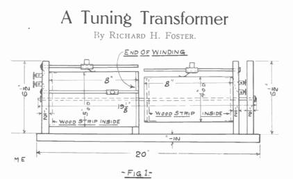
The following transformer can very easily be made by any amateur, and it will be a valuable addition to any wireless station. The expense is not much when compared to the cost of an ordinary tuning coil. Absolute tuning as yet has not been entirely established, but the tuning transformer is a long step toward this end. Great care, however, should be used in building this transformer, as a short circuit would ruin its efficiency.
