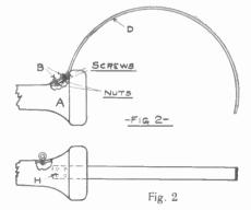
part, shown at B, Fig. 2. I now bored 4 corresponding holes (H, Fig. 3) in the receiver shell just back of the screw cap with a 3/32 inch drill. I now screwed the brass strap to the receiver with four screws, 5/16 inch long. These screws (6-32 or 8-32 thread), are fastened inside with 4 nuts, which makes the head band very secure.
