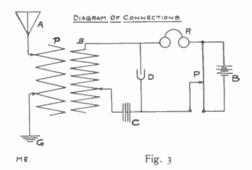
place is found. The secondary slider may then be moved if, necessary. Signals come in very loud with this type of transformer, and distant stations can be heard quite clearly. Without question the efficiency of a station will be much improved with the use of this transformer.
