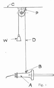
ter this distance again (D. Fig. 1), and passed it over the pulley and fastened one end of the weight (W, Fig. 1), which is a lead or iron chunk, weighing one ounce less than the receiver (A, Fig. 1).
