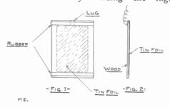
around the edge of the board and fastening the wires leading from them to each board, so that connection will not tear (Fig. 2). The condenser is completed by
