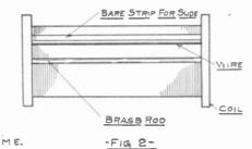
Materials—Round brass rod of any length, and about  $\frac{3}{8}$ -in. diam.; one piece sheet copper  $3.5x\frac{1}{2}$ -in. of sufficient
