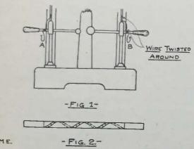
lac and wind the tinfoil on as shown. Let this dry twenty-four hours and then with a sharp knife cut the tinfoil into squares, being careful to cut way across the foil at each place. Next give the ends a coat of shellac for about an inch and wind a piece of tinfoil on each end. This tube should just fit the hooks on the static machine and when the machine is in action should light up with small blue sparks. The balls of the machine should be pulled as far apart as they will go.
