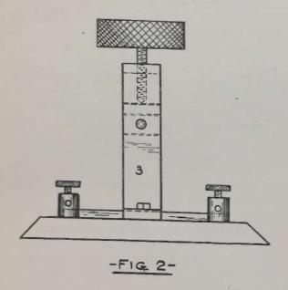
Figs. 1 and 2 show the side and end views of the finished detector. Fig. 3 shows the upright support, which may be made in two ways: either by taking a piece of strip brass 4 x 1/2 x 1/32
