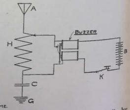
cessfully up to about one-half mile by using ten dry batteries on the buzzer. The helix must be adjusted well to get the right results. The condenser C must also be used in the ground.
