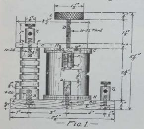
for the standard and other parts, in the base, and having mounted them thereon, the bottom of the screw holes, on the under side of the base should be filled in with beeswax or some other good insulation.
