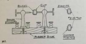
It may be seen that either perikon, silicon, (with point) or carborundum, (with flat surface) detectors, may be used, changing from one to another in a few seconds by turning standard around which gives us flat surface.
