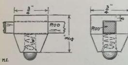
I then drill another hole up through the block to meet the first hole (B). This second hole is large enough to permit a spiral spring to lie in it and is widened at the bottom to admit a ball of steel or iron. This ball makes connection with the rod through the spiral spring and is pushed against the wires by it. The block is tapered toward the bottom and sandpapered.
