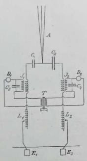
connected to the oscillation transformer J2; this in turn connects to a tuner L2 and ground E2. Condenser C4 is shown connected across the secondary of the oscillation transformer. Detector D2 is in series with the telephone winding at T.
