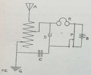
is presumed that you have a double slide tuning coil on which you may use a slide direct to the ground.
