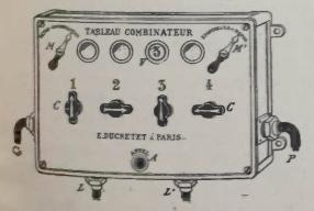
the French fleet. Orders can be very well transmitted to the engine room, the artillery and different parts of the vessel without obliging the men to leave their be used with six receivers at the same points in the vessel, so that the orders are time. The central post on shipboard uses suppresses the use of jacks and cords and all the apparatus is enclosed in a tight
