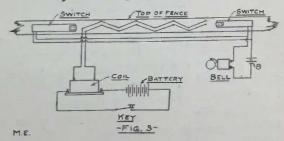
one block. Cut the bed spring in half, and using one piece for each switch, nail it midway between the blocks. Now take the one foot length of board and fasten it, by means of a hinge, on the other block. Having made the other switch in like manner. nect them in parallel, and connect up a bell and battery in series with them (fig. 3).
