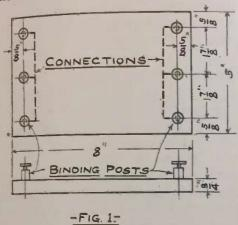
wood, such as oak, 8x5x3/4 inches and mount six binding posts on it as shown in fig. 1, and connect them as indicated by the dotted lines.
