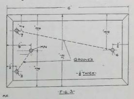
piece Y on R, resting it on N, and slip on the 3/4-inch piece of brass tubing M. Place X as shown in Fig. 1 and screw cap 1 down very tightly. Next screw Z to hole No. 6 on base and after screwing in binding posts 7 and 8, Fig. 3, wire as shown in Fig. 3. Now insert your screws A and B and place a piece of silicon with a smooth surface toward Z, as shown in Fig. I.
