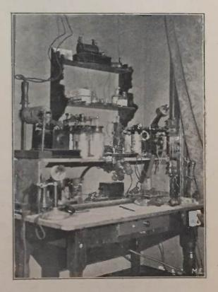
is also a Wheatstone bridge and galvanometer, which is behind the telephone.
