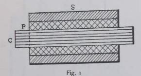
of the secondary is exceedingly low when compared to the resistance of the secondary of an induction coil of the same capacity, the current obtained is relatively very large and the spark that it produces is thick and hot, thus rendering it of great advantage for wireless transmission. These transformers are never rated by the length of the secondary spark but their output is always expressed in kilowatts as in the case with commercial transformers.
