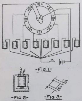
In Fig. 1, the ring with the eight divisions should be two inches outside diameter, and should be made of hard wood. The distance between each adjacent copper segment should be 1/8 in. Each segment is screwed to the hard wood ring by two screws which must be countersunk.
