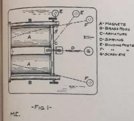
Mount the magnets upon a base-board about 4 by 6 inches. Then make a soft non armature as shown in Fig. 2, and wolder to it a silver or platinum contact n one side, and a spring made of fine
