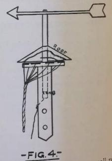
vane, the switch arm, and the small roof are rigidly fastened. At the lower end of this shaft, a narrow groove is cut at right angles to its longitudinal axis. A set-screw screws into this through the outside socket to keep the shaft from be-
