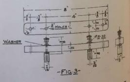
end, the rods to be 1 3/8 inches long. Provide two nuts and a washer and also a battery knurl for each and set together in the inside holes of the 8 inch piece
