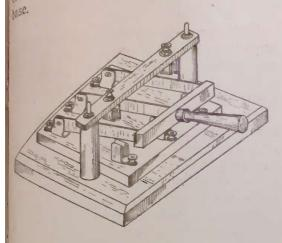
It would be well to measure the distance between the outside poles of the switch before boring holes in crosspiece as when the switch is thrown up these poles should fit in the clips on the cross piece.
