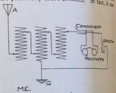
prises us that any result at all is obtained with the above connections. The only way we can explain this slight result is that when the high power government station a few miles away from this station is operating, the energy is ceived is enough to cause a condenser active We believe that by connecting the phones rectly between the aerial and the ground the this government station could be heard quit a little better than is now possible.
