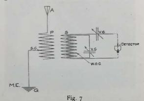
It may be seen from diagram that very sharp tuning can be realized by varying the inductance in the primary, by sliding the secondary and weeding-out coil in or out of the primary, or by varying one or both condensers.
