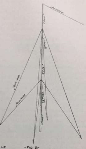
the lower end of pipe. If the pole is to be raised 60 or 70 feet it will need one set of guy wires (fig. No. 1), but if it is to be raised 80 or 100 feet, it will of course need two sets, one near the top, the other approximatly half way down (fig. No. 2).
