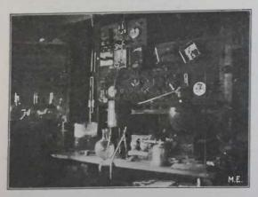
one to twenty volts, oil condenser, telegraph set, 1,000 ohm relay, commercial sounder, commercial type transformer, ratio one to ten, 1 1/2 inch induction coil and 12-inch Geissler tube, standard rheostat and a Scranton tangent galvanometer. The collection of small vials shown at the extreme right consists of specimens of rare minerals and elements. I have used and made all kinds of detectors except Marconi's mag-
