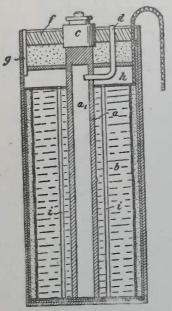
sistance of only 10 ohms. At the beginning of test the voltage was 1.60. The test was started February 29, 1908. The cell was never disconnected from its resistance and consequently never had a chance to recuperate. Despite this when a reading was taken on July 6, 1908, the voltage was still 1.18. total capacity of the battery, consequently, was 163 ampere hours, which is a remarkable showing for a dry cell.
