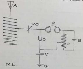
Ans.—The above diagram shows a very sentitive receiving arrangement. While it is not absolutely necessary to use a variable condenser, it is by all means preferable, as by using same, stations not wanted may be tuned out, also the sound in the phones will be greatly increased.
