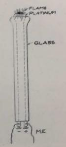
Referring to our illustration two platinum wires pass through a glass handle 6 to 8 inches long. These two wires are made to protrude at the top for about 1/4 inch. As will be seen there is no cutting edge.
