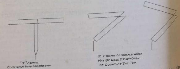
forming the antenna. The original Marconi aerial, namely, a single vertical wire, is very seldom used now, and the idea of the net aerial has also been almost entirely discarded, it having been theoretically determined that the number of wires placed in parallel, as shown in figure 5, are equivalent in capacity to a solid sheet of metal or a net, and the wires offer much less resistance to wind
