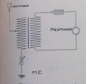
parent. This need has been met in a variety of ways, some mechanical, but usually with some form of tuner employing an air core transformer, technically called a "jigger."
