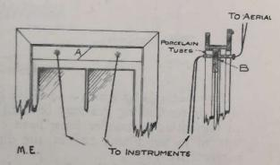
Two holes are drilled to let through two porcelain tubes, each about 18-20 inches long. These tubes should fit quite The aerial wires are then snugly. carried through the tubes. Leakage is practically impossible with this method. The construction has furthermore the great advantage that the boards can be taken off at a moment's notice and be replaced in another window. No unsightly holes remain nor will walls or window be damaged in any respect.
