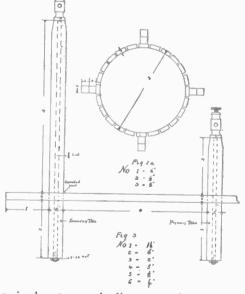
I inch at equal distances from each other, on each end of the coil, so as to form supports for four sticks, I/2xI/2xI7 inches, running lengthwise on the coil, and separated from the secondary wire, on which to wind the primary coil. Now make two grooves 1/8 inch deep and 1/8 inch wide, making this mea-urement a trifle full, and cut same a scant 1/4 inch apart, the edge of the
