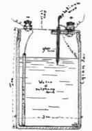
A. 4.—The sketch which we reproduce herewith represents a Wehnelt interrupter. However, you can not use same with less than 24 volts, either direct or alternating current. By pushing the platinum wire more or less into the electrolyte, more or less current will flow through the coil.
