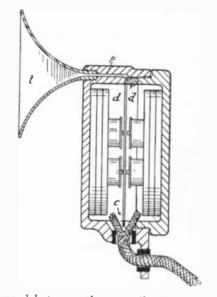
formed between the two diaphrams. At the upper part of the pasteboard ring a small piece is cut out. At this point a small channel p ends, which is in communication with the funnel t.
