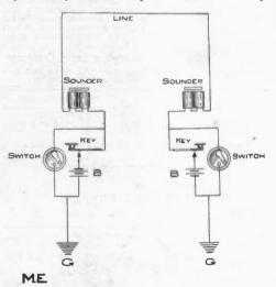
by following diagram, using common two-piece or combination telegraph sets and one extra switch for each station.
