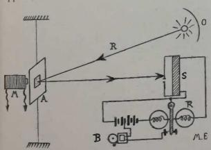
An extremely light piece of sheet iron A, is hung between two platinum wires of the minute diameter of 0.0001 inch. In the centre of the iron sheet a small, very light mirror is cemented. An electromagnet M, which may have a resistance as high as 10,000 ohms, is placed immediately behind the iron foil, so that the magnet core almost touches the iron.
