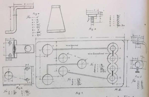
Procure a piece of brass 31/2" long (this allows for wastage), 1/8" thick, 11/8 wide at one end and 1/2" wide at the other, and make up as per Fig. 4.
